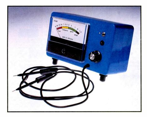
The subject of an electrolytic capacitor's ESR has generated a lot of interest in recent issues. Alan Willcox has taken it a stage further in designing a practical ESR meter. This first part deals with the operation of the circuitry used in the meter
