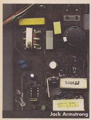
write this during the lightning season: my workshop has been filled with allegedly Tightning damaged' receivers, most of which had simply refused to start up after being unplugged from the mains supply for a while. This is usually a because of low-value electrolytics, nothing to do with lightning damage.
