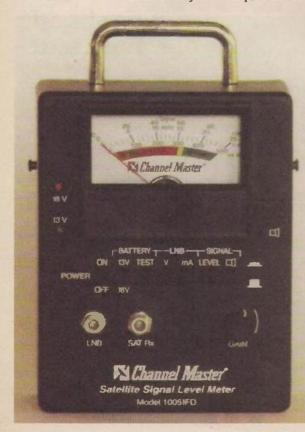
tion with the gain control to obtain accurate assessments of the performance of LNBs.
