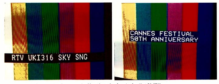
(Left) Analogue colour-bar identification received by John Locker from Intelsat K at 21.5°W. (Right) Digital colour-bar identification received by John Locker from Intelsat K. Note the sharper bar transitions.
