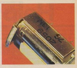
Fig. 4: A worn head. The step or groove is visible near the top edge of the audio head insert.
