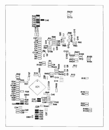
Fig. 2: Some of the surface-mounted component layout around IC1.
