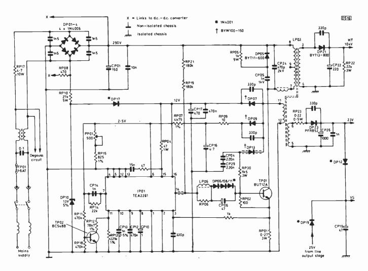
Fig. 2: The power supply circuit. Some component values/voltages depend on the type of tube fitted. We have shown the values for the 14in. model, since this is the one mainly sold in the UK.
