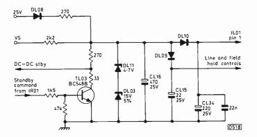
Fig. 4: The standby/on switching circuit that controls the supply to pin 1 of the TDA8218 timebase chip IL01.
