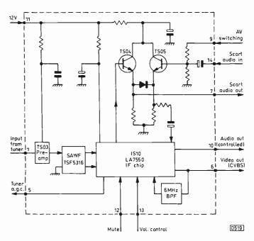
Fig. 5: Block diagram of the i.f. module used in UK models, including the scart audio input/output switching circuit.
