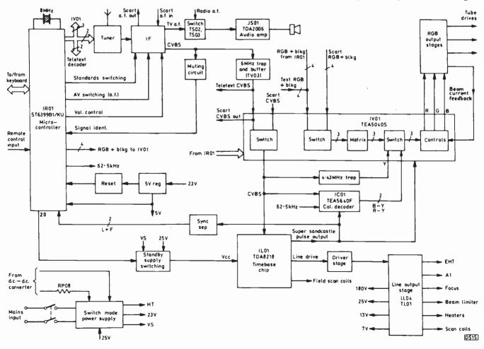
Fig. 1: Simplified block diagram of the TX90E chassis.
