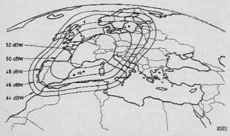
Fig. 3: Eutelsat II F1 superbeam footprints.
