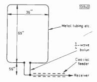
Fig. 1: Brian Williams' squashed-quad aerial, covering chs. E2/3, is suitable for loft mounting. Connection is shown via a quarterwave balun.
