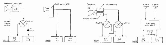
Fig. 6 (left): Simplest way of using the output from a single LNB to feed two satellite TV receivers. An extra lead, shown with broken line, is required where the polariser is current driven.
