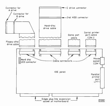
Fig. 8: Typical IDE board layout.
