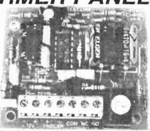
Z5514 Universal bell timer. Panel 63x55mm uses a 556 + 3 transisitors to provide both 10 minute delay and 20 min cut off timers, with ability to disable one or other. +ve or -ve trigger. SPCO relay. 12V operation, Supplied with adhesive stand offs and connexion data. REDUCED TO £4.95
