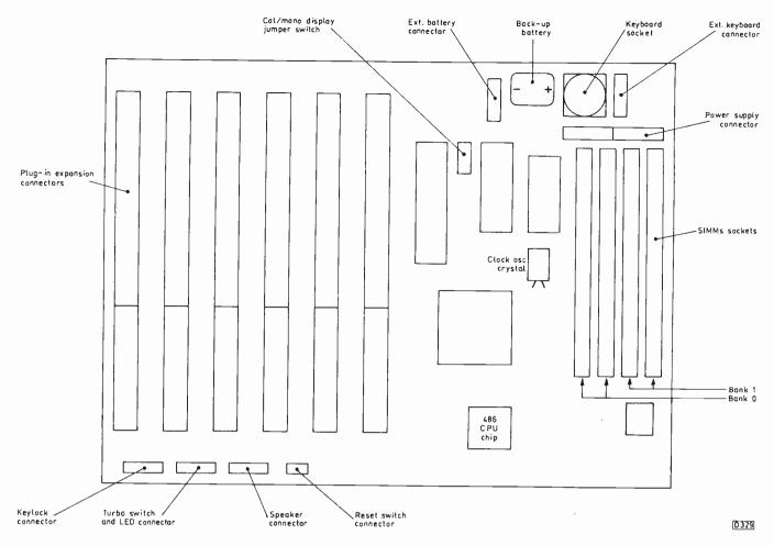
Fig. 1: Typical motherboard layout.
