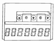
Z2658 LED module. An interesting little PCB 50x35mm that has mounted on it a 7 digit 7 segment red display, and a plastic moulding under which are 3 surface mount LED's, one each red, yellow and green. On the back of the PCB is a SED5031M chip. Offered without info at present, although we are working on it. Believed to have been the display on a mobile phone. Only £1 each
