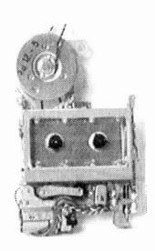
Z5716 Extremely high quality compact mini only size Overall cassette deck. 89x57x16.5mm, 3V operation. Motor has tacho 4 Combined sensor. record/playback/erase head. Another motor with worm drive just 14x11mm dia used to engage the pinch roller with the capstan. Brass flywheel, diecast frame. No electronics, but flying leads from motor, head and switch Superb value at £4.95
