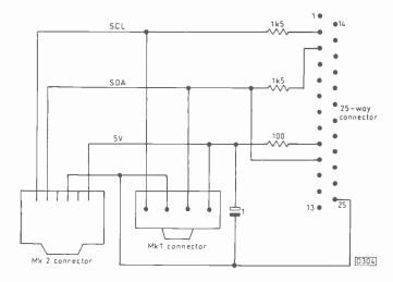
Fig. 3: Connections to an LPT1 computer port.
