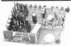
**Z5783** Ringer Generator Panel. The best thing about this PCB is the power transistors - TIP35C & TIP36C (25A 90W 100V - over £5 a pair!) on heatsinks. Also on the main board 220x195mm are 4 x 100uF 63V caps, 'continental' relay, LM358, LM339, around 20 plastic transistors, R's, C's etc + a DIN41612 connector and 9 x 10way DIL header plugs. A sub panel 132x35mm contains 8x74HC chips + an SGS 28640(?) 68 pin PLCC chip. £4.95
