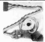
**Z5046 Motor Panel**, PCB with mercury tilt switch, 2 x VTL10D2 opto slotted switches, length of 11 core cable with socket and superb 12V. 48 step, 7.5° Airpax stepper motor 35mm dia  $\times$  21mm with a 16 tooth 9.5mm gear wheel mounted on the 2mm dia spindle. Fixing centres 42mm £3.50
