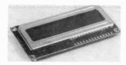
Z5096 16 character × 1 line. Very similar to our Z1814 but slightly larger character -6.3x3.15 (8 × 5 dots). Type LCDM16166 by Refac. Supplied with data. Uses Hitachi HD44780AOO chip.
