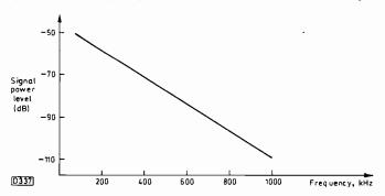
Fig. 1: Frequency response of a voice-grade cable (approximate).
