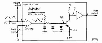
Fig. 8: Generation of the variable duty-cycle pulse waveform required to control the thyristor field output circuit.
