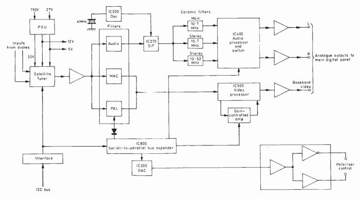
Fig. 2: Simplified block diagram of the satellite receiver.
