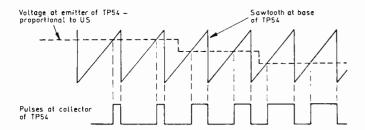
Fig. 2: Action of the pulse-width modulator transistor TP54.
