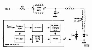
Fig. 7: Outline of a thyristor-controlled, pump-mode field timebase.
