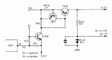
Fig. 3: The power-on switching circuit.
