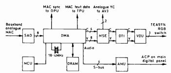
Fig. 3: Block diagram of the D2MAC part of the features board.
