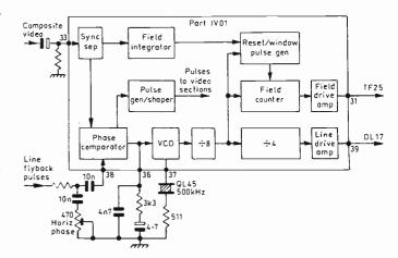
Fig. 4: Block diagram of the timebase generator sections of IV01.
