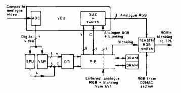
Fig. 4: Block diagram of the PIP part of the features board.
