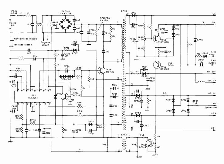
Fig. 1: Power supply circuit, Ferguson ICC7 chassis. Some component values depend on tube type.
