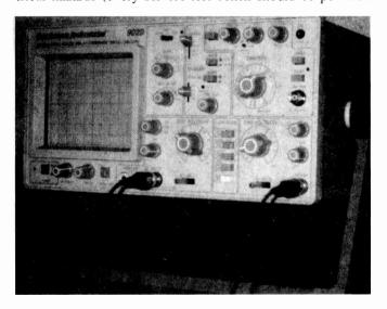
The Wavetek 9020 dual-trace, 20MHz oscilloscope.
