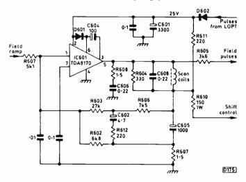
Fig. 6: Field output circuit used in a current-production, large-screen TV chassis.
