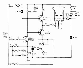
Fig. 7: Part of the tube base panel circuitry, including the red output stage.
