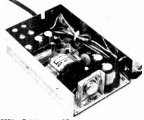
AA12531 Switch mode PSU by Astec partially cased, 160x104x45mm overall with 160x100mm Eurocard PCB, Inputs and outputs are on colour coded flying leads, Input 115/230V 50/60Hz, Outputs: +5V @ 5A; +12V @ 0.15A, Total wattage 50W.
