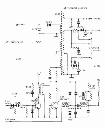
Fig. 5: Line driver and output stage circuitry. Some circuit details vary with tube type.
