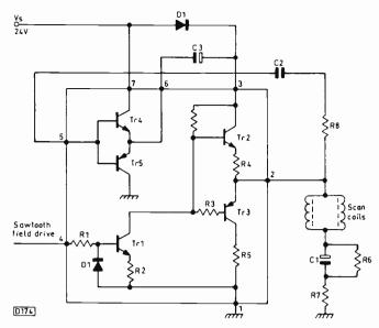
Fig. 5: Principle of the flyback-boosted field output stage: the chip's internal circuitry has been simplified to illustrate the basic operation.
