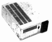
BM41012 Superb switch mode PSU made by Astec. Enclosed case 175x136x65mm with switched and fused IEC mains inlet. 160x80mm PCB with output plns extended to external connector. Input 115/230V 50/60Hz. Outputs: +5V @ 3.75A: +12V @ 1.5A: -12V @ 0.4A. Total wattage 65W £14,95; 25+11,70: 100+9,75
