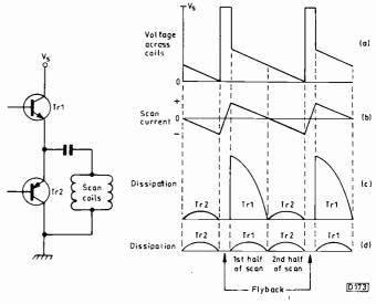
Fig. 4: Reason for using a flyback generator. (a) Voltage waveform developed across the scan coils. (b) Scan current waveform. (c) How the upper transistor (Tr1) would have to absorb the difference between the applied and the required energy during the first half of the scan without a flyback generator. (d) The low, equally-shared output transistor dissipation when a flyback generator is used.
