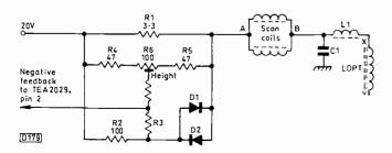
Fig. 10: The feedback arrangement for s-correction and height control with the type of circuit outlined in Fig. 8. Both rely on the voltage developed across R1.
