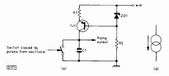
Fig. 2: Simple constant-current generator circuit (a), constant-current generator symbol (b).
