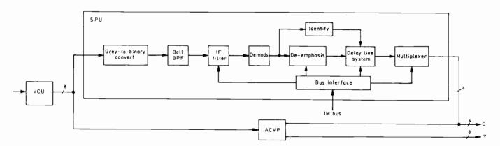
Fig. 1: Block diagram of the Secam processor unit.
