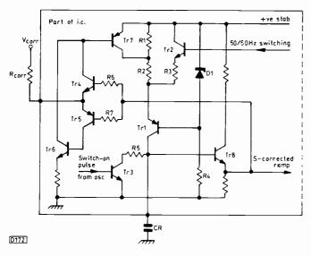
Fig. 3: Principle of in-chip s-correction: the circuitry actually used is much more complex than this.
