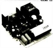
**Z660** Astec switch mode PSU type AA7271. This small PCB, just 50x50mm will accept 8-24V input and give a stable 5V dc at up to 2A output. The 6 transistor circuit provides current overload protection, thermal cut-out and excellent filtering. Offered at a remarkably low price. Price £5.00
