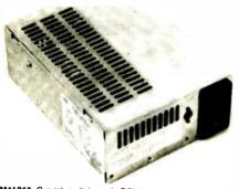
BM41012 Superb switch mode PSU made by Astec. Enclosed case 175x136x65mm with switched and fused IEC mains inlet. 160x80mm PC8 with output pins extended to external connector. Input 115/230V 50/60Hz. Outputs: +5V @ 3.75A; +12V @ 1.5A; -12V @ 0.4A. Total waitage 65W £14.95; 25+11.70; 100+9.75
