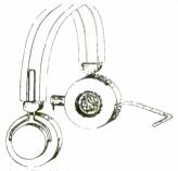
H8 Excellent quality Adastra stereo headphones with boom microphone. Freq. response 20-20,000Hz, 32R impedance. Microphone 600R . 2m leads fitted with 3.5mm plug for mic, and 3.5 mm plug +adaptor for headphones. Padded earpleces and leatherette headband. ONLY £9.95
