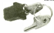
Z2168 Superb quality British made (TOK). Gold plated DPCO contacts. Key can be removed in either position. PC mounting or clip fix - needs 15x15mm cut-out. Ideal for alarms etc.
