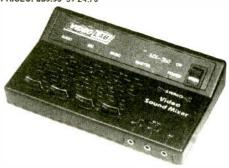
MX350 3-channel portable stereo video sound mixer. Inputs from camera audio, stereo microphone and music source. Output to video recorder controlled by master Earphone monitor socket. Powered by internal battery or external power supply. Supplied complete with 4 connecting leads and a 6.35mm stereo adaptor
