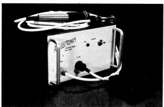
The AK Electronics RA100 desoldering station.
