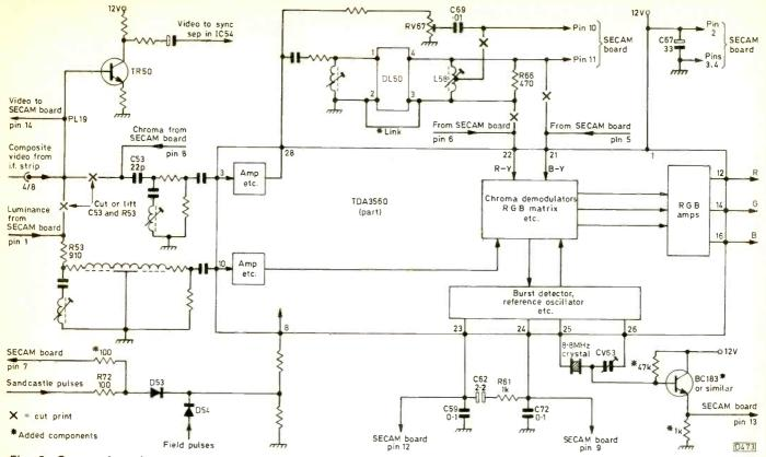
Fig. 2: Connections between the Sendz SECAM board and the TDA3560 PAL decoder circuitry in the Ferguson TX9 chassis.
