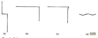
Fig. 3: Silicon pnp transistor waveforms: (a) base-emitter, (b) base-collector, (c) emitter-collector. The centre pin-base waveform with an STR450 is shown at (c).
