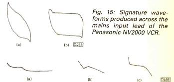
Fig. 16: Signature waveforms produced between various pins of a TDA4503 i.c.: (a) between pins 20 and 21, (b) between pins 22 and 23, (c) between pins 25 and 26.
