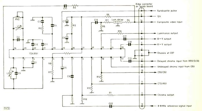
Fig. 1: Approximate circuit of the Sendz SECAM board.
