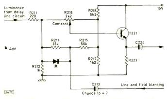
Fig. 1: Blanking modification for the Philips G8 chassis to cure teletext-line interference. The components shown are on the decoder panel
