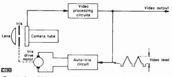
Fig. 1: Auto-iris system. The auto-iris circuit drives the iris so that it opens or closes to maintain a constant average video level.
