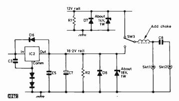
Fig. 1: Modifications to D.J. Stephenson's satellite TV servicing aid. See letter from G.R. Darby. The diodes in series with IC2's earthy lead are in the 1N400X series.
