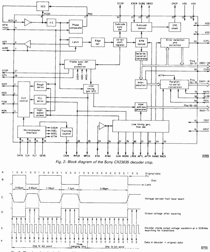
Fig. 3: The decoder checks for transitions in the off-disc signal then generates the appropriate ones and zeros.
