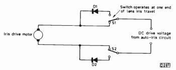
Fig. 2: The microswitch arrangement.
