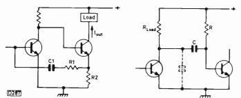
Fig. 5 (left): Two-stage current amplifier using frequencydiscriminating negative feedback for l.f. boost.
