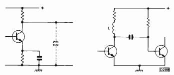
Fig. 7 (left): Use of negative feedback to compensate for h.f. loss caused by shunt capacitance.
