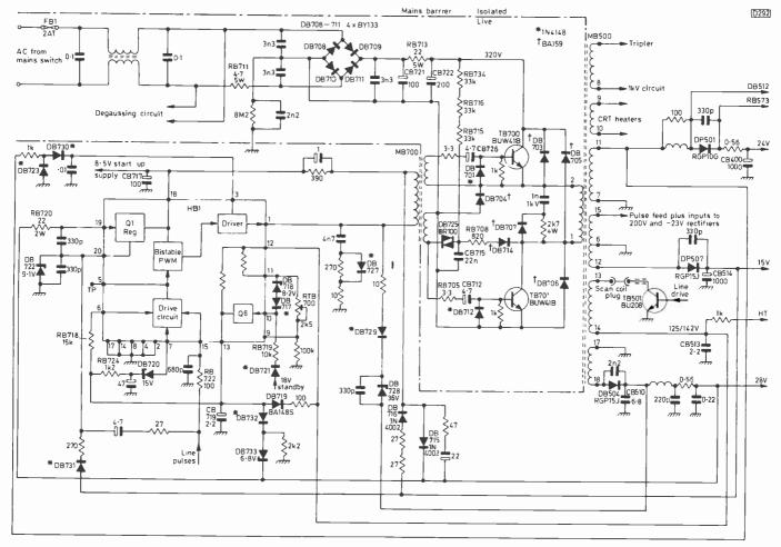
Fig. 1: The Ipsalo-2 circuit as used in the H chassis.
