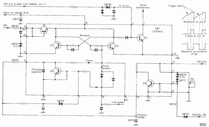
Fig. 2: Circuitry in and around the LF0034A hybrid chip HB1.
