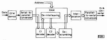
Fig. 4: How the signal is handled during the error correction processes: the RAM makes it available to the various decoders and carries out de-interleaving.
