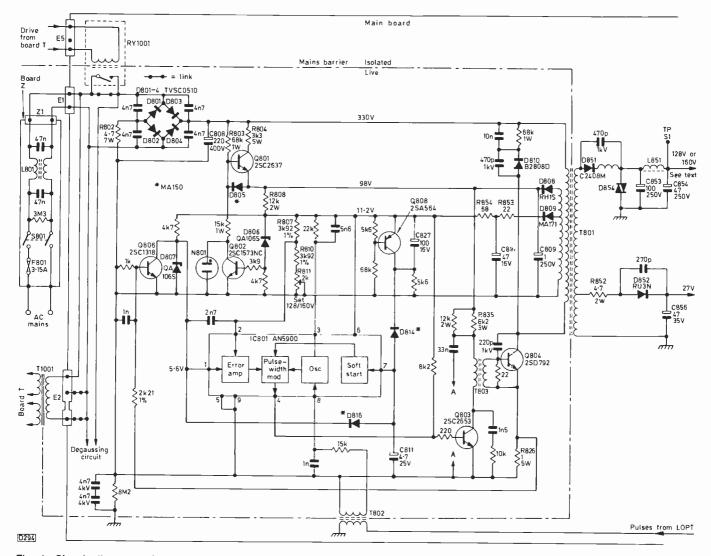
Fig. 1: Circuit diagram of the chopper power supply used in the Panasonic U3 and U3W chassis. The e.h.t., 195V, 26V and 18V supplies are derived from the line output transformer. The 18V supply feeds the 12V regulator.
