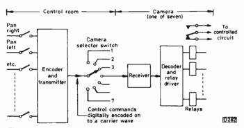
Fig. 3: Outline of the telemetry control system.
