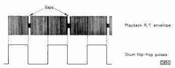
Fig. 1: Top, the waveform at the faulty machine's playback head amplifier. Bottom, the correctly timed 25Hz drum flipflop waveform.
