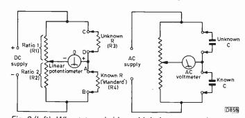
Fig. 3 (left): Wheatstone bridge with balance potentiometer.
