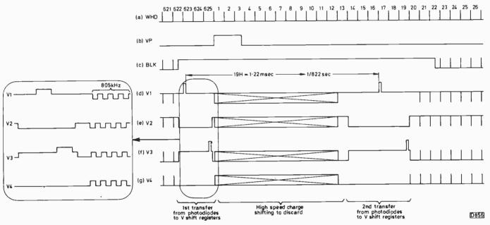
Fig. 5: Time-related waveforms for the high-speed shutter mode, (a) line sync pulses, (b) field sync pulse, (c) composite blanking, (d-g) three-level vertical drive pulses in the image sensor section – the highest levels V1 and V3 trigger photodiode charge transfer. The 805kHz pulse trains in the waveforms on the left rapidly empty the vertical shift registers during the first half of the field blanking period.
