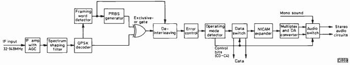
Fig. 6: Decoding the NICAM 728 stereo signal.
