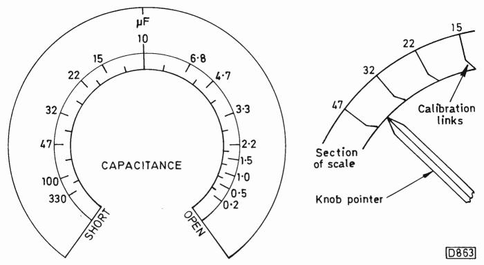
Fig. 9 (left): Full size calibrated scale for the bridge.
