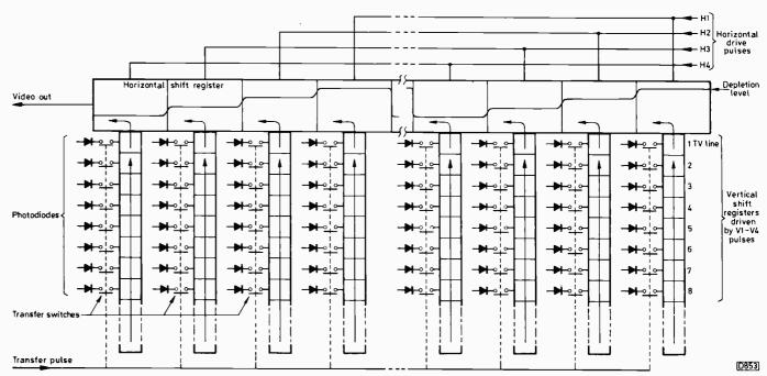
Fig. 2: Representation of a complete CCD image sensor, simplified to show 64 sensors in an eight-by-eight matrix. Typical practical arrays for consumer cameras would have about 250,000 elements arranged in a  $579 \times 422$  matrix. The switched charges progress upwards along the vertical shift registers then along the horizontal shift register, under the control of four-phase clock pulses.
