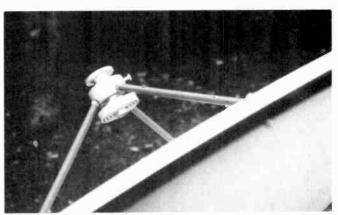
Photo 7: Another view of the scalar ring assembly – its adjustment screw can just be seen. This enables the ring assembly to be slid up and down the feed tube. Careful observation of a weak signal on a TV screen while adjusting the ring will show clearly where it peaks.
