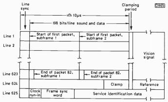
Fig. 2: Frame multiplex structure used for C-MAC and D-MAC Packet systems (not to scale).
