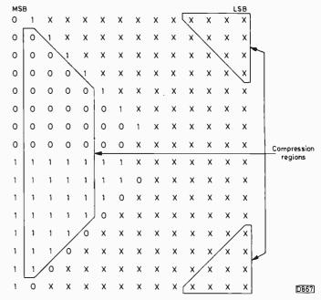
Fig. 4: Coding scheme for NICAM 728 companding.
