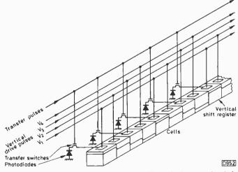
Fig. 1: Photodiode charge transfer. The diodes on the left represent one column of image sensors: the "progressive bucket" effect of the transfer charge voltage applied to each cell of the register on the right is represented by the depth lines on their sides.
