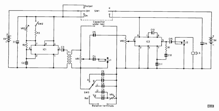
Fig. 6: Circuit of the wide-range capacitance bridge.
