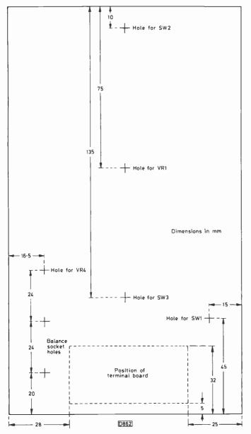
Fig. 8: Suggested drilling details for the case top. Hole sizes depend on the components used.
