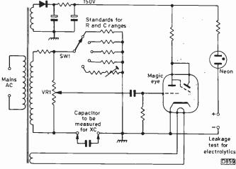
Fig. 5: Basic circuit arrangement used in the Hunt's Capacitance Analyser.
