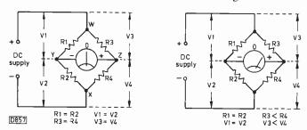
Fig. 1 (left): Wheatstone bridge in the balanced condition.
