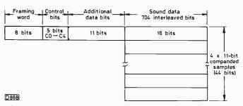
Fig. 5: NICAM 728 frame multiplex.
