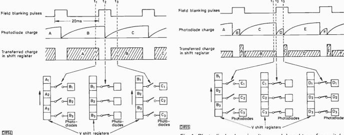
Fig. 3: Photodiode charging and transfer switching at the normal (20msec) shutter speed. Three successive fields, identified as A, B and C, are shown.
