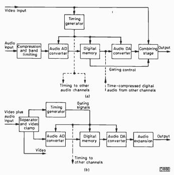
Fig. 3: The VIMCA system. (a) Block diagram of the encoding arrangement. (b) Decoder block diagram.
