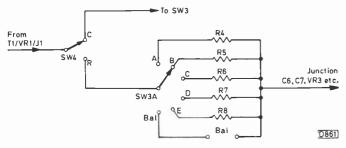
Fig. 7: Extra components required to add resistance ranges. SW3/SW3a comprise a two-pole, six-way switch.
