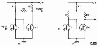
Fig. 4: Feedback arrangements as in Fig. 3 but this time with field effect transistors.
