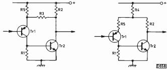
Fig. 5 (left): The arrangement shown in Fig. 4(a), but this time with complementary transistors.
