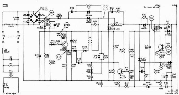
Fig. 1: Thyristor power supply circuit used in the initial version of the Ferguson TX9 chassis (main panel PC1001).
