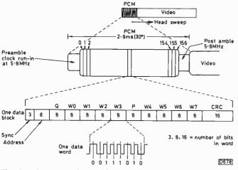
Fig. 37: Analysis of the PCM segment of a recorded tape track. The characteristics are explained in the text.
