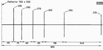
Fig. 4: Element dimensions and spacing.
