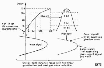
Fig. 35: The effect of non-linear quantisation on the playback signal: quantising noise is present only with large (loud) signals.
