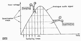
Fig. 31: Principle of digitising an analogue signal.
