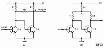
Fig. 3: Two ways of applying negative feedback to a twostage amplifier, (a) by means of a pi network and (b) by means of a T network.
