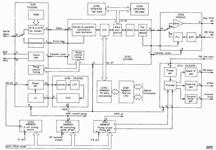
Fig. 36: PCM processing is carried out by several i.c.s, as shown here with their relationships and interconnections. IC111/152/153 are mainly concerned with multi-PCM operation: IC151 additionally deals with PCM dub processing.
