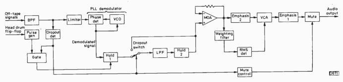
Fig. 30; Block diagram of the audio f.m. playback electronics.
