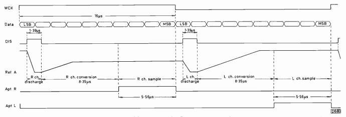
Fig. 39: D-A conversion during PCM replay. In this example the R-channel output is much lower than the L-channel output.
