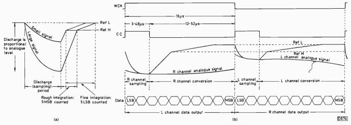
Fig. 33: A-D conversion: (a) working principle; (b) timing diagram.
