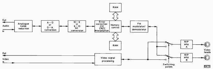
Fig. 32: Block diagram of the PCM processing arrangement.
