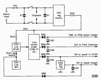
Fig. 2: Block diagram showing the origin of the various supply lines in the TX9 chassis.
