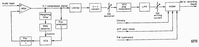
Fig. 29: Block diagram of the audio f.m. recording system.
