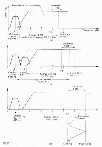
Fig. 1: Comparison between the signal spectra for various VCR systems. (a) Existing VHS. (b) Beta super hi-band. (c) The New Super-VHS specification.
