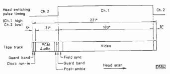
Fig. 7: Composition of a single recorded track on the tape.
