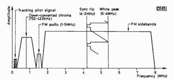
Fig. 8: Video 8 system signal frequency spectrum.
