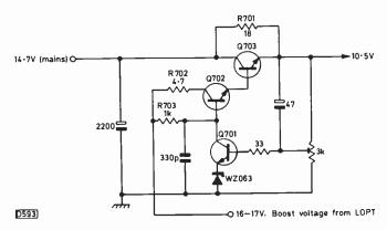
Fig. 1: Regulator circuit used in the Sanyo Model 12-T280.
