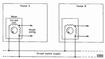
Fig. 1: Electricity supply arrangement.
