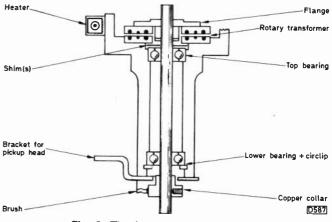
Fig. 2: The lower drum assembly.
