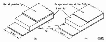
Fig. 1: Structure of the two types of metal tape used with the 8mm video system: (a) metal powder – MP; (b) evaporated metal – ME.
