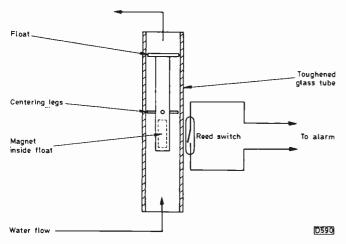
Fig. 3: Water flow alarm system.
