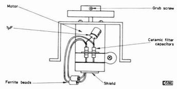
Fig. 1: The drum motor.
