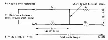
Fig. 4: Using cable resistance measurements to establish the approximate position of a short-circuit.
