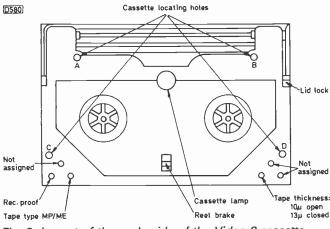
Fig. 3: Layout of the underside of the Video 8 cassette.
