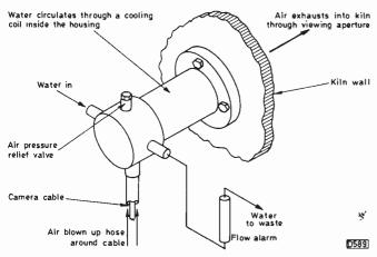
Fig. 2: Kiln camera equipment layout.
