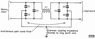
Fig. 3: Effect of using a long earth wire.
