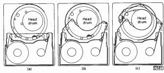
Fig. 4: Video 8 deck layout, showing from (a)-(c) the three-stage tape loading process.
