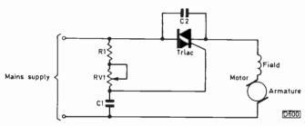
Fig. 5: A.C. motor controlled by a triac.
