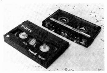
Fig. 2: Video 8 and compact audio cassettes compared. The sizes and weights are similar. In the audio-only mode the Video 8 tape can accommodate up to 18 hours of very high quality audio sound – the audio cassette has a 90 minutes maximum capability for ordinary stereo reproduction.
