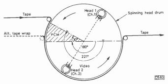
Fig. 6: Tape wrap and head scanning. The usual 180° of head scan is used for video recording: a "pre-scan" section is available to accommodate PCM audio signal recording.
