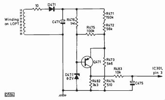
Fig. 2: Over-voltage protection circuit used in Samsung and Toshiba colour portables.
