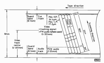
Fig. 5: Track layout on Video 8 tape.
