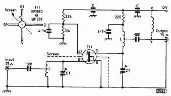
Fig. 1: MOSFET Band III preamplifier circuit designed by Philippe Bouchard. The trimmers are 2-10pF subminiature types. All resistors \(^1\s\text{W}\) metal oxide. Coils L consist of four turns of 22-26g wire, \(^1\s\) in. diameter, tapped 1\(^1\) turns from the "dead" end. The v.h.f. choke (if required for powering) consists of 12 turns of 30g enamelled copper wire, close-spaced \(^1\) in. diameter, self-supporting.
