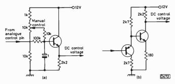
Fig. 6: Analogue control interfacing circuits.
