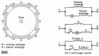
Fig. 1 (left): Pole arrangement for a split-phase motor. Fig. 2 (right): Methods of phase shifting.
