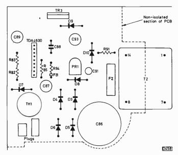
Fig. 3: Positions of the main components, and those referred to in the text, in the power supply. TH1 is the degaussing circuit thermistor.
