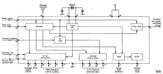
Fig. 4: Block diagram of the SAA5012 decoder chip.
