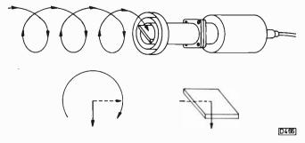
Fig. 3: Depolarising a circularly-polarised signal – the C band method for Gorizont. A PTFE wedge at 45° bends the horizontal component of the signal through 90°, adding it to the vertical component to increase the gain by 3dB.
