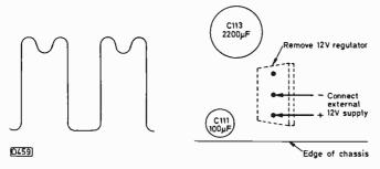
Fig. 4 (left): Waveform at the base of the chopper transistor TR3 with F2 removed from its holder.
