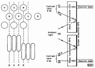
Fig. 42 (left): To achieve a comparable number of vertical picture lines the dot pitch of an in-line gun tube must be much finer than with a delta-gun tube.
