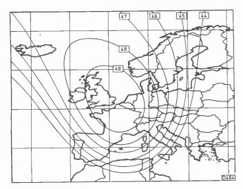
Fig. 1: Footprint for Eutelstat-1 - dBW contours.
