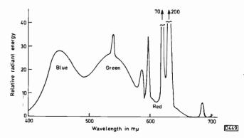
Fig. 40: Spectral emission and relative efficiencies of the phosphors. Although red peaks far higher than the others its very narrow emission band makes it the least efficient of the three.
