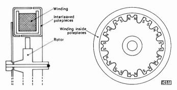
Fig. 3 The synchronous motor.
