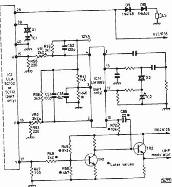
Fig. 11: Circuit variations around IC1/IC14 in earlier versions compare with Figs. 1 and 5.
