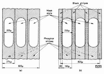
Fig. 41: Positive-tolerance screen-mask system (a) compared with a negative-tolerance system (b) for use with a black matrixed screen.
