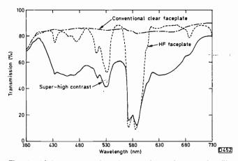
Fig. 44: Light transmission characteristic of a selective filter faceplate.
