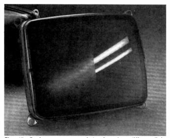
Fig. 45: Surface treatment of the faceplate diffuses light reflections from the tube's faceplate.
