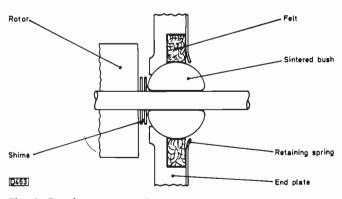
Fig. 6: Bearing construction.
