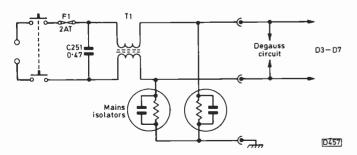
Fig. 2: Alternative mains filter arrangement.
