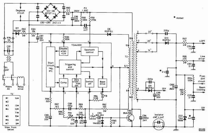
Fig. 1: Power supply circuitry used in the Fidelity ZX3000 chassis
