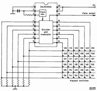
Fig. 1: Transmitter keyboard and encoder.
