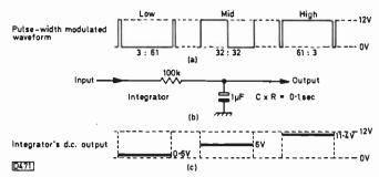
Fig. 5: Conversion of a pulse-width modulated "analogue" output from the SAA5012 to a d.c. control voltage.
