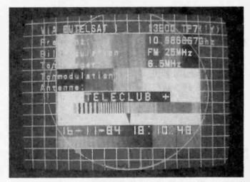
Photo 4: Same signal as shown in Fig. 3 but this time received with the addition of an LNA.
