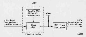
Fig. 1: Block diagram of the downconverter/u.h.f. i.f. amplifier system. The oscillator can be tuned over approximately 10-4-11-4GHz.
