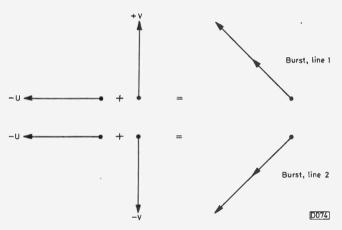
Fig. 5: Forming the burst signal.
