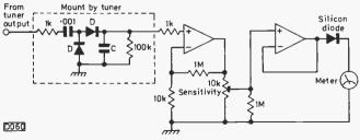
Fig. 5: Signal strength meter circuit. Diodes D type OA90 or similar. C is  $0.001\mu\text{F}$  – if the readings vary a lot with the video content, increase the value of C to  $0.1\mu\text{F}$  or more. The  $10k\Omega$  potentiometer adjusts the meter's sensitivity. Any type of operational amplifier will do.
