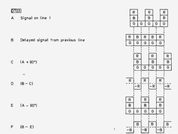
Fig. 4: How the phase colour separation system works.
