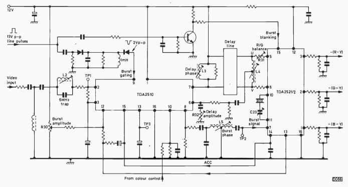
Fig. 3: The two-chip decoder used in Network Models NWC1401 and NWC1402 (simplified circuit).
