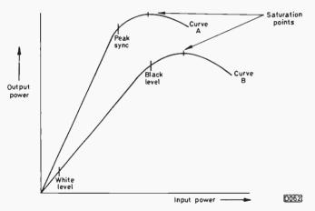
Fig. 2: Klystron power characteristic curves. Efficiency can be increased by pulsing the klystron so that its characteristic is altered for different parts of the input signal waveform.
