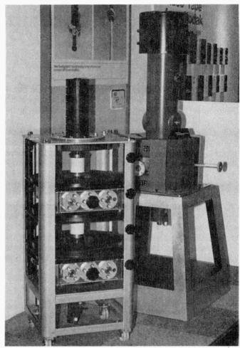
High-power devices for u.h.f. TV transmitters: a four-cavity klystron on the left and a klystrode on the right. Klystrons are tuned by adjusting the cavities: two of the four cavities of the device on the left are shown in position. The klystrode is a new, experimental type of amplifying device that combines some of the features of a tetrode and a klystron output amplifier.
