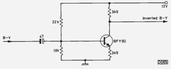
Fig. 2: Simple signal inverter circuit.
