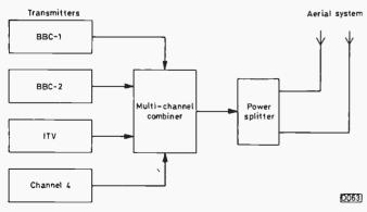
Fig. 3: Combining the outputs from four transmitters to drive the aerial system.
