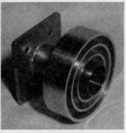
Photo 5 (left): Scalar feedhorn, showing front rings.
