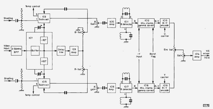
Fig. 6: Block diagram of the colour signal processing system used in the Ferguson 3V17 camera.
