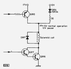
Fig. 1: Pinch roller solenoid circuit, Sanyo VTC9300.
