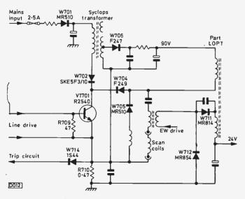
Fig. 1: The main elements of the Syclops circuit used in the Thorn 9000 chassis.
