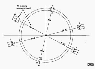
Fig. 5: Type of display obtained with a misaligned or faulty decoder.
