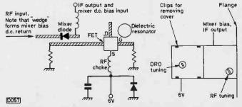
Fig. 2: Left, approximate circuit of the Mitsubishi FO-UP-11K oscillator/mixer module. Right, pin connections.
