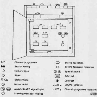
Fig. 1: Philips' on-set controls with the TRD IV remote control system – and what the symbols mean.
