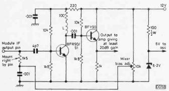
Fig. 3: U.H.F. i.f. preamplifier and mixer bias circuits. Take the output to a further wideband u.h.f. amplifier with a gain of at least 20dB. An additional amplifier prior to the receiver may help as well. Coil L consists of two turns 1/8in. diameter wound on a resistor.
