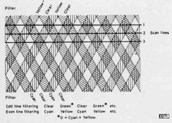
Fig. 2: Phase colour filter arrangement.
