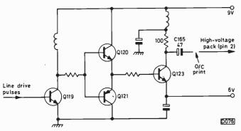
Fig. 2: High-voltage pack drive circuit, Panasonic video camera type WV3000.
