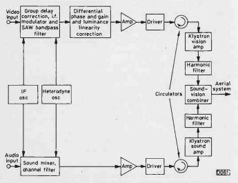
Fig. 1: Block diagram of a high-power u.h.f. TV transmitter using i.f. modulation and klystron output stages. The sound and vision channels are both shown: the outputs from the two klystrons are combined.
