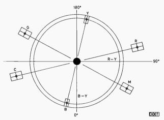
Fig. 4: Scope vector display obtained with a correctly adjusted decoder. The display arises from the fact that the scope's X and Y axes coincide with the B-Y and R-Y axes respectively: with a colour bar signal of the type used dots are obtained at the phase positions corresponding with the colours in the pattern.
