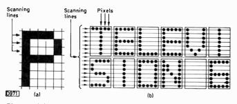
Fig. 13: (a)  $7 \times 5$  dot matrix used for data displays. (b) Dots, cells and their relationship to the TV raster.
