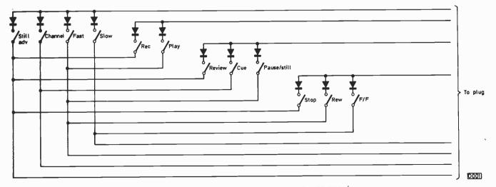
Fig. 3: Multicore cable remote control switch circuit used with the Panasonic NV7000.
