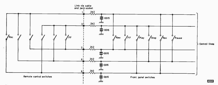
Fig. 4: Remote/on-board switching circuit, Mitsubishi Model HS304.
