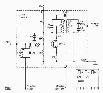
Fig. 1: Circuit of the U500 sound selectivity module.
