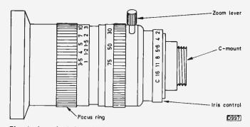
Fig. 4: A typical detachable zoom lens. The first control from the end is the focus ring, which is calibrated in feet and metres. More adjustment is needed at the near end of the scale than the distant one, as the wider spacing of the calibration shows. Next is the zoom control, which is sometimes calibrated with focal length. Finally there's the iris control, which is marked with the f numbers. The C position denotes closed, i.e. no light enters.
