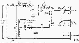
Fig. 1: C.R.T. tester/booster circuit.
