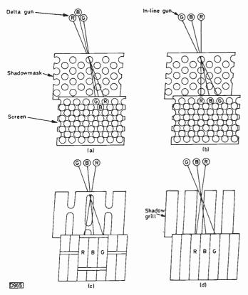
Fig. 7: The four alternative gun/mask/screen shadowmask tube configurations, (a) delta gun, (b) dots with in-line gun, (c) striped screen with slots and in-line gun, (d) Trinitron system.
