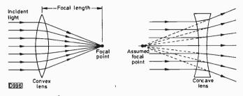
Fig. 2 (left): When parallel rays encounter a convex glass surface they are bent inwards. The angle of refraction is greater for the outside rays than for the inner ones because the angle of incidence is greater, due to the surface curvature. Thus all the rays converge at a certain point (the focal point).
