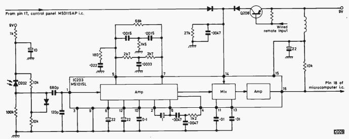
Fig. 7: Infra-red remote control receiver circuit, Ferguson Model 3V35.
