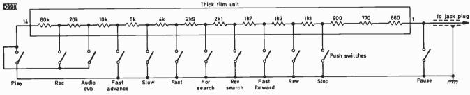
Fig. 1: Circuit of the Hitachi VT8300's remote control handset.
