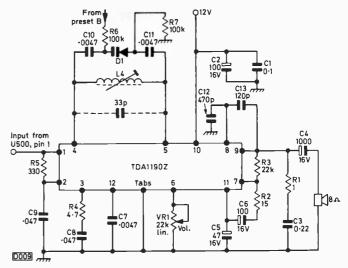
Fig. 3: Demodulator and a.f. circuit.
