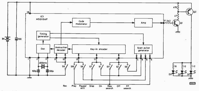
Fig. 5: Infra-red remote control transmitter circuit, Ferguson Models 3V35/3V36.
