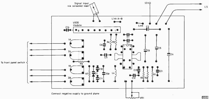
Fig. 4: Component layout. The components are mounted on the groundplane side of the board. Board actual size. **TELEVISION NOVEMBER 1984**
