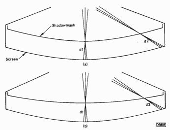
Fig. 10: (a) Constant mask/screen spacing used with earlier delta-gun tubes. Distance d2 is greater than d1, and the phosphor dots are more widely spaced at the extremes of the display. (b) When the mask and screen have different radii distances d1 and d2 remain the same and the dot pitch is uniform over the entire screen area.
