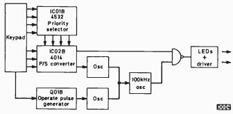
Fig. 6: Block diagram of the infra-red remote control transmitter used with the Hitachi VT8500.
