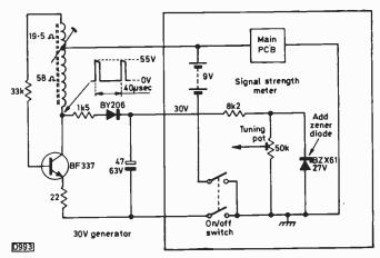
Fig. 1: Oscillator circuit used to obtain a 30V tuning voltage supply from a 9V battery.
