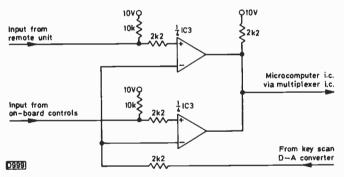
Fig. 2: Arrangement used in the Ferguson 3V29 to combine the remote and on-board control commands.
