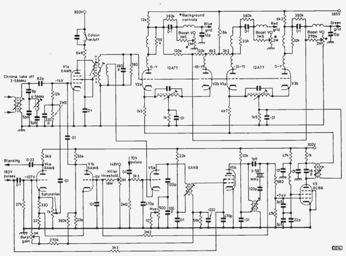
Fig. 1: The colour decoder circuit used in late-production 1957 RCA Super and Special models. The burst/reference signal section was simplified by the use of a passive subcarrier regenerator, hence no need for an a.p.c. loop. Demodulation was carried out on the B - Y and G - Y axes, with matrixing to obtain the R - Y colour-difference signal. Only a single chroma amplifier stage was used.
