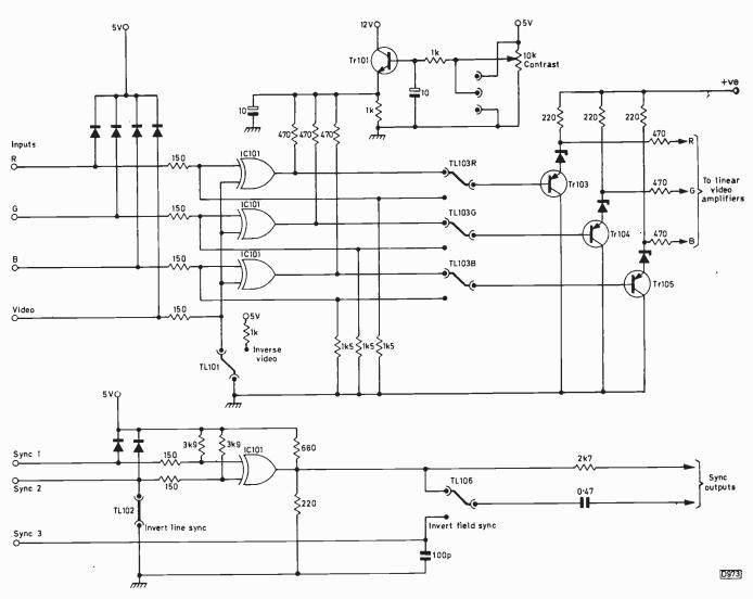
Fig. 15: Representative computer monitor video input circuitry. TTL or linear operation is selected by means of links TL103R/ GIB. The exclusive-OR gates in IC101 invert the video pulses when link TL101 is changed and the line sync pulses when TL102 is present. Transistor Tr101 forms the upper leg of a resistive attenuator for contrast control in the TTL mode. Tr103/4/5 and the accompanying zener diodes provide level-shifting and temperature compensation.
