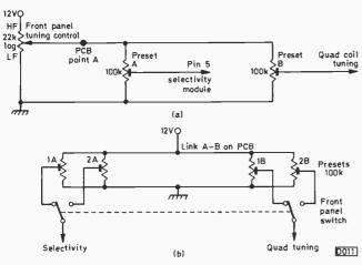
Fig. 5: Alternative tuning arrangements. (a) For continuous tuning, (b) for two-position switched tuning.
