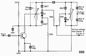
Fig. 2: Selectivity module after modification.
