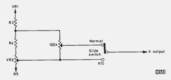
Fig. 2: Modification to the scope component test unit.
