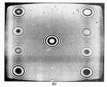
Fig. 6: Off-screen photos of a green zone-plate image. (a) Monitor display. (b) Display after passing through a PAL codec.
