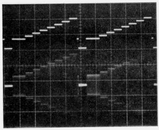
Fig. 3: Alignment traces: upper, video input, 0.5V/cm; lower, r.f. envelope, 200mV/cm.
