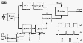
Fig. 17: Digital servo arranged for speed control. The FG pulses operate both counter 1 and the latch.
