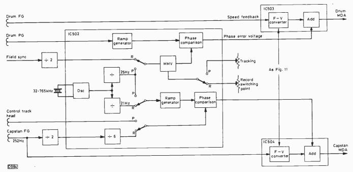
Fig. 12: Addition of the phase and speed control signals. The four-loop system used in the Hitachi VT8000.
