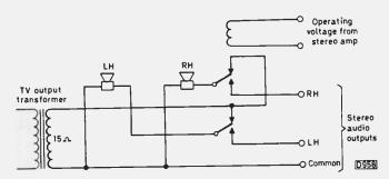
Fig. 1: Relay-operated dual-speaker system for mono/stereo operation.
