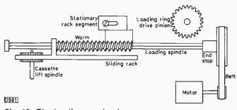
Fig. 10: The loading mechanism.
