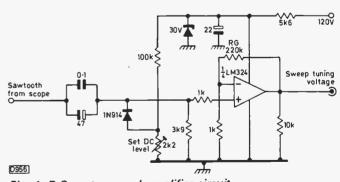
Fig. 4: D.C. restorer and amplifier circuit.
