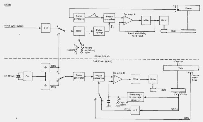
Fig. 10: Block diagram of the servo system used in the Hitachi VT5000 to control two d.c. motors.
