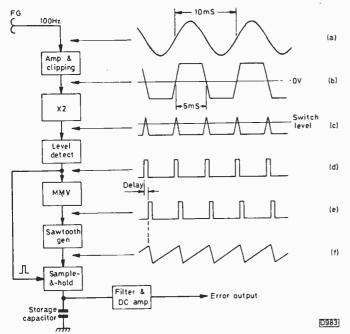
Fig. 11: Speed control system used in the Hitachi VT8000. This employs frequency-to-voltage conversion by means of a ramp and sample system. The duration of the ramp is set by the FG frequency.
