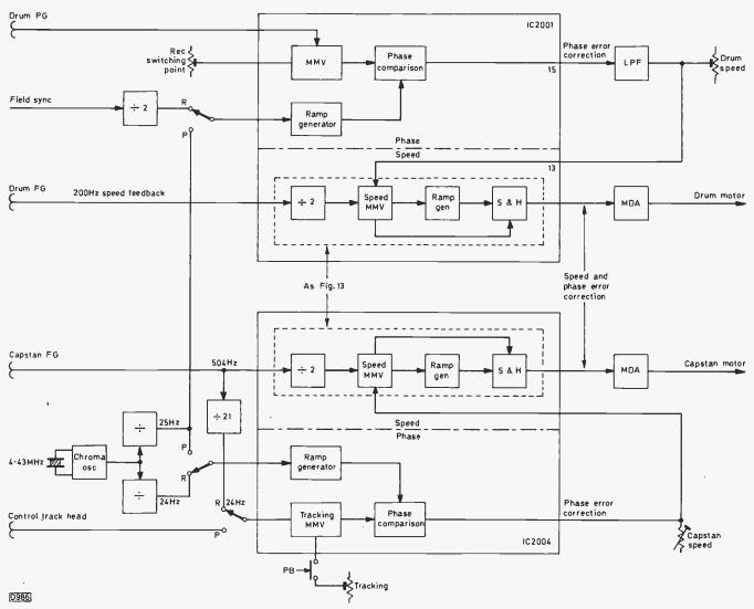
Fig. 14: Phase loops operating on the speed MMVs – Panasonic NV7000. The 4·43MHz chroma reference crystal also provides the servo reference signals.
