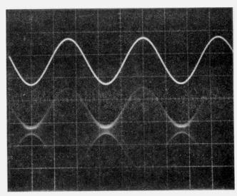
Fig. 4: Alignment traces: upper, sound sinewave input, 0.5V/cm; lower, r.f. envelope, 200mV/cm.
