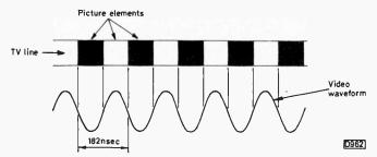
Fig. 3: TV scanning line with maximum detail, with the corresponding video waveform shown below.
