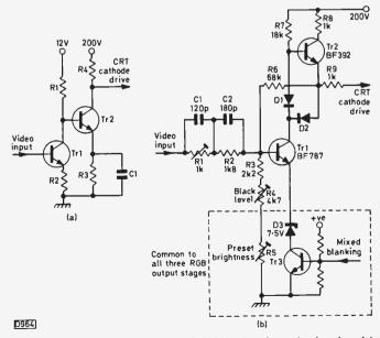
Fig. 5: Video output stages. (a) Simple class A circuit with driver. (b) Class AB circuit as used by Microvitec.
