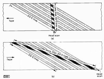
Fig. 19: Video head path with respect to the tracks in (a) cue and (b) review. It can be seen how noise bars arise, also why drum speed correction is required to maintain the correct line scanning rates in these modes.
