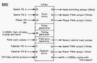
Fig. 18: LSI servo chip used in the Sony F1 and C9. These machines have no drum servo as such: regularly positioned magnets on the drum give six pulses per revolution to PGs A and S. Because the PG S coil is offset by 30° under the drum its pulse lags A by 3msec and the speed loop works to maintain this interval. PG B provides one pulse per drum revolution for phase control.
