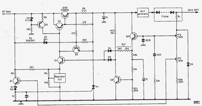
Fig. 2: E.H.T. regulation and protection system used in the Barco CTVM3 series monitor.
