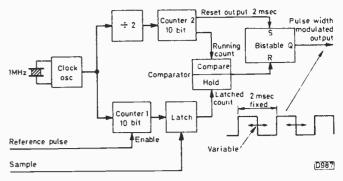
Fig. 15: Simplified outline of a digital servo used to provide phase control.
