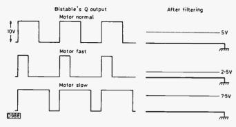
Fig. 16: Low-pass filtering (integration) produces a d.c. error voltage proportional to the mark-space ratio of the squarewave output from the SR bistable.
