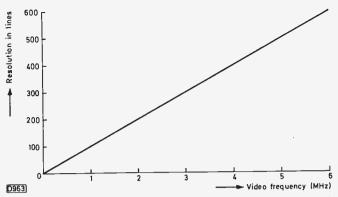
Fig. 4: Video signal frequency plotted against resolution in lines for the standard 625/50 system.
