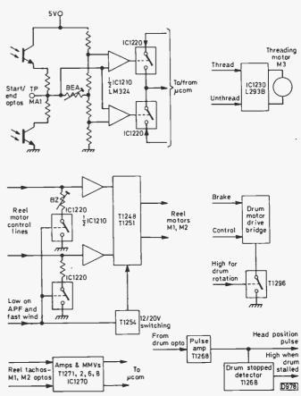
Fig. 7: Motor connection board block diagram.
