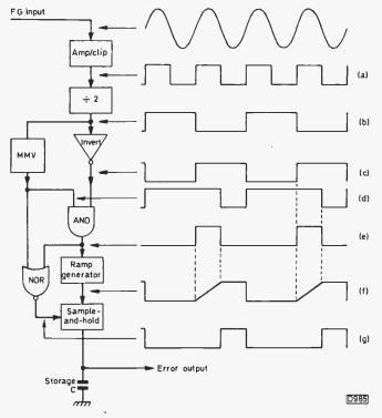
Fig. 13: Frequency-to-voltage conversion technique used in the Panasonic NV7000.
