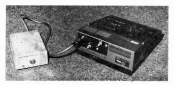
The sync adaptor unit (left) in its diecast box connected to the Sony HV2000 video unit (right).
