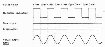
Fig. 4: Effect of the cyan filter in the Saticon tube.
