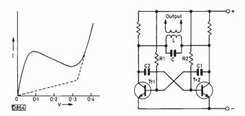
Fig. 15 (left): Forward voltage-current characteristic of a tunnel diode (shown in solid line) and a normal pn junction diode (shown in broken line).
