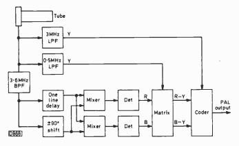
Fig. 3: Block diagram of the electronics required with a Saticon colour camera tube.
