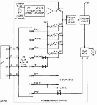
Fig. 126: Reel motor control system used in the 3V24.
