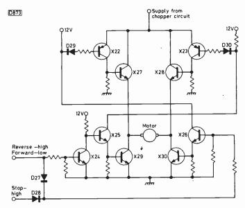
Fig. 128: Reel motor drive amplifier circuit.
