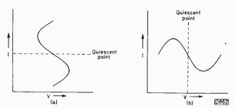
Fig. 12: Examples of current-voltage characteristics with a negative-resistance region. (a) Current controlled, (b) voltage controlled.
