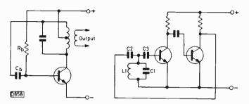
Fig. 7 (left): Hartley oscillator circuit with automatic bias provided by Cb and Rb.
