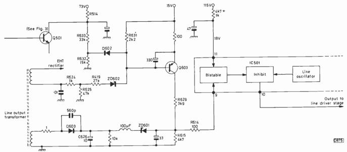
Fig. 2: The shut-down protection circuit.
