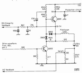
Fig. 3: The field output circuit.
