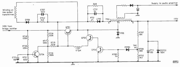
Fig. 1: The switch-mode power supply - simplified circuit.
