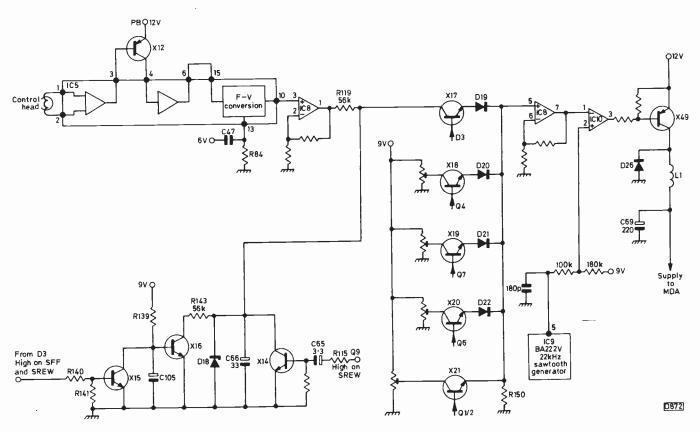
Fig. 127: Circuit details of the reel motor control system.
