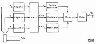
Fig. 1: Block diagram of the electronics required with a trielectrode vidicon tube.
