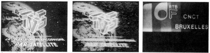
Satellite TV. Left: TV5 signal relayed via satellite and received on a Belgian cable network. Centre: The same signal as received by Nick Harrold in Essex, using an 8ft petal dish. Right: A TV5 test pattern as transmitted from Brussels on ch. E56 – the pattern varies slightly from time to time.
