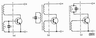
Fig. 4: Oscillator circuits with inductive coupling. (a) Reinartz; (b) Meissner; (c) tuned collector.
