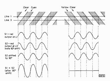
Fig. 5: Colour signal separation with the Saticon tube. The use of a 90° phase shift, a 64 $\mu$ sec delay line and addition gives signal reinforcement or cancellation.
