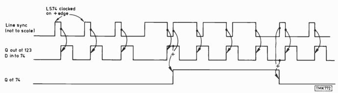
Fig. 4: Field sync pulse generator waveforms.
