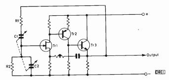
Fig. 11: Wien-bridge oscillator circuit, basic form.
