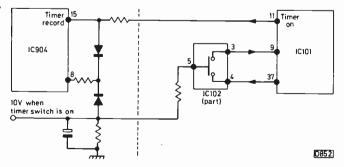
Fig. 4: Arrangement used to control the start of a timer recording, Hitachi Model VT14.
