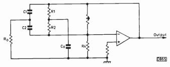
Fig. 17: Oscillator using selective amplification of noise, with the selectivity provided by a parallel-T RC network in a negative feedback path.
