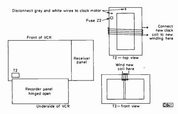
Fig. 1: Transformer details.
