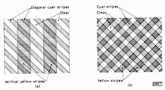
Fig. 2: Filter stripe arrangements used with electronic colour signal separation. (a) RCA Spectraplex tube. (b) Saticon colour tube. Arrangement (a) gives rise to two different colour carrier frequencies. Arrangement (b) introduces a 90° phase shift between the two colour signals.
