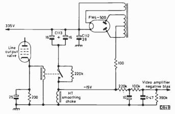
Fig. 1: The full-wave h.t. rectifier circuit used in the Mullard Model MTS389.
