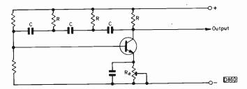
Fig. 10: Simple RC phase-shift oscillator circuit.
