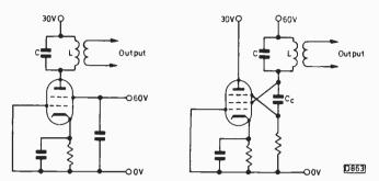
Fig. 13 (left): Dynatron oscillator circuit, basic form. Fig. 14 (right): Transitron oscillator circuit, basic form.
