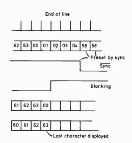
Fig. 3: Column counter and character timings - not to scale.
