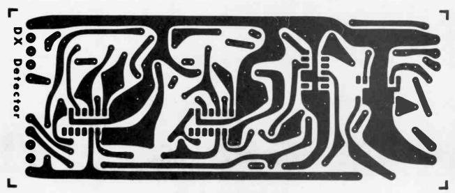
Fig. 6: Track pattern, scale 1:1.
