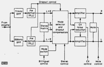
Fig. 4: Block diagram of the sound processing system.
