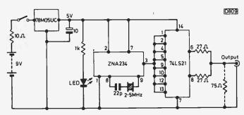
Fig. 1: Black level generator circuit.
