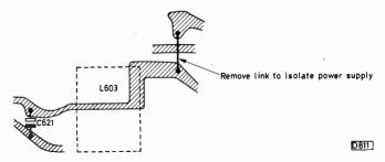
Fig. 2: Location of the power supply isolating link.
