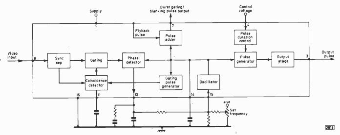
Fig. 3: Block diagram of the sections of the i.c.s used.
