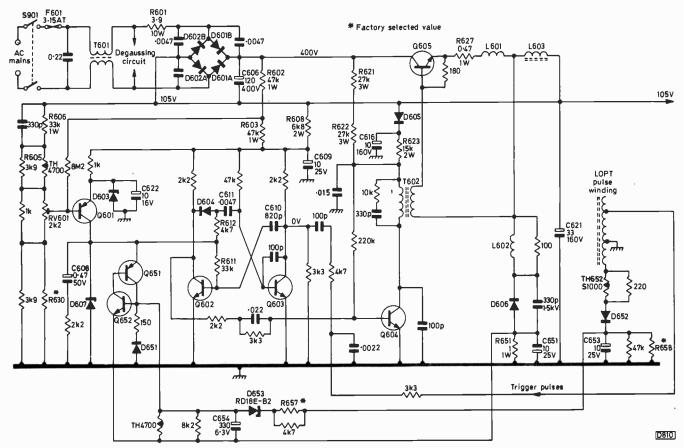
Fig. 1: Circuit diagram of the switch-mode power supply. The multivibrator's main time-constant network comprises R611/C610, the control transistor Q601 adjusting C610's charging time.
