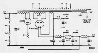
Fig. 1: The Ferguson 841T's power supply circuit.
