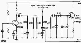
Fig. 2: The resonant circuits and detector used to retrieve the f.m. signal from the disc.
