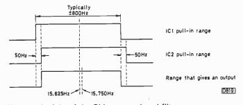
Fig. 4: Principle of the PLL narrow-band filter.
