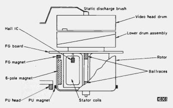
Fig. 121: Basic construction of the drum motor.
