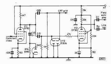
Fig. 2: The video amplifier and sync separator circuits, with d.c. restoration in both feeds.
