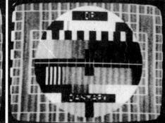
Tropospheric reception from Denmark ch. E8 on December 4th, showing progressive reduction of the bandwidth from 6 to 3 to 2MHz to reduce interference, using the equipment described in the February-April 1982 issues of Television.
