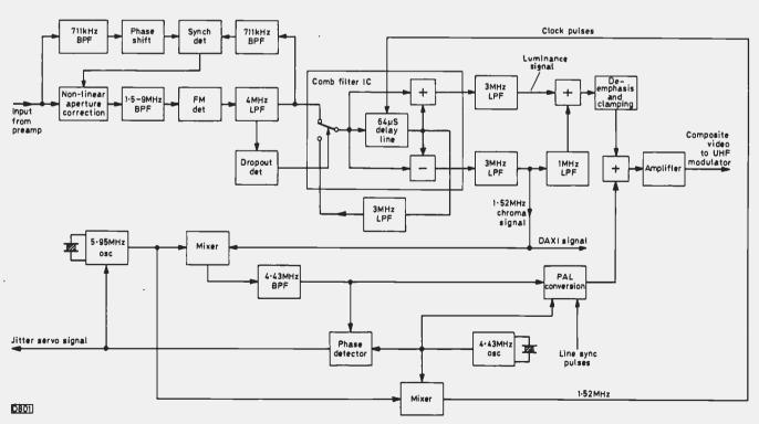
Fig. 5: Block diagram of the video signal processing system.
