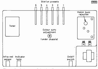
Fig. 1: Basic layout of the Ayr T11 teletext adaptor.
