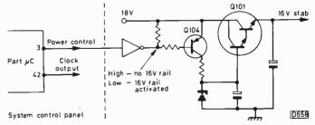
Fig. 1: 16V regulator circuit, Hitachi Model VT11E.
