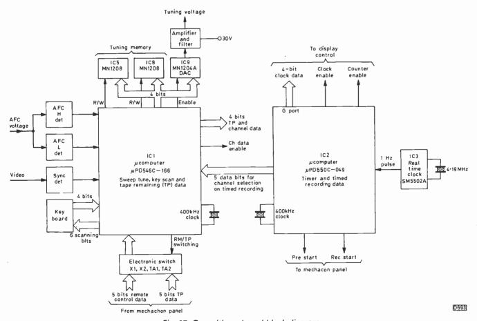
Fig. 97: Tuner/timer board block diagram.
