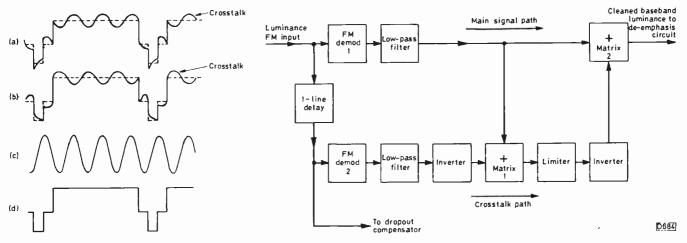
Fig. 13 (left): Luminance signals with crosstalk. (a) Direct signal. (b) One-line delayed signal. (c) Crosstalk signal obtained at the output from matrix 1 (see Fig. 14). (d) The effect of subtracting (a) and (c) in the correct proportions – the crosstalk ripple is cancelled.
