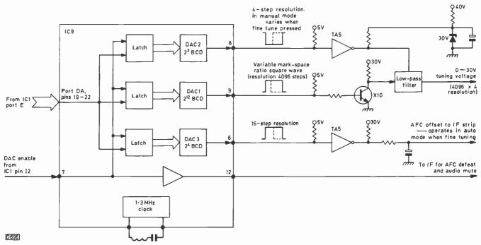
Fig. 100: Digital to analogue converters and tuning voltage integrator.
