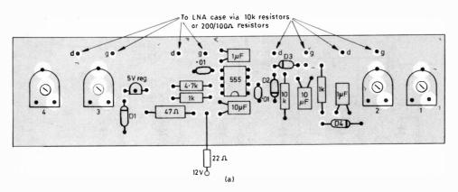
Fig. 6: Power supply PCB track pattern and component locations.
