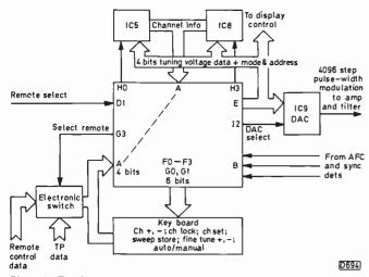
Fig. 98: Tuning system block diagram.
