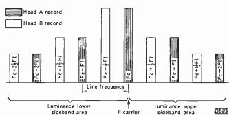
Fig. 12: How the positions of the luminance "energy packets" are interleaved on the tape. The f.m. carrier signal recorded by head A is at the nominal carrier Fc, the sideband components spacing themselves on each side at multiples of the line frequency. Head B records an f.m. signal at 7-8kHz below that of head A, so that the sidebands interleave with those recorded by head A. Thus the clear and shaded components in the diagram appear on alternate tape tracks.
