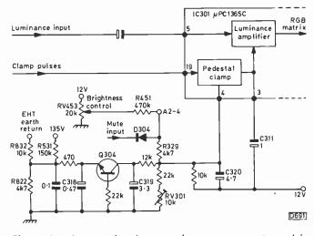
Fig. 1: Luminance signal processing arrangement used in the Sony Model KV2201UB.
