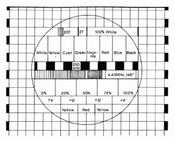
Fig. 6: The composite test pattern.
