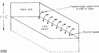
Fig. 4: Amplifier board in its case - "cut-away" view.
