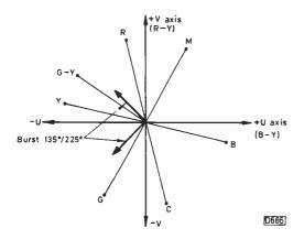
Fig. 2: Colour phase axes.
