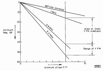
Fig. 10: Effect of azimuth offset at different frequencies.
