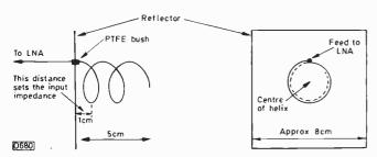
Fig. 7: Simple helical feed system.
