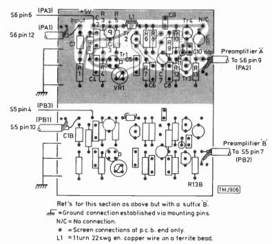
Fig. 12: Preamplifier component layout.
