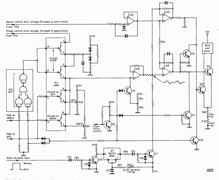
Fig. 82: Drum motor control arrangements.
