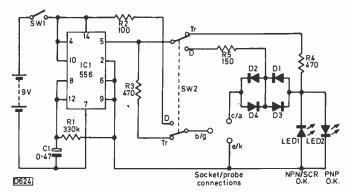
Fig. 2: Complete circuit. Diodes are tested by being connected across the collector-emitter terminals.
