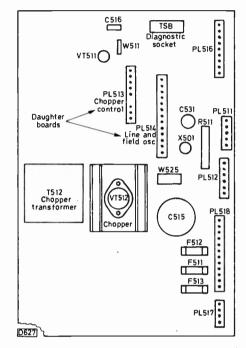
Fig. 2: Items on the right side power supply panel.
