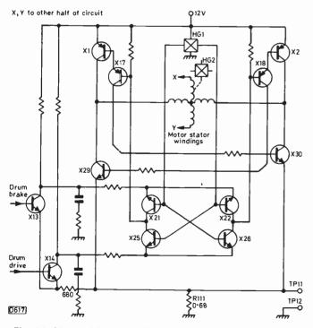
Fig. 84: Motor drive amplifier circuit.
