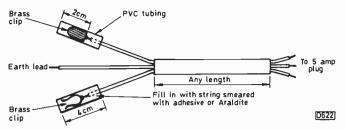
Fig. 2: DIY adaptor for converting a 13A plug for operation from a 5A socket.
