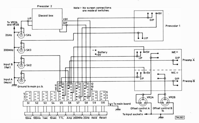
Fig. 11: Interwiring for the complete assembly.
