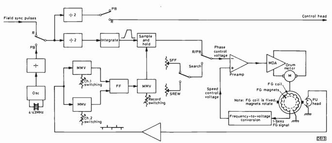
Fig. 80: The drum motor control system used in the 3V23.
