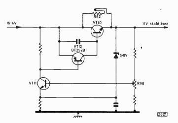
Fig. 1: Series regulator circuit used in the Bush Ranger Model BM6514. With a light load and VT10 non-conductive the output remained at 11V.
