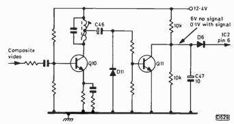
Fig. 1: Sound muting circuit, Ferguson 3V29.
