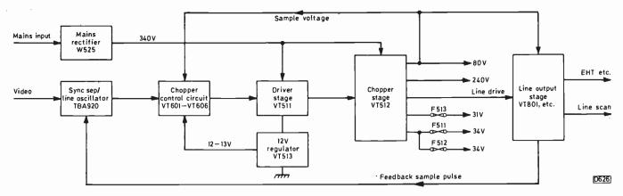
Fig. 1: Power supply/line timebase arrangement used in the Thorn 9600 chassis.
