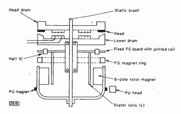
Fig. 83: The head drum/motor assembly.
