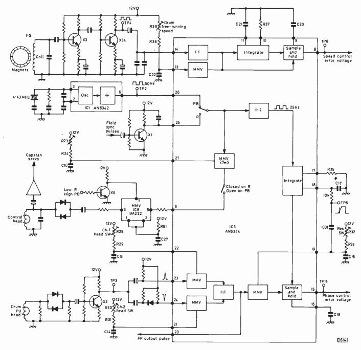
Fig. 81: The servo systems that provide drum speed and phase control.
