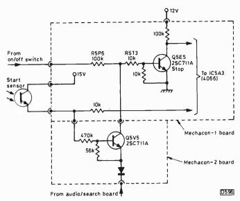
Fig. 2: Start sensor circuit, Mitsubishi HS300B.
