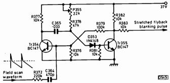
Fig. 2: Monostable multivibrator circuit used in 20AX GEC sets to lengthen the field flyback blanking pulses.
