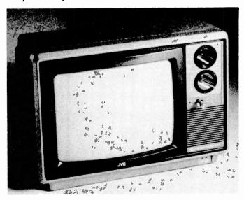
The JVC VM14PSN multi-standard video monitor. The two large switches on the right-hand side are for standard selection (five positions, auto/PAL/SECAM/NTSC-4-43/NTSC, top) and for input selection (three positions, A/B/VTR, below).
