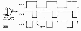
Fig. 2: Waveforms found at one of the gates in IC9.
