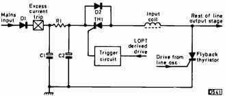
Fig. 1: Energy-dumping principle. When the regulator thyristor TH1 is triggered on, excess energy developed in the line output stage is returned to the smoothing capacitor C2.
