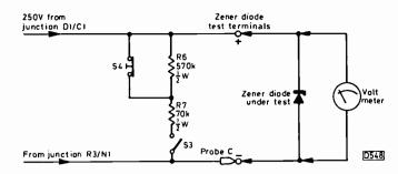
Fig. 1: Adding a zener diode test to Walter Spencer's capacitor tester (see also Letters October 1982).
