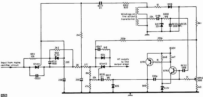
Fig. 2: Regulator, slow-start and electronic trip circuits used in the Rediffusion Mk. III chassis. 6R3, 6C13 and 6D2 provide the slow-start feature. 6THY2 is the regulator thyristor, which is triggered by the pulses produced by 6TR1/2. The electronic trip thyristor switches off in the absence of pulses from the line output stage.
