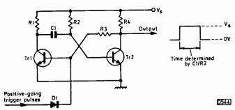
Fig. 1: Basic monostable multivibrator circuit.
