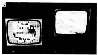
Photograph showing a converted signal display (left) and the same signal applied directly to a system I receiver (right).
