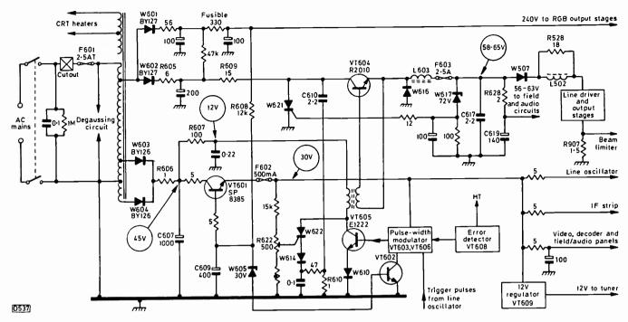
Fig. 1: The power supply arrangements used in the Thorn 3000/3500 chassis – simplified circuit. W621 is the over-voltage trip and W622 the excess current trip. F601 omitted in later production chassis.
