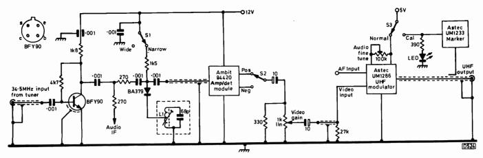
Fig. 2: Circuit diagram of the system L-I converter.
