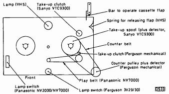
Fig. 2: Top view of the cassette compartment, showing various items that might require attention in different machines.
