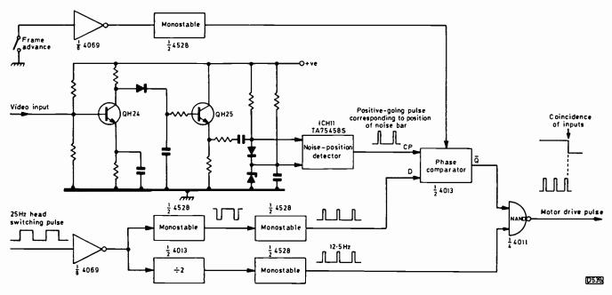
Fig. 66: Freeze-frame circuit used in the Toshiba V5470.
