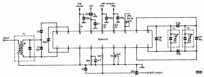
Fig. 3: Circuit of the Ambit 94420 module - 35MHz version.
