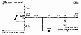
Fig. 2: C.R.T. grid bias/blanking circuit.
