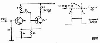
Fig. 3: Basic Schmitt trigger circuit.
