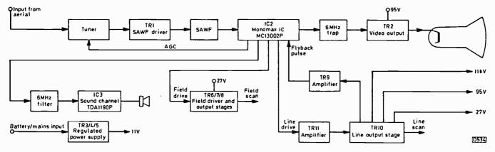
Fig. 1: Block diagram of the Thorn 1790 series chassis. IC1 (not shown) is the ZTK33 tuning voltage stabiliser.
