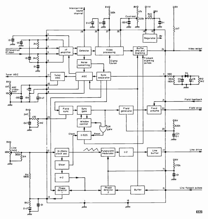
Fig. 2: Block diagram of the Motorola MC13002P Monomax i.c., with external components as used in the Thorn 1790 chassis. The height control acts on the feedback applied to pin 21.
