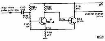
Fig. 4: Schmitt trigger circuit used in remote control versions of the Philips G11 chassis to shape the pulse fed to the channel change i.c.
