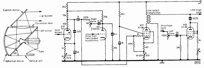
Fig. 1 (left): The Mullard optical unit for use in projection receivers. Fig. 2 (right): The line timebase circuit used in the Decca Model 1000, with left and right form correction stages to compensate for the distortion introduced by the optical system.
