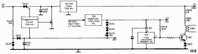
Fig. 1: Outline of the power supply arrangements used in the Telefunken 711 chassis. In the absence of an output from the 12V regulator, D422 will attempt to take over the supply to the U3 rail and the 26V line will fall to around 14V.
