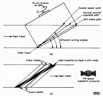
Fig. 60: Different head scanning angles on normal playback, still frame and double speed (a). Still frame conditions with the Philips Model N1502 (b).
