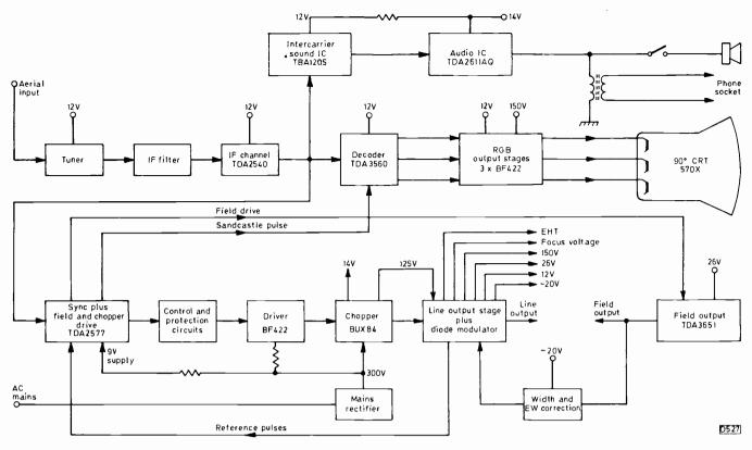
Fig. 1: Block diagram of the Philips CTX chassis.
