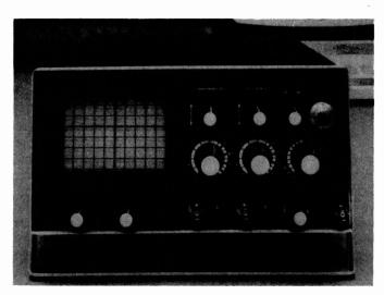
The Scopex 14D-10V oscilloscope.
