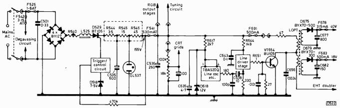
Fig. 1: Basic power supply arrangements used in the Pye 713/5/7 series chassis. Use of the mains bridge rectifier means that the chassis is at half mains potential. The line output transformer also feeds the line shift and c.r.t. first anode supply rectifiers.
