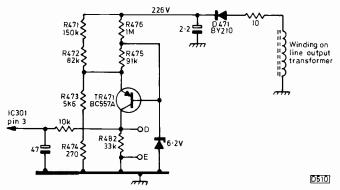
Fig. 1: Over-voltage trip circuit, Toshiba T24 chassis.
