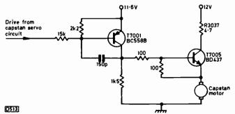
Fig. 3: Capstan drive circuit, Philips VR2020.
