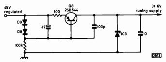
Fig. 2: Tuning voltage supply circuit, Ferguson 3V29 and 3V30. Q8 is forward biased by D8/9 and acts as a constant-current source for IC3.
