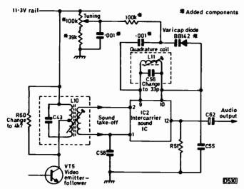
Fig. 1: Robin Crossley's tunable sound i.f. circuit. To align, set the potentiometer mid-way, tune in a 6MHz signal and peak L10/11 for maximum sound. Tune in 5·5 and 6MHz transmissions and check the potentiometer's tuning range (should exceed ±1·5MHz about centre). Repeak if necessary.
