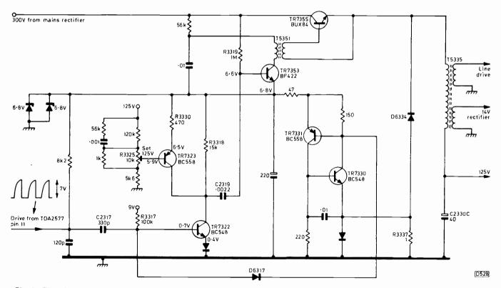
Fig. 2: The chopper transistor TR7355 and its control circuit. The chopper part of the circuit is shown in simplified form.
