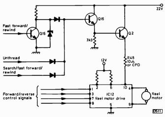
Fig. 1: Reel motor drive/control arrangement used in the Ferguson 3V29 and 3V30.
