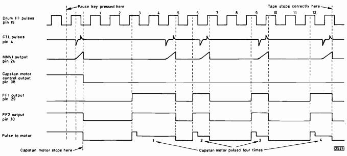
Fig. 65: Timing chart for freeze frame operation.
