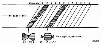
Fig. 61: Conditions when the tape is stopped with the JVC/ Ferguson HR3330/3V00.
