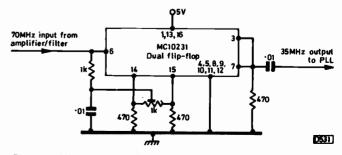
Fig. 2: Divide-by-two circuit to obtain a 35MHz output.
