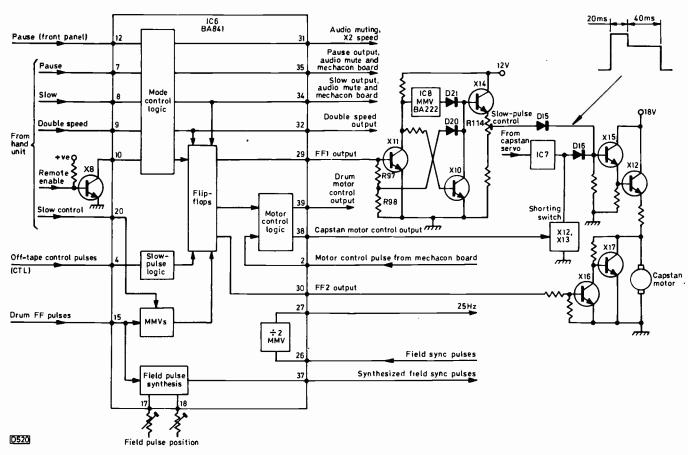
Fig. 64: Motor control arrangements for freeze frame and slow motion.
