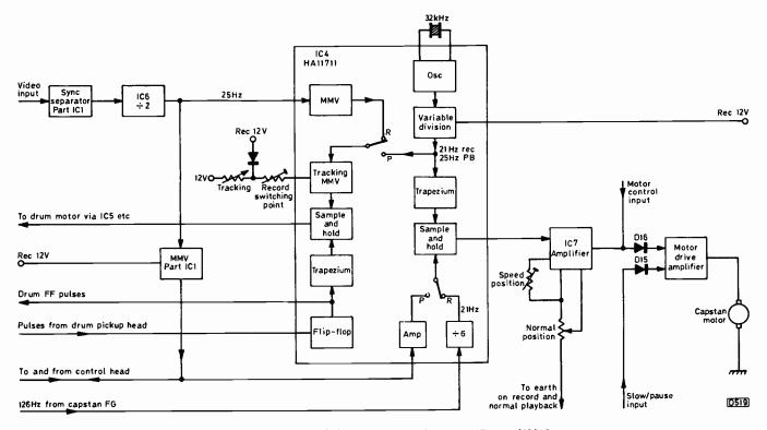
Fig. 63: Block diagram of the servos used in the HR3660/3V16.
