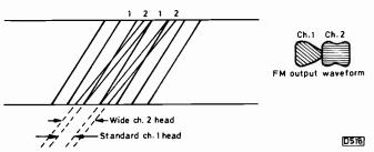
Fig. 62: Same conditions with the HR3660/3V16 with its wide channel 2 head.
