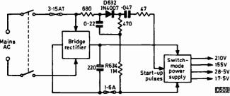
Fig. 2: Start-up circuit, Körting chassis 9.
