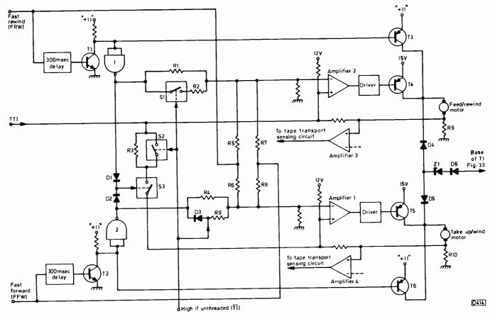
Fig. 32: Feed/take-up motor control circuit.
