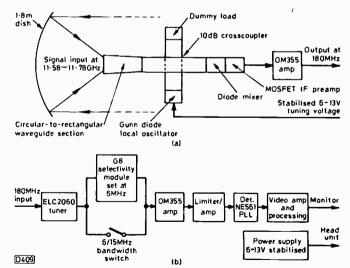
Fig. 1: Arrangement being used by Chris Wilson and Grahame Harding for reception from the OTS-2 satellite. (a) Aerial and head unit – the OM355 amplifier is required only when there's a long cable run. (b) Indoor unit.
