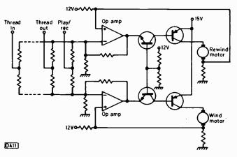
Fig. 29: Basic motor control circuit.
