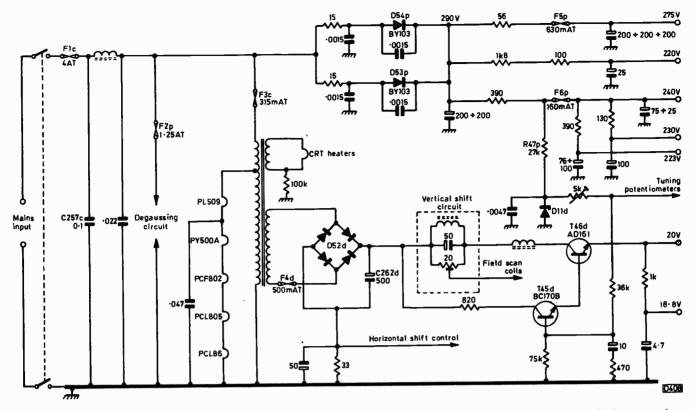
Fig. 1: Power supply circuits, ITT CVC5 chassis. Some models have only one h.t. rectifier. Modifications in later versions include extra fuses and fusible resistors, use of a simpler mains filter and omission of the 18·8V rail.
