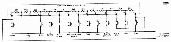
Fig. 2: Control button circuit.
