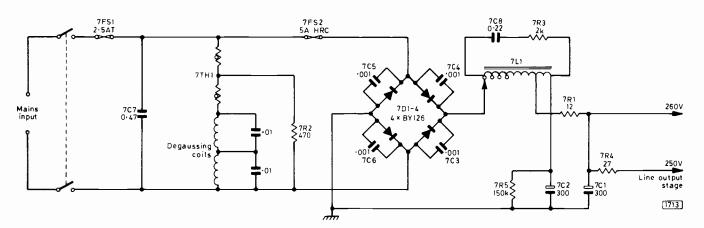
Fig. 2: The mains input, degaussing and h.t. circuits.
