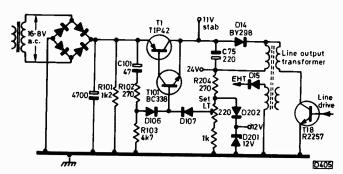
Fig. 1: Power supply arrangements used in the ITT VC402 chassis. C101 discharges via R101 at switch off.
