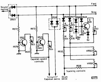
Fig. 4: Fast/slow play circuit extras on main board.
