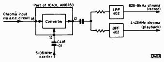
Fig. 1: Colour converter arrangement, JVC Model HR7300.
