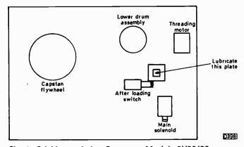
Fig. 2: Sticking switch - Ferguson Models 3V29/30.
