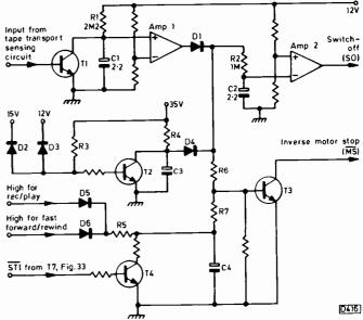
Fig. 34: Generating the protection signals.
