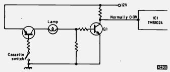
Fig. 3: Cassette lamp system, JVC Model HR7300
