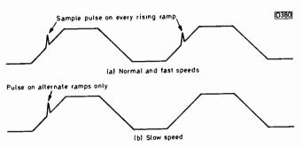
Fig. 7: Fast/slow setting up with an oscilloscope.
