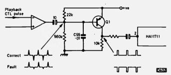
Fig. 4: Capstan servo pulse generator stage, JVC HR7300.
