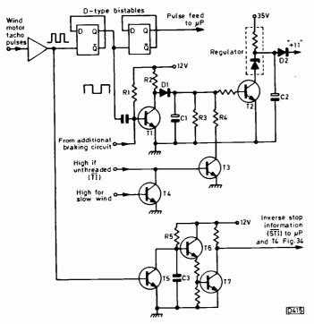
Fig. 33: Pulling motor speed control and inverse stop information circuits.
