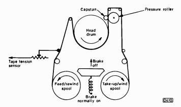
Fig. 28: Layout of the tape transport system.
