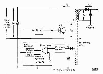
Fig. 6: Basic arrangement of the chopper power supply.
