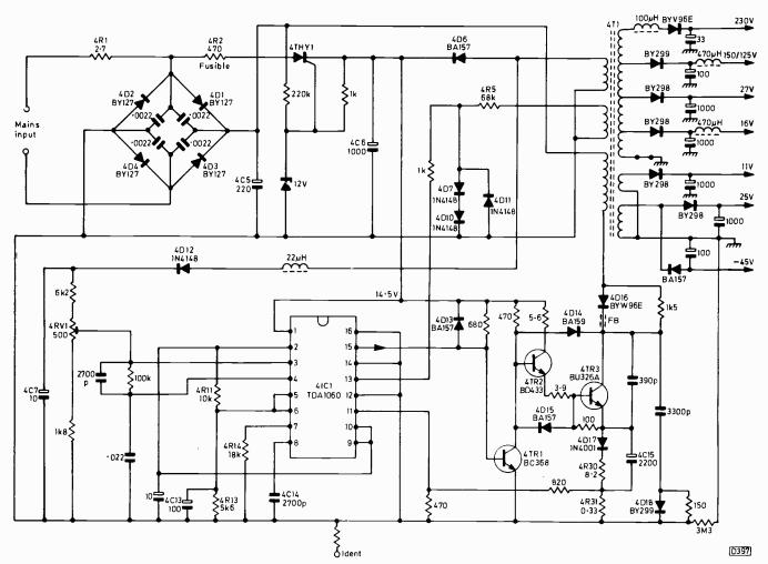
Fig. 8: Full circuit of the switch-mode power supply. The different versions of the board have different value resistors connected to the ident pin so that they can be automatically identified by the production test equipment.
