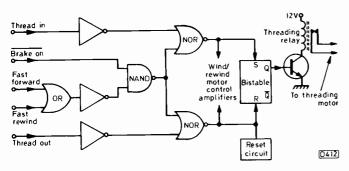
Fig. 30: Method of controlling the threading motor.
