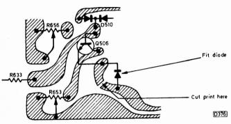
Fig. 3: Fast/slow modification, main board.
