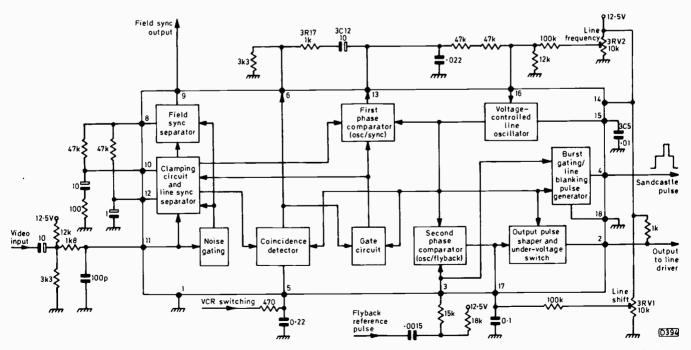
Fig. 5: Block diagram of the TDA1950 sync/line generator i.c. Pin 18 enables field flyback blanking pulses to be fed in to obtain a composite blanking/gating pulse waveform: as this facility is not used the pin is connected to chassis.
