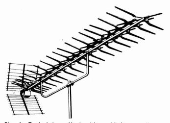
Fig. 1: Typical long Yagi with multi-element director assemblies.
