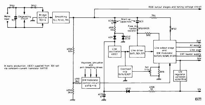
Fig. 1: General arrangement of the h.t. supply, line timebase and EW modulator circuits in the Rank Z718 chassis.
