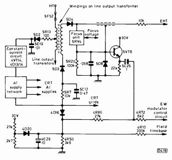
Fig. 3: The e.h.t., focus, c.r.t. first anode, grid bias, antibreathing and beam limiting circuits.
