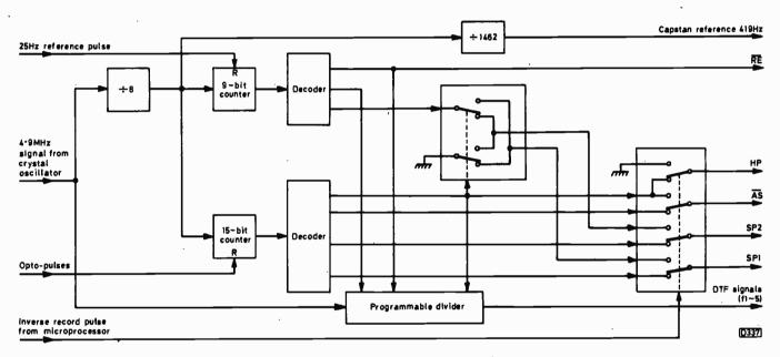
Fig. 20: Later system in which all the control signals are counted down from the output of a 4-9MHz crystal oscillator.
