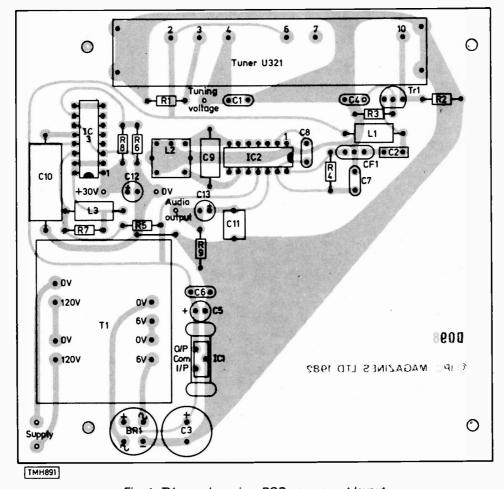
Fig. 1: TV sound receiver PCB component layout.
