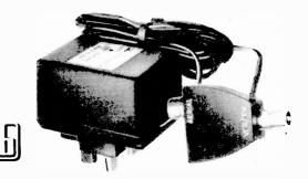
The Wolsey 'Super-Vision' is a single output low noise UHF amplifier intended for boosting the input signal to a VCR and/or TV receiver combination. The compact amplifier module inserts directly into the coaxial input socket and is DC powered (via twin lead) from the mains power unit (with its integral 13 amp plug).
