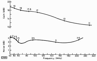
Fig. 2: Gain and noise characteristics, measured with 75 $\Omega$  input/output and a 9V, 4mA supply.
