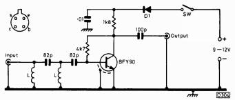
Fig. 1: Circuit diagram. The coils marked L consist of ten turns each of 28g wire, close spaced at 1/10in. diameter. Use 100V ceramic coupling capacitors and 1/8 or 1/3W carbon film resistors. Any silicon diode can be used in position D1, e.g. type 1N4002 etc.
