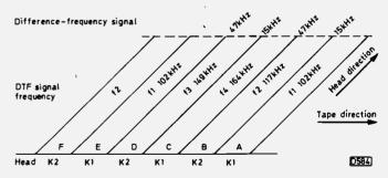
Fig 12: Arrangement of the DTF signals on the tracks.
