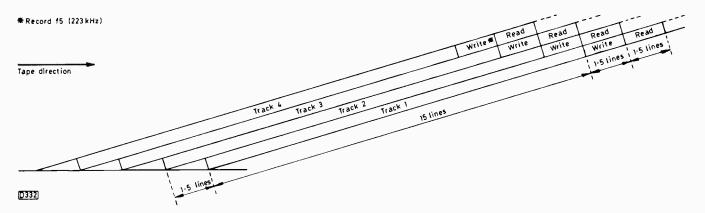
Fig. 15: Extra signals (f5) are laid down to control the heads on record.
