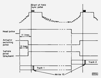
Fig. 17: HP, AS and SP1/2 pulse timing relative to the field sync pulse.
