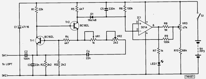
Fig. 1: Circuit of the line output transformer tester.
