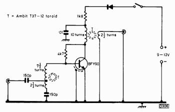
Fig. 3: Alternative input/output arrangements using Ambit r.f. toroids.
