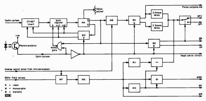
Fig. 19: Generating the control pulses.
