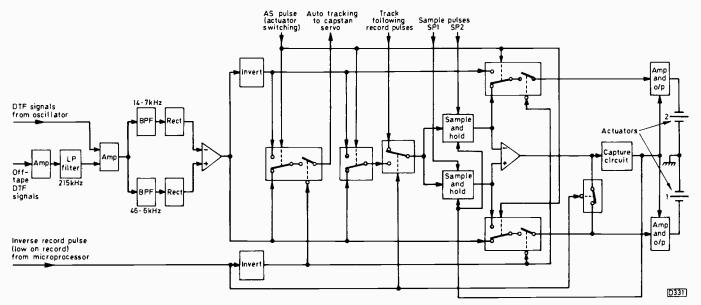
Fig. 14: Block diagram of the actuator control system.
