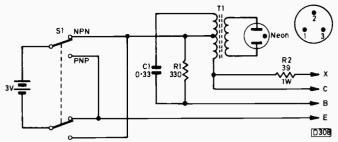
Fig. 2: Modified version of Mike Phelan's in-situ transistor tester devised by Walter Spencer, with an extra lead for additional tests. Walter reports using an  $0.22\mu F$  capacitor in the C1 position and a  $560\Omega$  resistor in the R1 position – the values of these components are not critical.
