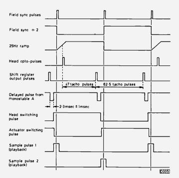
Fig. 18: Timing of the various control pulses.
