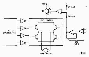
Fig. 3: Reel motor drive, Baird Model 8930.
