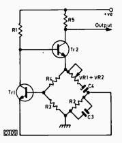
Fig. 2: The oscillator circuit redrawn to show the bridge circuit, with Wien network for positive feedback.
