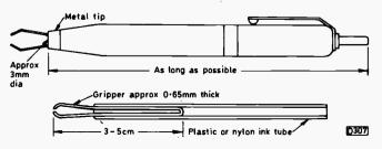
Fig. 1: Victor Rizzo's nut and bolt retriever.
