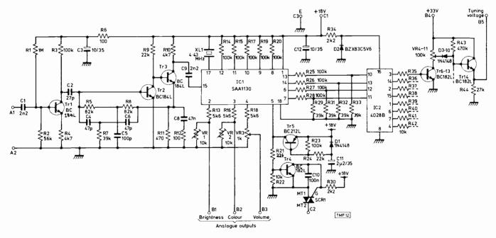
Fig. 2: Circuit diagram of interface board.
