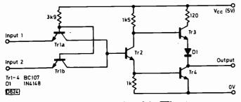
Fig. 2: Discrete component version of the TTL gate.
