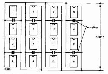
Fig. 7: Supply arrangements with TTL – a typical generalpurpose PCB layout.
