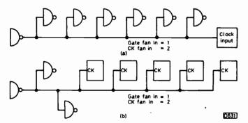
Fig. 9: Fan out and fan in. (a) An allowable configuration – the gate at the left has a fan out of 10, driving a total fan in of 8. (b) Non-allowable configuration. The gate, with its fan out of 10, is linked to 12 fan ins.
