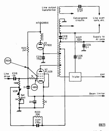
Fig. 3: Simplified circuit of the line output stage used in Pye hybrid colour chassis. This time the boost capacitor (C218) is returned to chassis. There is no h.t. fuse in this chassis, nor any fusible resistors in the h.t. supply. As a result, a shortcircuit in C219, C218 or C224 will blow the mains fuse.
