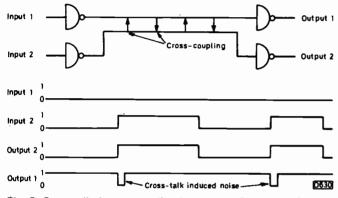
Fig. 8: Crosstalk due to coupling between adjacent tracks.
