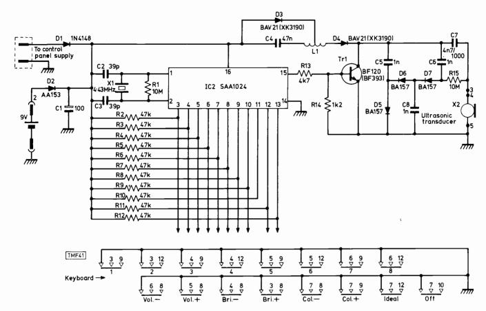
Fig. 1: Complete circuit diagram of ITT remote control transmitter. Note that the plug labelled "to control panel supply" is not used in our application.
