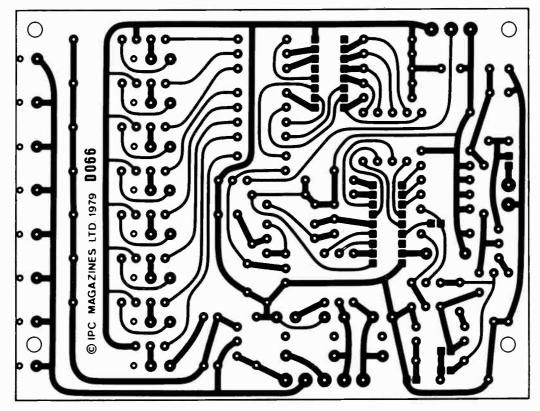
Fig. 4: Copper print pattern for interface board ref. D066.
