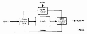
Fig. 6: Last ditch screening to eliminate external noise.
