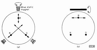
Fig. 3: Radial movements (a) of the three beams, under the influence of adjustable permanent magnets, to converge the beams at the centre of the screen (static convergence). (b) The blue beam requires horizontal as well as radial movement in order to align it with the red and green beams.
