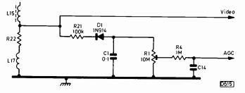
Fig. 3: Suggested alternative circuit. In this case leave R21 in place and disconnect V8 and C28.
