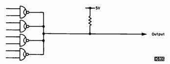
Fig. 11: Use of open-collector gates to provide the "wired-OR" logic function.
