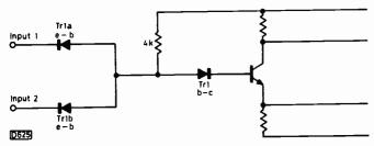
Fig. 3: Diode analogy of the action of Tr1 in Fig. 1.
