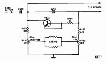
Fig. 7: Modified blue vertical convergence circuit used in later versions of the Pye hybrid chassis.
