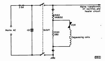
Fig. 8: The tube degaussing (demagnetising) circuit used in Pye hybrid colour receivers.
