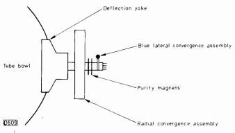
*Fig. 4: Positions of the various correction assemblies on the neck of a delta-gun shadowmask tube.*
