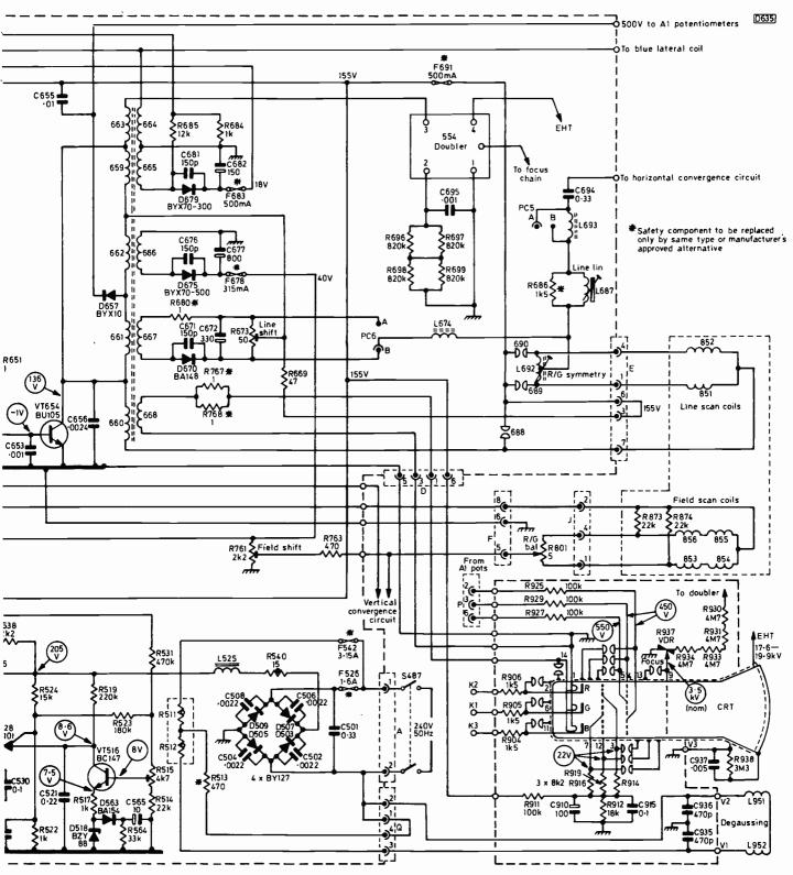
The 713 chassis has a different focus arrangement (see text).
