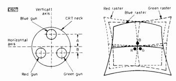
Fig. 1 (left): Arrangement of the electron guns in the neck of a delta-gun tube. Note that distance A along the vertical axis is roughly twice distance B, so that a greater current is required in the blue dynamic convergence coils than in the red and green coils.
