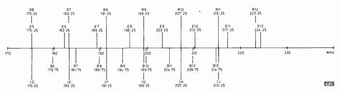
Fig. 1: European Band III vision carrier frequencies. The R channels are used in East Europe, with 6·5MHz sound/vision spacing (system D); the E channels in West Europe with 5·5MHz sound/vision spacing (system B); the I channels in Eire with 6MHz sound/vision spacing (system I); and the B channels in the UK with 3·5MHz sound/vision spacing (system A). System A has 405 lines and positive vision modulation, all the other systems 625 lines with negative vision modulation.
