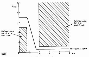
Fig. 5: TTL gate transfer characteristic.
