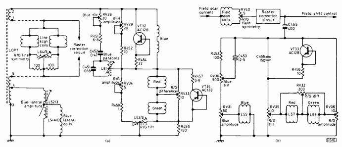
Fig. 5: The line (a) and field (b) convergence circuitry used in Pye hybrid colour sets. The line convergence circuitry is connected in series with the line scan coils via windings 3-5 and 1-2 on the line output transformer.
