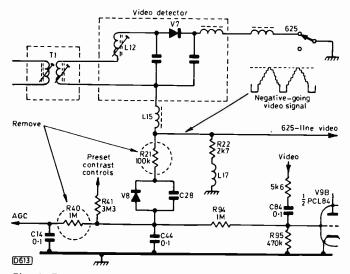
Fig. 1: The original mean-level a.g.c. circuit used in the Pye 11U series receivers. Removing R40 disconnects the controlled stages from the existing a.g.c. circuit; removing R21 or V8 and C28 eliminates unnecessary loading on the video detector diode V7.
