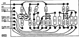
Fig: 3: Component layout on the board.
