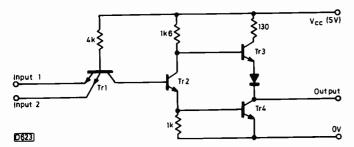
Fig. 1 : Standard TTL gate circuit.
