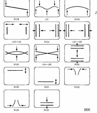
*Fig. 6: The effects produced by the various convergence controls in the circuit shown in Fig. 5.*
