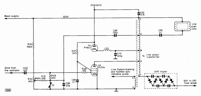
Fig. 2: Typical monochrome receiver line output stage (Thorn 1500 chassis, 20kV version). Check the line output transformer tuning capacitor C113 if a resistance check from the cathode of the boost diode to chassis reveals a short-circuit. This would open R124 (see Fig. 1). The boost capacitor C92 is returned to the h.t. rail and will thus give the sound, no raster symptom when it goes short-circuit.
