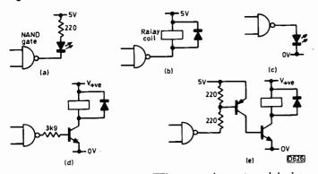
Fig. 4: Interfacing between a TTL gate and an external device. (a) Driving a LED. (b) Direct drive to a reed relay. (c) Alternative LED drive. (d) Driving a high-voltage relay. (e) Driving high current loads.
