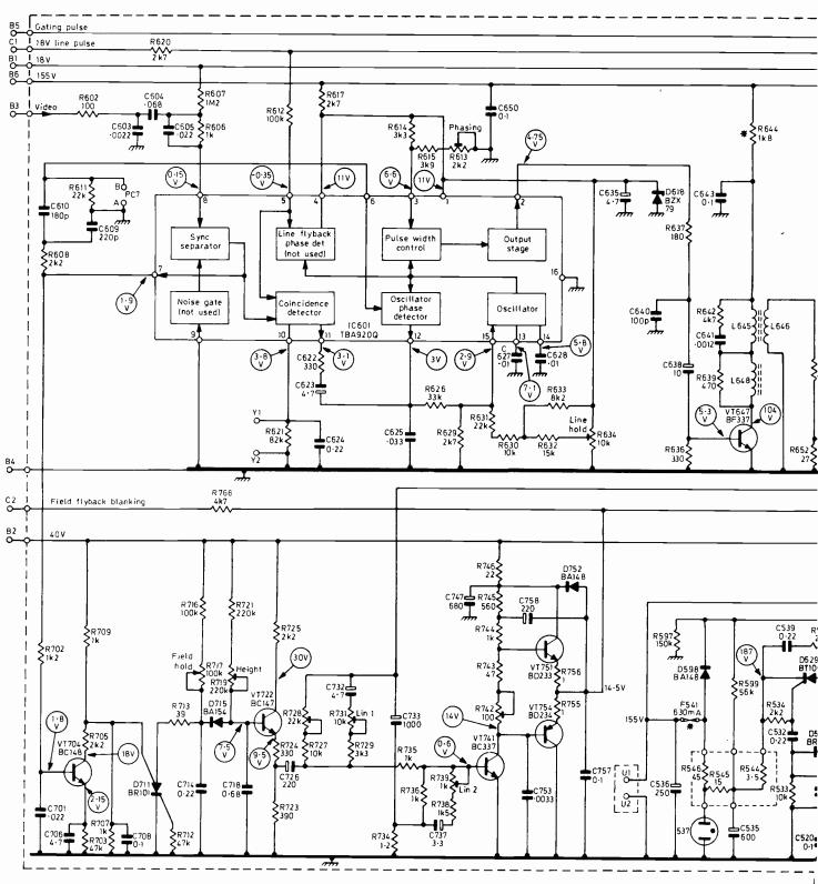
Fig. 7: Power supply and timebase circuits, Pye 715 and 717 chassis.
