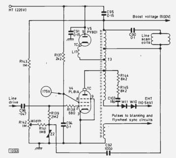
Fig. 1: The line output stage used in the Thorn 1580 chassis. This is quite conventional, with the boost reservoir capacitor C95 returned to the h.t. line. R144/R145/C103 form a damping network, C103 also providing third harmonic tuning.
