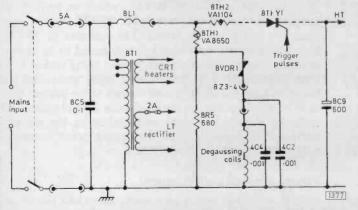
Fig. 1: Mains input circuit, Rank A823 colour chassis. Failure of the 5A mains fuse was found to be the result of a fault in the degaussing circuit.
