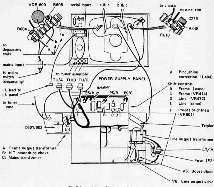
Fig. 3: Internal view, with the chassis folded flat.
