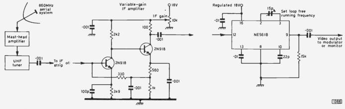
Fig. 1: Steve Birkhill's receiving system for the Indian ATS-6 satellite transmissions. The signal picked up by the dish passes via a mast-head amplifier to the u.h.f. tuner and then to either the two-stage i.f. amplifier shown above or a conventional i.f. strip. The amplified i.f. signal is demodulated by an NE561B phase-locked loop i.c.
