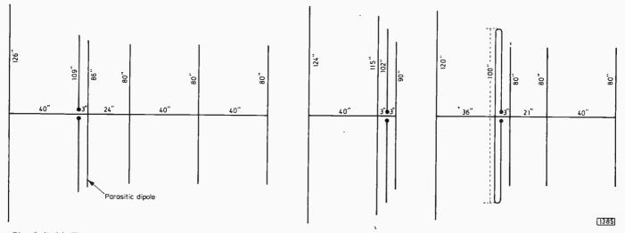
Fig. 2 (left): The Doug McFayden Band I aerial, covering New Zealand channels 1-3. Fig. 3 (centre): lan Beckett's design for a small, wideband Band I array. Fig. 4 (right): My own recently-constructed Band I design, using a folded dipole.
