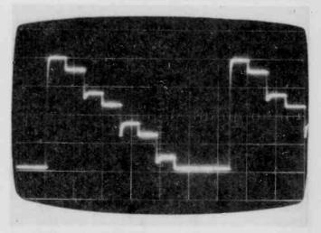
The generator output waveform. (Scale – Vertical: 0.5V/cm, Horizontal:  $10\mu s/cm$ .)
