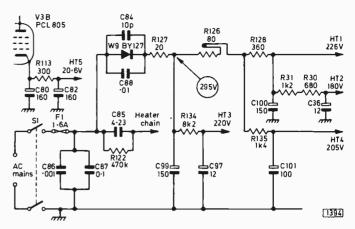
Fig. 2: The power supply arrangements used in the Thorn 1580 chassis. Capacitor C85 forms the heater circuit dropper, with R122 providing a discharge path. The field output pentode's cathode current is drawn via the low-voltage transistor circuits to provide the 20.6V supply (HT5).
