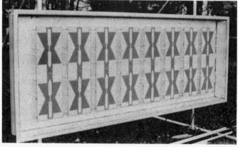
Fig. 1: A prototype single-bay adaptive aerial, shown with protective cover removed.
