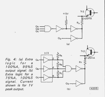
A 75% amplitude, 100% saturated signal is produced by adding one triple-input NAND gate and two open-collector inverter gates (Fig. 4(b)). In this case RA, RB and RC are chosen such that A = 8, B = 23 and C = 44. When all three counter outputs are at 0, resistor RY is unconnected. At all other counts it is switched into Tr2 emitter circuit and passes an extra 0.25mA. The inverted QD output is again connected in wired-OR mode to RY.
