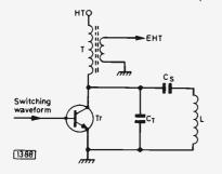
Fig. 2: Transistor line output stages usually take the form shown here. The transistor acts as a bidirectional switch, acting as efficiency diode (energy recovery) during the first half of the forward scan, then driving current through the primary of the output transformer T during the second half of the forward scan. Ct tunes the coils -L – during the flyback, while the scan-correction capacitor Cs charges and discharges during the forward scan to drive current through the scan coils.
