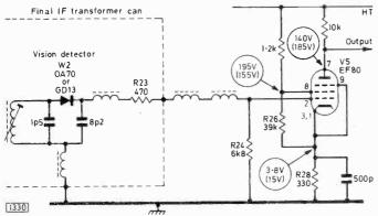
Fig. 3: Method of biasing the video output valve (V5) in the Thorn 980 chassis. Incorrect voltages, shown in brackets, were due to the bias stabilising resistor R26 having fallen in value to less than  $3k\Omega$ .
