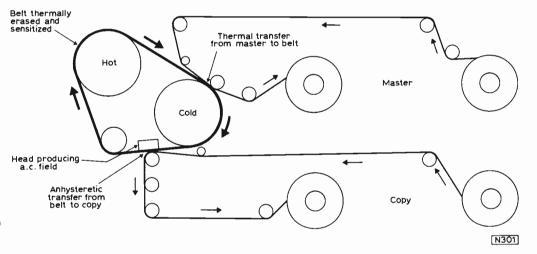
Fig. 1: Basic principle of the STAM high-speed contact copying process.
