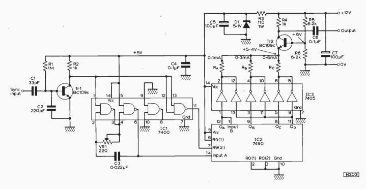
Fig. 2: Complete circuit of the simple grey-scale generator. The currents shown for RA, RB, and RC, are those required to produce an output signal of 1 V peak amplitude. See section "Modifications".
