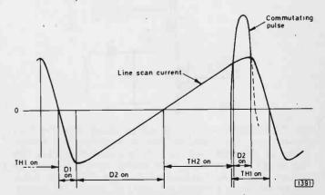
Fig. 5: Current waveforms during the scanning sequence, showing which active components are conducting during the various stages of the scan cycle.
