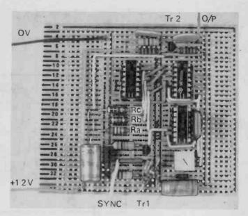
The completed generator, constructed on a West Hyde Prototype board.
