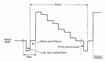
Fig. 1: The grey scale video signal. Each step lasts approximately  $6.5\mu s$ .
