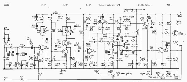
Fig. 4: Circuit of the i.f. strip. In the 30 series chassis R68 and C79 are omitted and a 41-5MHz trap is added in the detector circuit. With varicap tuners R58 and R60 are  $100k\Omega$ , R61, R62 and C68 are omitted and the junction of R60-C67 is connected to chassis.
