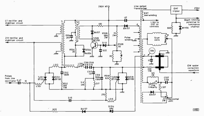
Fig. 6: A practical thyristor line output circuit – as used in the Grundig Models 5011 and 6011. Width/e.h.t. stabilisation is achieved by shunting a transductor (Td1) across the input transformer. The impedance presented by Td1 is controlled by Tr506 which senses the h.t. voltage and the pulse voltage at tag d on the line output transformer. R518 provides circuit damping; C519 provides pulse suppression to remove a shading effect across the screen.
