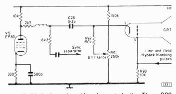
Fig. 4: Method used to bias the c.r.t. in the Thorn 980 chassis. The grid is at chassis potential while the d.c. level at the cathode is set by the brilliance control, the a.c. coupled video signal being superimposed on this bias.
