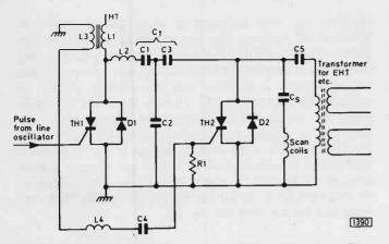
Fig. 4: A more practical form of thyristor line output stage. The tuning capacitor consists of three capacitors in a T network so that the working voltages can be reduced. C5 couples a transformer to the circuit to enable the flyback pulse to be used for the generation of e.h.t. and other supplies. The trigger pulse for TH2 is obtained from a secondary winding wound on L1, with shaping by means of L4, C4 and R1.
