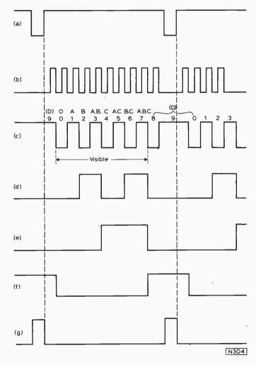
Fig. 3: Idealised waveforms. (a) Tr1 collector pulse. (b) IC2 input, pin 14. (c) IC2 output A, pin 12. (d) IC2 output B, pin 9. (e) IC2 output C, pin 8. (f) IC2 output D, pin 11. (g) Reset pulse, IC2 pin 7.
