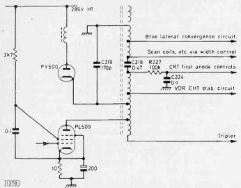
Fig. 2: Main elements of the line output stage in the Pye 691 chassis. The c.r.t. first anode voltage smoothing capacitor C224 going short-circuit blew the mains fuse. Up-rating this component from 1 kV to 1 5kV gives improved reliability.
