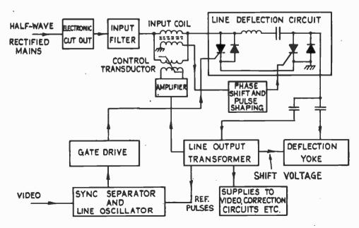
Block diagram of a thyristor line timebase, showing how it fits into the complete receiver circuit. Stabilisation is achieved by using a transductor to control the input power. Any supplies derived from the line output transformer will also be regulated therefore. Courtesy ITT.
