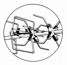
Fig. 1: Close-up showing position of the 'launch directors'.
