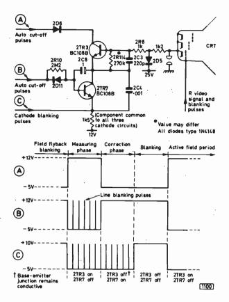
Fig. 1: Automatic grey-scale correction circuit used in the latest Bang and Olufsen colour chassis (red cathode circuit only shown), with associated waveforms beneath. During the measuring phase the cathode current is measured; during the following correction phase a clamping action sets the charge on 2C8. In this way the circuit automatically sets the cathode voltage at the start of each field period.
