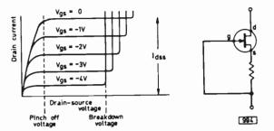
Fig. 3 (left): Id/Vds characteristics of an n-channel junction field effect transistor.
