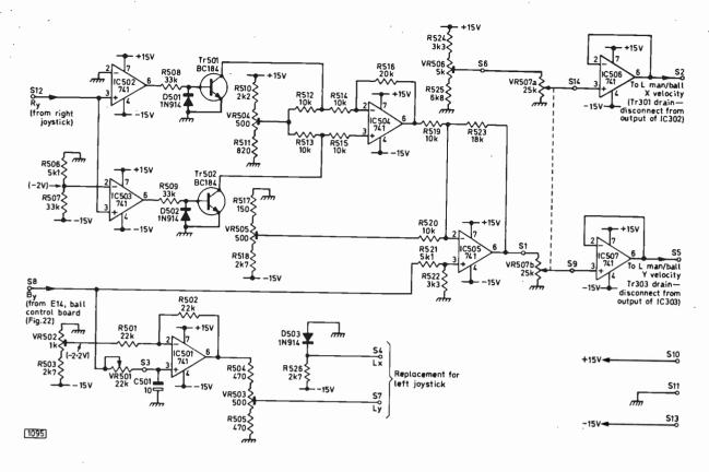
Fig. 33. Circuit for Superman, intended as a plug-in replacement for the left joystick. VR501 and VR507 are front-panel controls for setting the speed of response and kick respectively.
