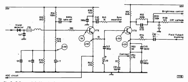
Fig. 2: D.C. coupled video circuit used in the Thorn 1590 chassis. VT6 acts as a sync preamplifier as well as a video buffer/driver stage. The 1591 chassis is the same except for R131 which is  $100k \Omega$ .
