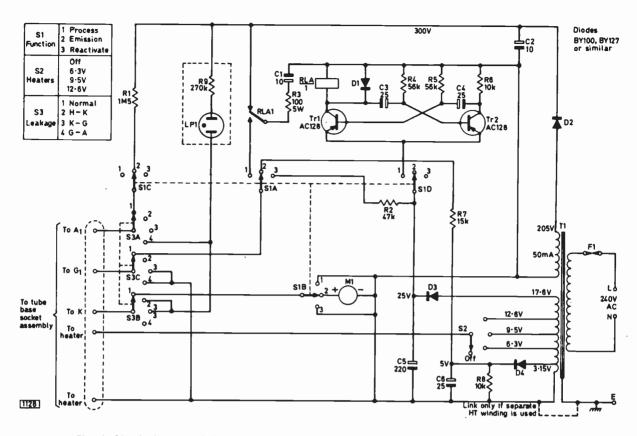
Fig. 4: Circuit diagram of the meter unit. Transformer T1 may be an auto-transformer-see text.
