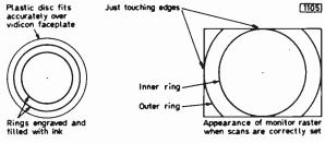
Fig. 5: Setting the scans with an engraved disc.
