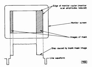
Fig. 4: Setting the line scan amplitude using the line waveform: the mask images must be centralised and expanded.
