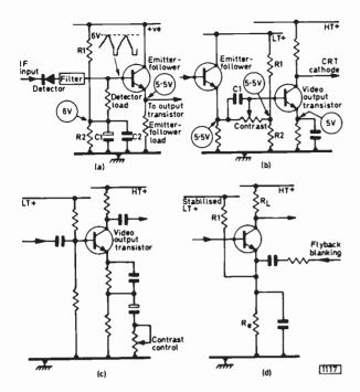
Fig. 1: Circuit techniques used in transistor video channels. (a) Method of biasing the driver stage. (b) Contrast control in a d.c. coupled circuit. (c) Contrast control by means of variable negative feedback in the emitter circuit of the video output transistor. (d) Bias stabilisation and flyback blanking techniques.
