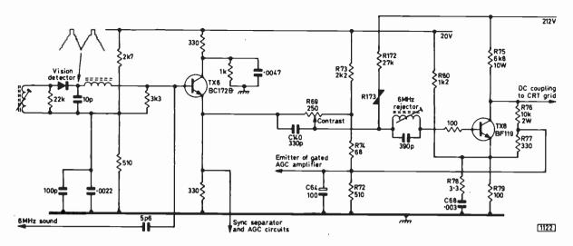
Fig. 6: D.C. coupled video channel used in the ITT VC200 chassis. The output is applied to the c.r.t. grid.
