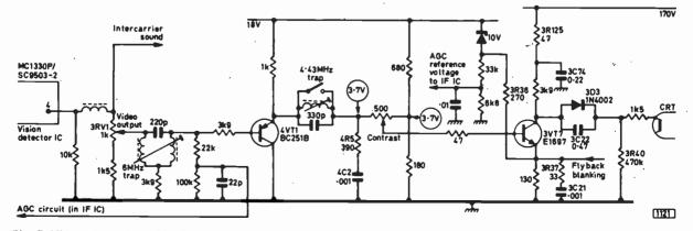
Fig. 5: Video channel used in the RRI A816 chassis, with diode beam limiter 3D3. 3RV1 sets the threshold for the a.g.c. circuit which is in the i.f. i.c. (MC1352P/SC9504P).
