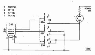
Fig. 3: A neon lamp is used to indicate inter-electrode leakage.
