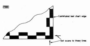
Fig. 6: Scan setting using a commercial test chart.
