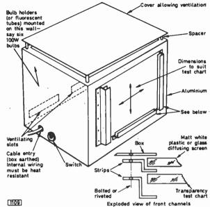
Fig. 9: Light box for CCTV setting-up work.
