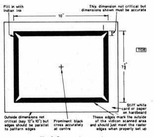
Fig. 8: Scan setting test chart.
