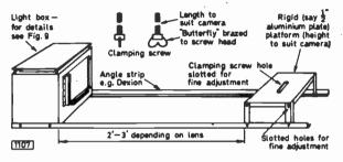
Fig. 7: Camera setting-up jig.
