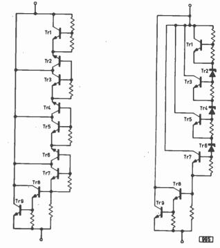
Fig. 5 (left): 35V i.c. stabiliser-internal circuit. Types TAA550 and TBA271.
