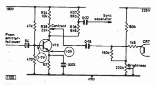
Fig. 4: Video output stage used in the Thorn 1580 chassis. Contrast is controlled by tapping the required degree of c.r.t. drive from the output transistor's collector load circuit.
