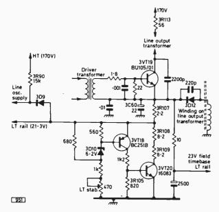
Fig. 3: The circuit used to develop the l.t. supplies in the RRI A816 chassis. The 21.3V rail is stabilised by the shunt regulator circuit which also indirectly stabilises the h.t. supply.
