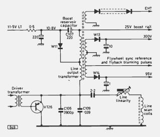
Fig. 1: Line output stage used in the TCE 1590/1591 chassis. The series efficiency diode W11 charges the boost reservoir capacitor C107 to provide a 25V boost rail. C109 tunes the transformer; C106 (270pF in the 1591 version) provides flashover protection.
