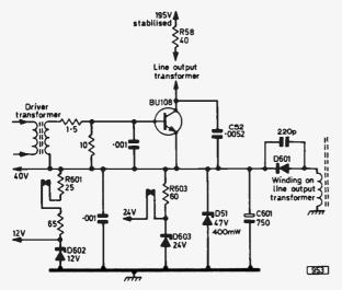
Fig. 5: Another variation on this theme: in the GEC C2110 series chassis the BU108 line output transistor sits on a 40V I.t. rail.
