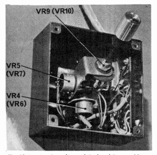
Fig. 12: Interior view of one of the joystick control boxes, showing the method of coupling together the potentiometers.
