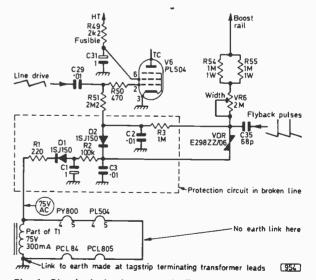
Fig. 1: Circuit devised to provide line output stage protection. Component ratings: R1-R3  $\frac{1}{2}$ W; C1 160V; C2 and C3 400V.
