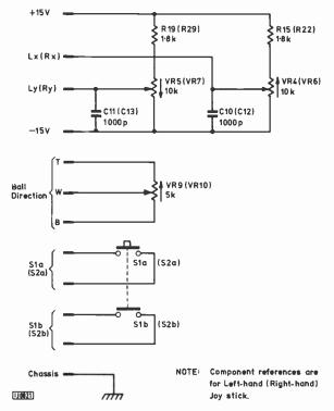
Fig. 13: Circuit of one of the joystick control boxes. Component reference numbers given apply to the left-hand box —those for the right-hand box are shown in brackets.
