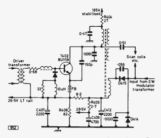
Fig. 4: A similar circuit is used to obtain the l.t. supplies in the Nordmende F IV 110° colour chassis.
