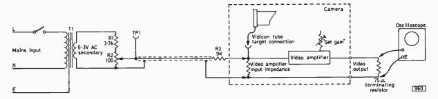
Fig. 4: Circuit and use of the gain test jig.
