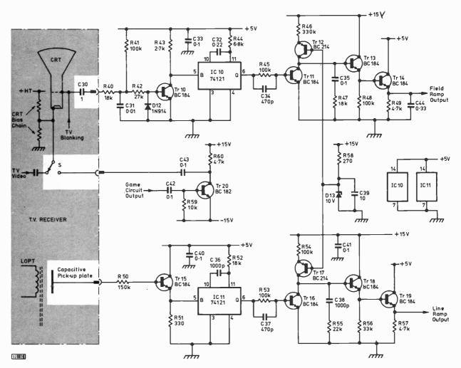
Fig. 8: Circuit diagram of the ramp generators and the TV drive circuit for use with a monochrome receiver. Existing receiver circuitry is shown within the shaded area on the left.
