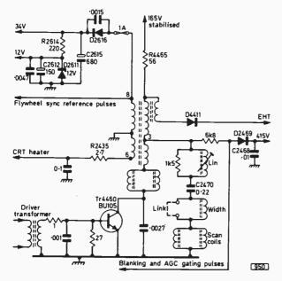
Fig. 2: Line output stage used in the Philips 320 largescreen monochrome chassis.
