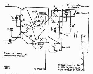
Fig. 2: Layout of the circuit as used in the "Television" 625-line receiver.
