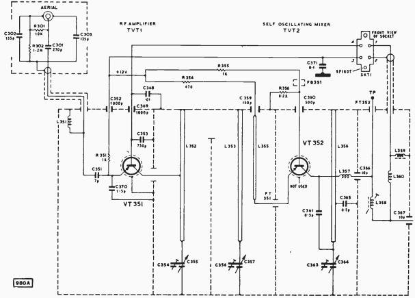
Fig. 3: Circuit of u.h.f. tuner type T21-200 used in the 1590 and 1591 chassis.
