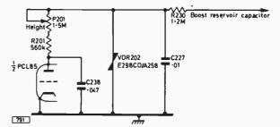
Fig. 3: Field charging circuit used in the GEC Series 1 chassis.
