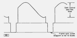
Fig. 5: Typical camera output waveform obtained when using the gain test jig.
