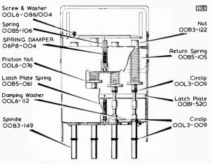
Fig. 5: Tuner push-button mechanism.
