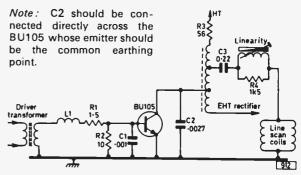
Fig. 4: The basic BU105 line output stage: the component values shown are typical of those found in practice.
