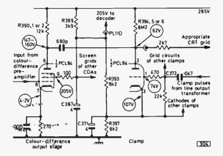
Fig. 3: Colour-difference output stage/clamp circuitry.
