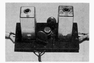
bias components are incorporated in an integrated circuit. This reduces the physical size and the stray capacitances, thus producing a more useful amplifier.
