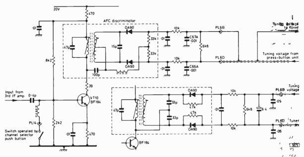
Fig. 4: Single-stage a.f.c. circuit used in chassis fitted with varicap tuners. Complete circuit, 693 chassis; below right, modifications in the 697 chassis.
