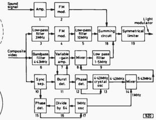
Fig. 6: Block diagram of the circuits used in recording a VLP record.
