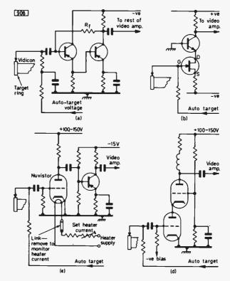
Fig. 2: Typical head amplifier circuits (simplified). (a) The feedback pair. The feedback resistor Rf may need optimising if the transistors are changed. (b) Cascode amplifier with f.e.t. input stage. (c) Valve/transistor hybrid circuit. (d) Valve cascode circuit—typically uses two nuvistors (heater circuits omitted).
