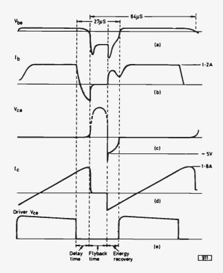
Fig. 3: Several large-screen monochrome receivers use the Mullard BU105 line output transistor. The correct waveforms in a stage using this transistor are shown above.
