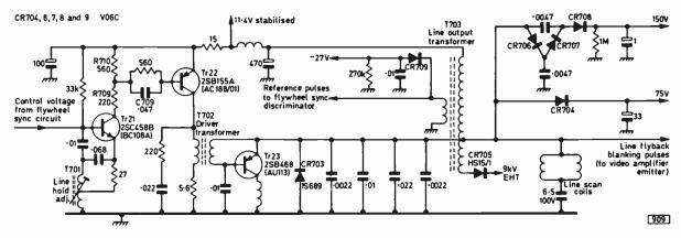
Fig. 1: Line timebase circuit used in the Ekco Model T545 9in. mains/battery portable. The pnp line output transistor Tr23 is operated in the emitter-follower mode.
