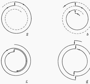
Fig. 3: Different ways of using the picture recorded on the VLP disc—twice per revolution during the field flyback period an opportunity occurs to change from one track to another. (a) A reverse jump after each revolution gives a stationary picture; (b) a forward jump after each revolution gives motion at twice the true speed; (c) reverse jump after every second revolution reduces the speed by half; (d) a reverse jump every half revolution gives reverse motion at the correct speed.
