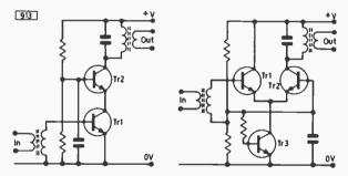
Fig. 1 (left): Cascode amplifier circuit.
