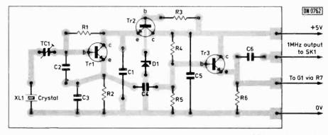
Fig. 8: Layout of the oscillator board, viewed from the copper side. (C5 is an electrolytic.)
