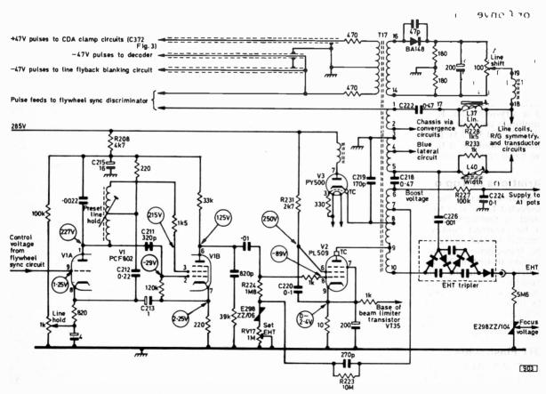
Fig. 2: Circuit of the line oscillator and output stages.
