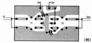
Fig. 6: Layout of the printed circuit.
