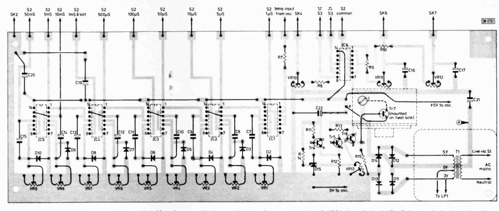
Fig. 7: Layout of the main panel used in the prototype, viewed from the copper side. Note that incorrect pin numbers were given for IC6 in the main circuit (Fig. 3) last month: the pin numbers shown there for G21 and G24 and also for G22 and G23 should be interchanged to conform with the layout above.
