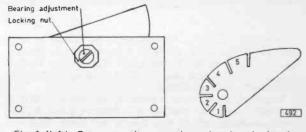
Fig. 1 (left): Gang capacitor rear view, showing the bearing adjustment screw and locking nut.
