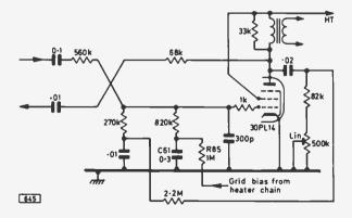
Fig. 1: Field output stage used in the BRC 980 chassis, with grid bias obtained from the heater chain.
