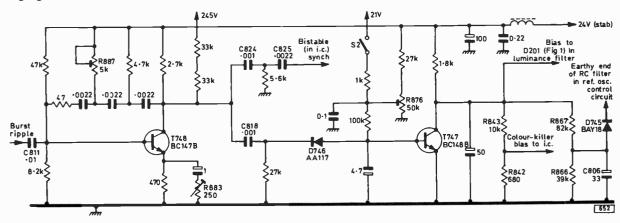
Fig. 6: The RC oscillator ident stage and colour-killer circuitry.
