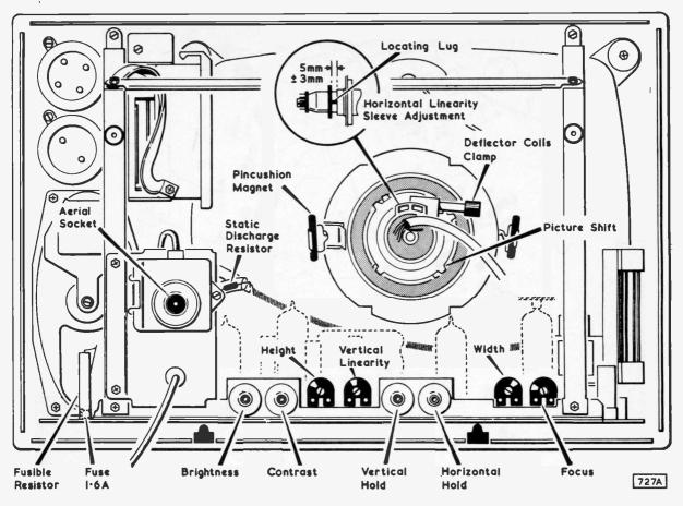
Fig. 3. Rear chassis view showing preset adjustments.
