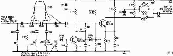
Fig. 5: The first chrominance amplifier and a.c.c. circuit.
