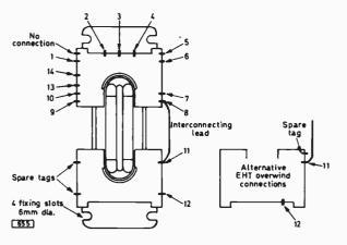
Fig. 1: Line output transformer tag identification.
