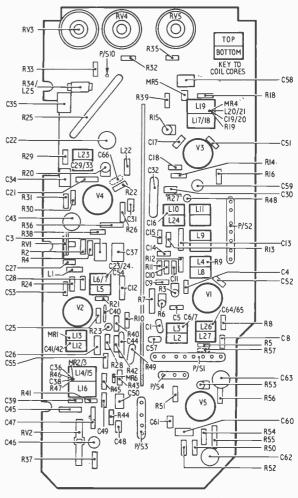
Fig. 1: Layout of the i.f. unit.
