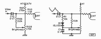
Fig. 1 (left): The video signal is a.c. coupled by C40 to the cathode of the c.r.t. in the BRC 1500 chassis. The two video stages are also a.c. coupled. Since a signal passed through a capacitor loses its reference level, this form of coupling means that the black level of the video signal is no longer stable but varies with alterations in average signal amplitude.
