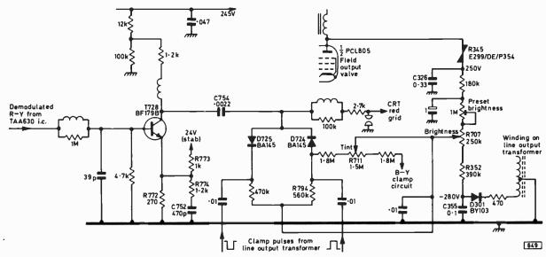
Fig. 3: Circuit of the R-Y colour-difference output stage together with the brightness and tint control arrangements. Tube protection is afforded by deriving the brightness potential from the field output valve.
