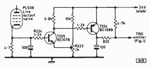
Fig. 2: The beam limiter circuit.
