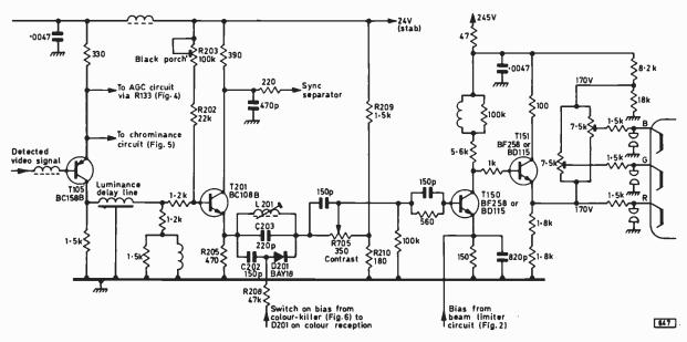
Fig. 1: Complete luminance channel circuit, which is d.c. coupled throughout.
