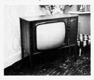
The Philips Model G25K500, a 25in. receiver fitted with the G6 dual-standard colour chassis.
