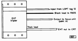
Fig. 3: Connections to the e.h.t. tripler.
