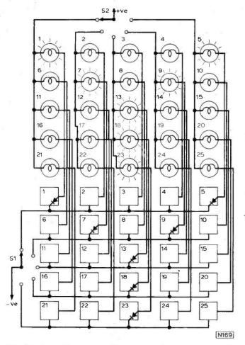
Fig. 33: Principle of operation of the character ROM. The letter Y is being generated on a  $5 \times 5$  matrix.
