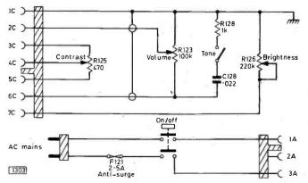
Fig. 1: Mains input arrangement and connections to the main controls.
