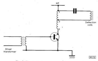
Fig. 2: The basic line output transformer circuit.
