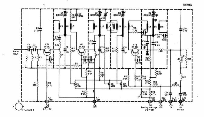
4 L18 + L17 L16 R5 Rn (R13) C17 4 10 78 Ч 9 0 c160 Fig. 1 (top) and Fig. 2 show the circuit and Make output connection layout of the ELC1043. L20 Juununin Components to be here removed are marked with an asterisk. N168
