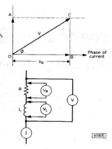
Fig. 15: Relative phase of current and voltages across the various parts of a circuit containing resistance and inductance.
