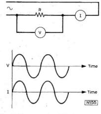
Fig. 5: Phase relationship of current and voltage in a circuit containing pure resistance only.
