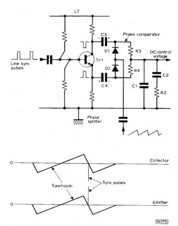
Fig. 5: A simple flywheel phase comparator circuit with pulse timings at the transistor collector and emitter.
