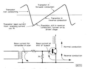
Fig. 3: Current flow in a line output transistor.
