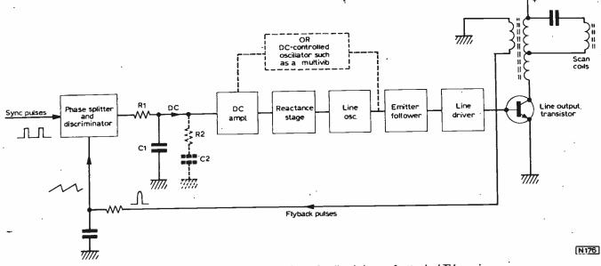
Fig. 6: Complete flywheel line timebase feedback loop of a typical TV receiver.
