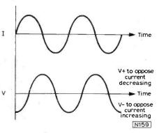
Fig. 9: Relative phase of the current and induced e.m.f. in an inductor.
