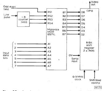
Fig. 35: A character generator using the Motorola MCM6571L.
