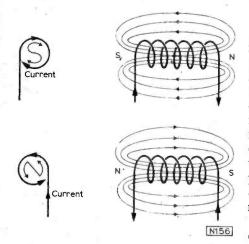
Fig. 6: Magnetic fields around an inductor. (Conventional current flow).
