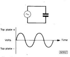
Fig. 12: An alternating voltage applied to a capicitor produces an alternating charge between the plates.
