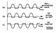
Fig. 3: For a wave which is not symmetrical, 180° phase shift is NOT the same as inversion.
