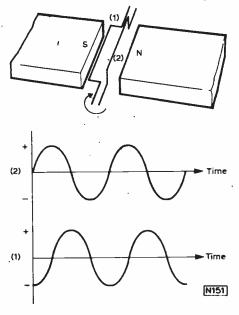
Fig. 1: Two loops rotating 90° apart will produce two sinewaves separated by 1 cycle, a phase shift of 90°.
