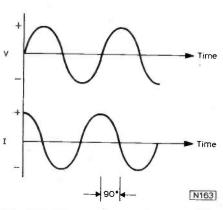
Fig. 13: The current peaks occur 90° earlier (to the left) of the voltage peaks in a capacitor.
