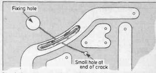
Fig. 4: Board cracks often radiate from a fixing hole and break nearby tracks. Repair with a wire bridge and drill a small hole at the end of the crack to prevent it spreading.
