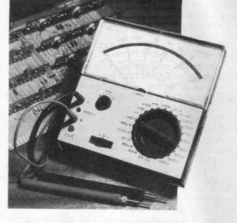
Six decade resistance ranges are provided with mid scale readings of  $5\Omega$  to  $500k\Omega$ . The range of measurements is from  $0.05\Omega$  to  $50M\Omega$ . It is unusual to find the two low resistance ranges on an instrument of this type but they are very useful when making up low value resistors from resistance wire (e.g. Power amplifier emitter resistors), or for measuring the resistance of connecting leads.
