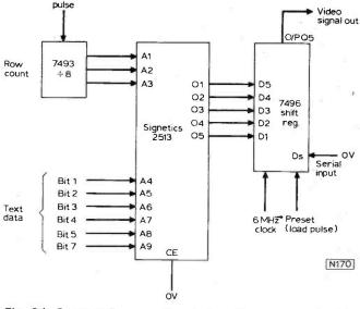
Fig. 34: System diagram of a character generator using the Signetics 2513 ROM.
