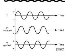
Fig. 10: Relative phase of the current, induced voltage and applied voltage in an inductor. Now consider the phase diagrams for an inductor, Fig. 10.
