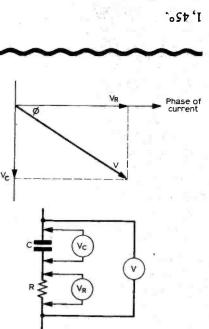
Fig. 16: Relative phase of current and voltages in a CR circuit.
