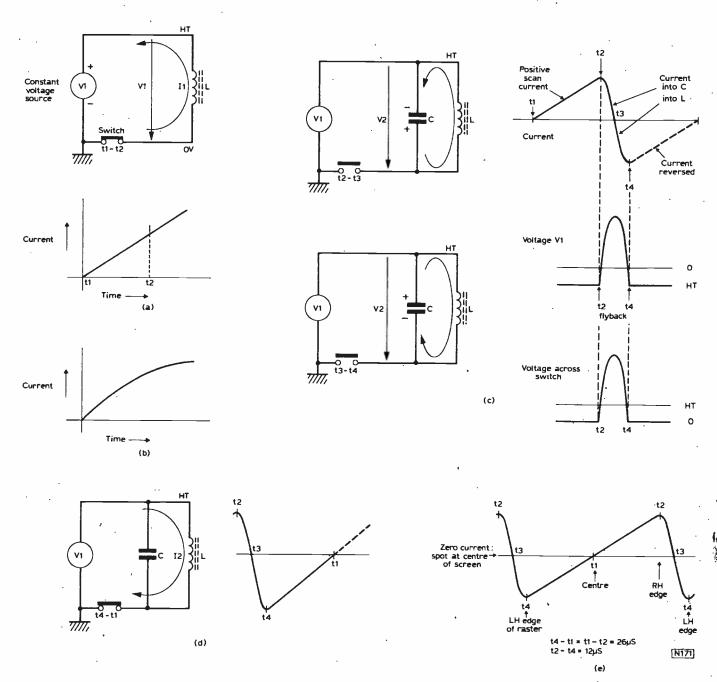
Fig. 1: A Switchable constant voltage applied across the inductance of the line scanning yoke produces a sawtooth scan current and a high voltage pulse. (a) The switch closes at instant t1 to produce the rising current sawtooth. (b) Losses cause the sawtooth to become nonlinear. (c) The flyback cycle is in two parts. (d) The first part of the scan is a decreasing current sawtooth. (e) The complete scan cycle.
