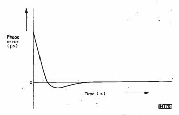
Fig. 8: For VTR operation, the shorter filter time-constant reduces settling time to about 5 lines in a well-designed circuit.
