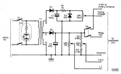
Fig. 3: Circuit diagram of the Power and Control Unit.
