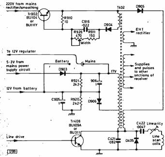
Fig. 1: Switch-mode power supply/line output circuit used in several mains-battery portable models.
