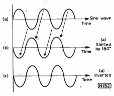
Fig. 2: Phase shifting a sinewave by 180° produces the same effect as inversion.
