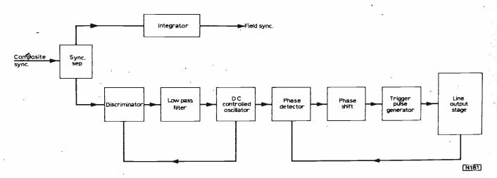
Fig. 11: Block diagram of a typical combined sync separator and flywheel line oscillator i.c. A second phase-controlled loop ensures correct phasing of the line output stage despite changes caused by variations in transformer loading and circuit tolerances.
