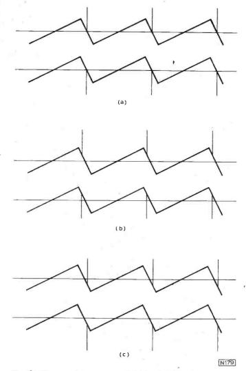
Fig. 9: Changes in waveforms of Fig. 5 with timing errors: (a) Oscillator frequency correct – no d.c. control voltage. (b) Oscillator frequency too low – positive d.c. output. (c) Oscillator frequency too high – negative d.c. output.
