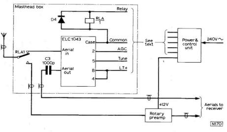
Fig. 4: Internal wiring of the masthead unit and general system connections.
