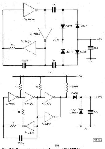
Fig. 36: Generating supplies for the MCM6571L.
