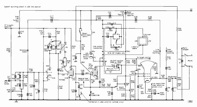
Fig. 1: Line timebase and c.r.t. circuit, STC VC52 chassis. The same basic circuit with only minor component value changes was used from the VC2 chassis on. In earlier chassis the arrangement of S11 is slightly different and the S-correction capacitor C130 is 0.0022µF (3kV).
