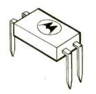
The Motorola  $\frac{1}{4}$ -Watt Audio Amplifier is designed for the output stage of battery powered portable radios.
