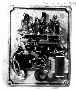
Internal view of the prototype preamplifier.
