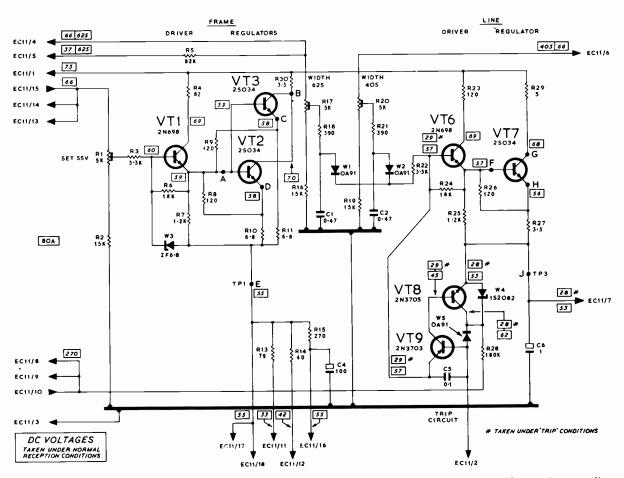
Fig. 7: Power supply regulator circuits.
