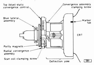
Fig. 1: General arrangement of the tube neck components using the AT1022 type deflection yoke. Note that on this series the marker tab is red: on AT1027 and AT1029 assemblies with convergence "rider" units (see text) the tab is blue.
