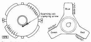
Fig. 4 (left): Connection numbering and interconnections required for all deflection units. Interconnections to be made: field, 5 to 4, 5' to 4', 3 to 6' and 6 to 3', with input from 4F on the timebase panel to 3 and return from 3' and 6 to R427 on the convergence panel at 5M and 5N (see Fig. 3, page 17, November issue); line, 1 to 2, with input to 1 from 5B and return from 2' and 1' to L402 via 5D and 5C on convergence board.
