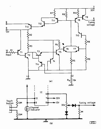
Fig. 3: (a) One of the switch channels of the Siemens SAS560/SAS570 bipolar touch-tuning i.c. series. (b) External connections to the i.c.
