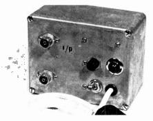
The prototype is housed in an Eddystone diecast box.
