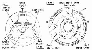
Fig. 2 (left): Rear view of the AT1023 type radial convergence assembly mounted on the tube neck with the blue lateral assembly also shown.
