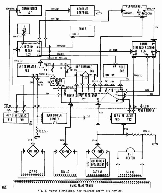
VT6 going short-circuit. The latter causes a small picture with sky-high e.h.t. Unadjustable e.h.t. can be due to a faulty W1. C2 and C8 can explode with no apparent reason.
