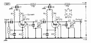
Fig. 1: Circuit diagram of the basic preamplifier. See also modification mentioned in text.
