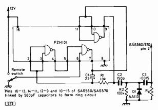
Fig. 4: Use of an FZH101 i.c. as a clock pulse generator to apply remote control to the Siemens touch-tuning i.c.s.
