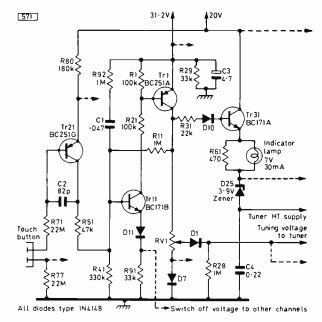
Fig. 2: Circuit of one of the six touch-button controlled switch channels in the tuner control unit used with the ITT CVC7 chassis (fitted in the KB Feathertouch 100 colour receiver).
