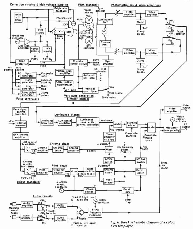
is preamplified before being fed to the track selector switch. As with the video section of this switch three possible output combinations are possible—track A sound, track B sound or colour. In positions A or B the output from the switch is fed through a further stage of audio amplification and the resultant is available either as an audio output for supplying extra amplifiers and loudspeakers or as
