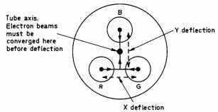
Fig. 2: Triangular arrangement of the three guns in the shadowmask tube, showing how X and Y deflections (convergence) have to be made to position the beams correctly on the axis of the tube before scanning.
