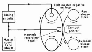
Fig. 3: High-speed EVR printer arrangement.
