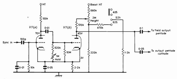
Fig. 1: Field generator circuit of the Bush Model TV115L. System switch S2h slightly reduces the right-hand triode anode voltage on 625 lines to equalise height. Fault symptoms were greatly reduced height and completely folded-over picture.
