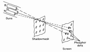
Fig. 1: Schematic of the shadowmask tube. The spacings have been distorted for clarity. In reality the guns are some 10-12in. from the screen, the shadowmask is about \( \frac{1}{2} \) in. from the screen, and the electron beams cover about three holesin the mask.
