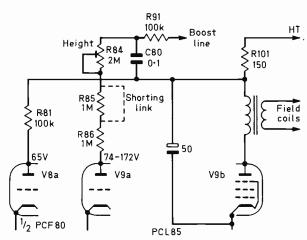
Fig. 2: Anode h.t. supplies in the RGD Model 628 field circuit. Height on this receiver had suddenly reduced to about half due to severe reduction of V9a anode voltage.
