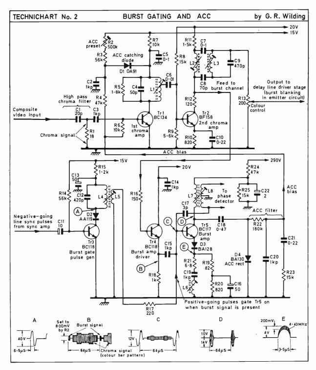
is in these models undertaken in the colour-difference preamplifier stages. Secondly instead of burst blanking—removing the burst signal from the chroma signal—being undertaken in the chroma circuits it is undertaken in the following delay line driver stage—by feeding positive-going pulses to its emitter so that it is switched off during the burst signal period, (the delay line driver, being an npn transistor, will be
