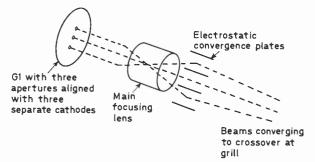
Fig. 9: Schematic of the Trinitron gun structure. The electron beams are converged within the tube with one very wide-aperture lens.
