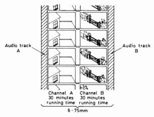
Fig. 1: Layout of monochrome EVR film. A one-hour cartridge has some 180,000 frames each of which can be studied individually.
