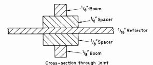
Fig. 2: Reflector assembly.
