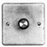
This is an attractive dimmer unit which fits in place of the normal modern light switch. The ivory mounting plate matches modern fittings and the control knob is bright chrome. An ON/OFF switch is incorporated to control 40-600 watts of all lights except fluorescents at mains voltages from 200-250V, 50 Hz.
