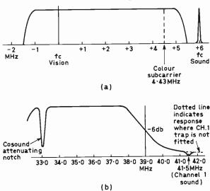
Fig. 1: (a) Transmission spectrum of a 625-line transmitter. (b) Response curve of an i.f. strip, using intercarrier sound, to handle the above transmitter spectrum. Note that the sense of the vision and sound signal is reversed at i.f. as the tuner's local oscillator operates above the channel frequency.
