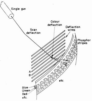
Fig. 3: Principle of the beam deflection type of tube. The chromatron is an example of this type of tube. The electron beam from a single gun lands on a green stripe if undeflected; if wire A is positive and wire B negative it lands on a blue stripe; if wire A is negative and B positive it lands on a red stripe.
