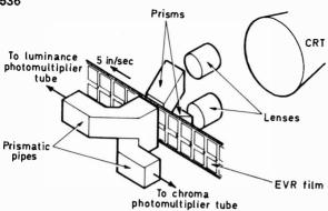
Fig. 5: Optical system in an EVR teleplayer.
