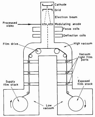
Fig. 2: Electron-beam recorder.
