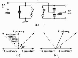
Fig. 3: (a) R.F. equivalent circuit of the latio detector tuned circuits. (b) Relationship of voltages at resonance. (c) When the sound carrier frequency deviates the 90° phase relationship of (b) no longer applies and the resultant vectors are of unequal length: one detector diode therefore conducts more heavily than the other.
