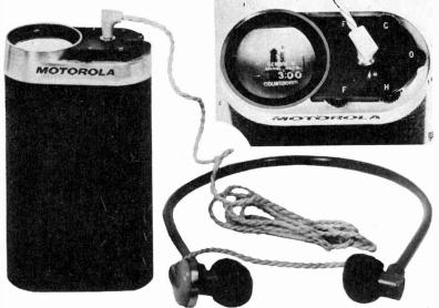
picture tube, power supply and batteries, the actual receiver circuits taking up only one cubic inch. Altogether 43 Motorola transistors and diodes are employed in the receiver which is at present designed for single channel operation. The set has a 3-transistor tuner, 3-stage i.f. amplifier, 2-stage video amplifier, ratio-detector type intercarrier sound demodulator and automatic gain control.
