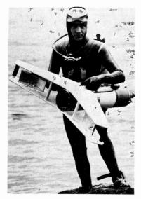
Group 70 Limited of Manchester have developed, in conjunction with Marconi Marine Limited, a new underwater combined camera and lighting unit.
