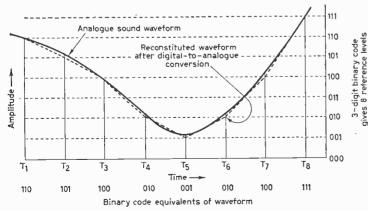
Fig. 1: Basic principle of sampling a sound waveform and converting the samples into binary form.
