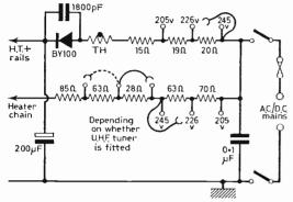
Fig. 1: Unconventional connection of the thermistor in the h.t rectifier surge limiter circuit instead of in the heater chain in the GEC 2000DS series.
