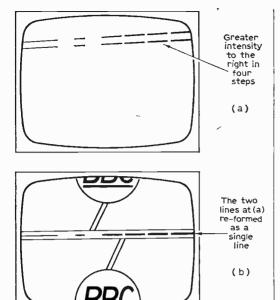
Fig. 4: Slow field retrace will show the BBC test pulses at the top of the picture as at (a). They are normally present between fields as at (b).
