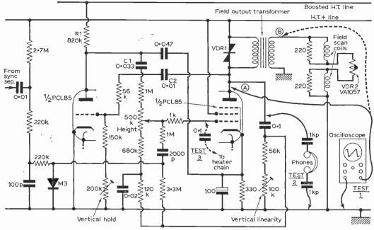
Fig. 2: The widely used PCL85 field generator/output circuit, showing basic tests.
