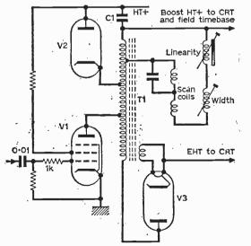
Fig. 1: Typical line output stage. VI line output pentode, V2 efficiency or boost diode, V3 e.h.t. rectifier. T1 is the output transformer and C1 the boost reservoir capacitor.
