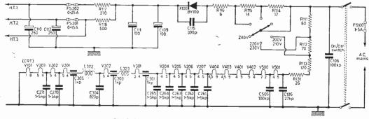
Fig. 6: Circuit of the h.t. supplies and heater chain.
