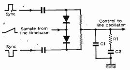
Fig. 3: A simple type of flywheel line sync discriminator; C1, R1, C2 are the flywheel components.
