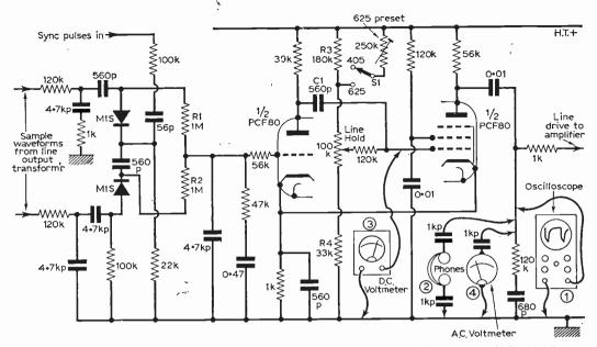
Fig. 1: Basic tests to make in the I ne oscillator stage. The stage shown uses a cathode-coupled multivibrator with flywheel line sync.
