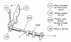
C326 is the stationary member in which the core moves. Adjust and unscrew at X.
