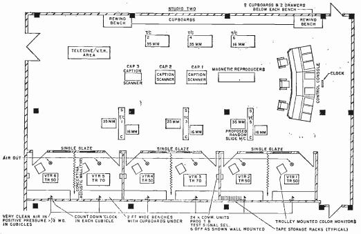
Fig. 1: Yorkshire Television's central apparatus room, showing the layout of the telecine/videotape area. At the top, three flying-spot telecine units, at the bottom of the main room three lead-oxide film chains, and between the caption scanners and tape reproducers. The videotape machines are arranged in pairs in the three booths: with the concertina doors open the pairs can be used for electronic editing.
