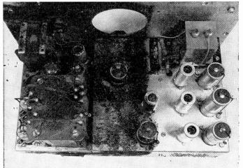
HE above photograph, sent to us by Dawe Instruments Ltd., shows how a chassis has been cleaned by one of their ultrasonic cleaning machines.
