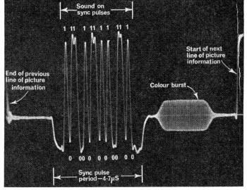
Fig. 2: BBC sound-in-vision signal. Two ten-digit binary signals are inserted in each sync pulse period. The pulses here read 1011001011010011010.
