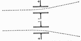
Fig. 1: The principle of electrostatic deflection. A beam of electrons is attracted by a positive potential and repelled by a negative one.
