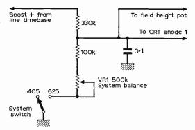
Fig. 2: Method of balancing the boost voltage on the two systems.
