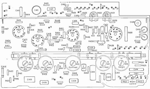
Fig. 4: Layout of the timebase printed board, viewed from the component side.
