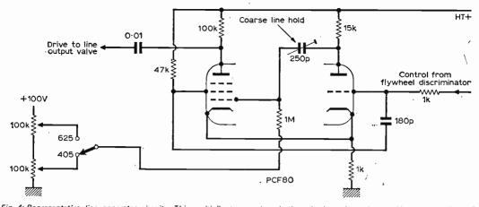
Fig. 4: Representative line generator circuit. This multivibrator employs both cathode and anode-to-grid cross-coupling. To reduce the load on the oscillator, feedback to the triode is from the screen grid instead of the anode of the pentode section of the valve.
