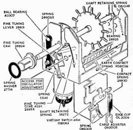
Fig. 4: Rotary tuner with fine manual tuning.
