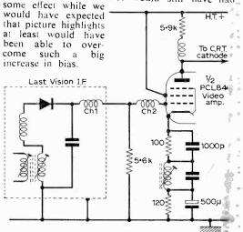
Fig. 2: Typical 405-only video circuit. The positive-going output from the diode detector produces an increased voltage at the video amplifier cathode as contrast is advanced. In one case of vision failing after 20 minutes coincident increase n this voltage indicated the probable cause.
