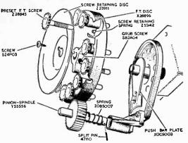
Fig. 3: Preset fine tuning mechanism.
