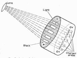
Fig. 2: Action of vidicon photoconductive layer.
