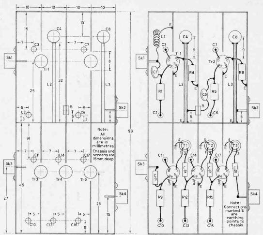
Fig. 5: Under-chassis layout and dimensions
