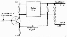
Fig. 13: Chrominance matrixing in the decoder to separate the B-Y and R-Y signals.
