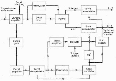
Fig. 14: Block diagram of a PALd decoder.
