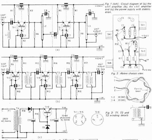
oscilloscope direct gain measurements at different frequencies can be made. The prototype amplifier was tested in this way (see Fig. 3). An indication of gain can however be obtained much more simply. Switch on a television receiver and if possible disconnect its a.g.c. line. Turn down the contrast control until the contrast is *just* out of the limiting condition. Plug the appropriate section of the amplifier into the aerial lead and observe the increased signal strength.
