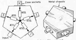
Fig. 7 : Four-way resistive splitter network.
