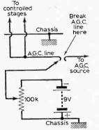
Fig. 4 (left):-It is possible to cut the a.g.c. line as shown and adjust the bias on the controlled valves by means of a potentiometer connected across a battery. Take care to observe the correct polarity or the controlled valves will be fed with a positive bias instead of the correct negative bias.
