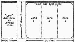
Fig. 7: Scanning zones. Raising the definition from "low" by three simultaneous transmissions of 30-line scanning.
