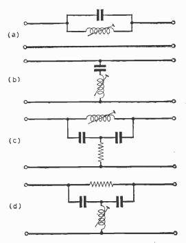
Fig. 11: Typical wavetraps used in television receiver i.f. circuits: (a) series rejector, (b) parallel acceptor, (c) and (d) bridged-T rejectors. Bridged-T filters give a much higher degree of attenuation and a more sharply tuned response than simple acceptor or rejector circuits.
