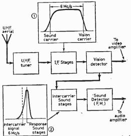
Fig. 4: Simple block diagram of a 625-line standard receiver, showing responses and signals.
