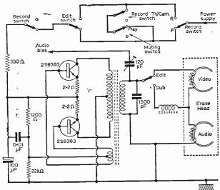
the audio erase head. In practice, of course, this is a single construction head, with dual windings and gaps appropriately positioned. (Easily said, but the problem of adjacent, interacting magnetic fields posed some ticklish engineering problems before this EF69-2102 head was brought into production, I am told.)
