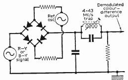
Fig. 10: A synchronous demodulator circuit in wide use. The series diode bridge detector.
