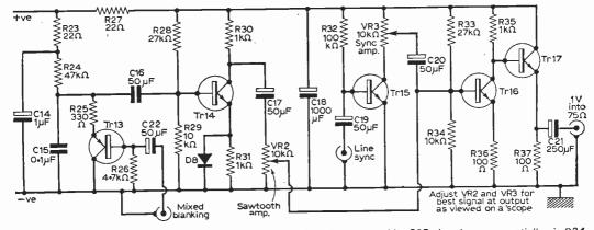
Fig. 6: The sawtooth pattern generator. The sawtooth waveform is generated by C15 charging exponentially via R24 and discharging when shorted by Tr13 being switched hard on. Tr14 acts as a linear amplifier.
