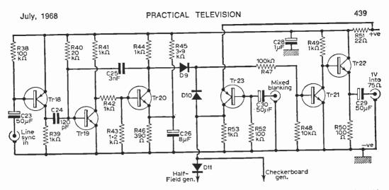
Fig. 7: The half-line generator. Tr18 inverts the input sync pulses which are used to trigger the monostable multivibrator Tr19, Tr20. The output is fed via D9 to the inverter Tr21 and emitter-follower output transistor Tr22, and via D10 to the checkerboard pattern generator to be described next month. The blanking pulses are also fed to the output to the checkerboard generator via Tr23.
