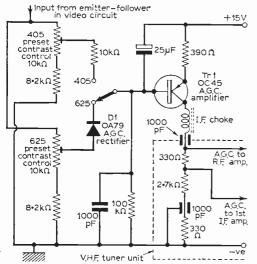
Fig. 2: A.G.C. circuit used in Bush-Murphy models with diode peak detector and p-n-p a.g.c. amplifier.
