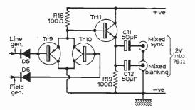
Fig. 4: The sync mixer. Tr9 and Tr10 form an or gate which drives the emitter-follower output stage Tr11.
