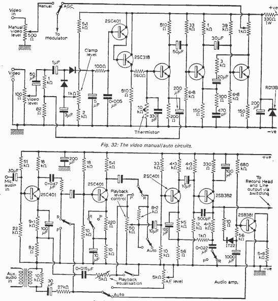
Fig. 33: The audio manual/auto circuits.
