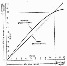
Fig. 2: Practical transfer characteristic (full line) compared with the ideal (broken line). Note increase in curvature outside the limits of the working range.
