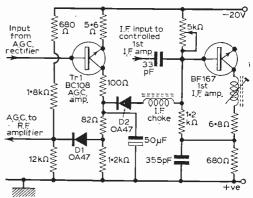
Fig. 3: Commonly used a.g.c. delay circuit providing independent control of the r.f. and i.f. stages.
