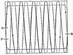
Fig. 13: Sinewave scan. This multiple interlace starts at S and then returns from R to finish at F. Continuing, the trace fills the screen without flicker or visible "structure".
