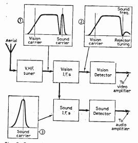
Fig. 3: Simple block diagram of a 405-line standard receiver, showing responses and signals.
