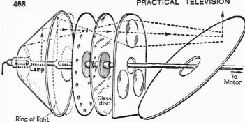
Fig. 10: Cone reflector for multi-scan: annular projection with apertured disc, bushed glass plate and circle of lenses.
