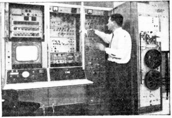
Telecine Room: In the centre, the Rank Cintel-35mm. flying-spot scanner; on the right the Westrex 35mm. double-head playback machine; on the left the Goldring Lenco disc player (on the stand) and mounted in the cabinets, two Armstrong AM/FM radio tuners, a  $\lambda$ -inch Ferrograph sound tape recorder and off-air television tuners, modulators and amplifiers.
