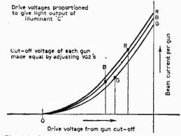
Fig. 11: Operating the c.r.t. for correct grey-scale tracking.
