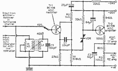
Fig. 1: A.G.C. circuit using a peak datector (Tr1) operating in the 625-line mode on the sync tips and an a.g.c. amplifier stage (Tr2).
