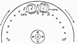
Fig. 8: Camera-receiver disc. Two lenses and two frames: for camera C, for receiver R. For 30-lines: 32 apertures.
