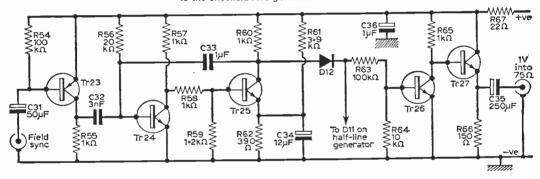
Fig. 8: The half-field generator. The same type of circuit as the half-line generator is used, with the value of the timeconstant cross-coupling capacitor altered to give the required pulse repetition frequency.
