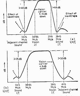
Fig. 14: Overall i.f. response curves for the circuits shown in Fig. 12, (a) on v.h.f. and (b) on u.h.f.
