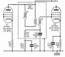
Fig. 15: Vision i.f. circuit overload protection. Should excessive inputs drive V2 into grid current R4, C1 develop additional self-bias to add to the bias provided by R5. V1 has a.g.c. applied to it R1 being left unbypassed to offset variations in input capacitance caused by a.g.c. variations.
