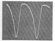
Fig. 3: This exponential drive waveform is obtained by the charging of a capacitor through a resistor and its sudden discharging through a-low resistance circuit.
