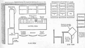
apparatus bays should be fitted with covers that duct heated air to the rear. Monitors, too, suffer from overheating and the positioning and spacing the monitor stack is important in this respect. A window-mounted ventilator with its wide range of adjustment could provide sufficient draught-free ventilation for most applications but in extreme cases strategically placed fans may be required. In a van, a fan heater will give both heat and cooling as required.
