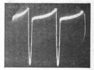
Fig. 5: The waveform at the line output stage when the Y lead is oosely coupled to the insulation of the lead to the anode of the line output valve.
