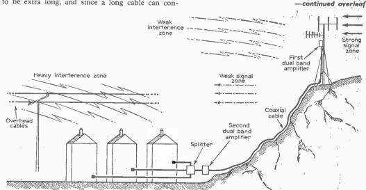
Fig. 1—Example of a hill-mounted aerial to improve the signal interference ratio. By the use of amplifiers and a splitter a number of viewers may be fed from the one aerial, thereby reducing costs. The masthead amplifier could be powered from a small unit at the set end of the coaxial cable; using the cable to feed power to the amplifier as well as to feed signal to the sets.
