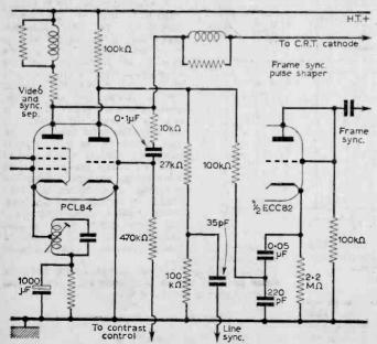
Fig. 27—McMichael MP18, etc., video, sync separator and frame pulse shaper circuit.
