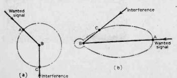
Fig. 2—An omnidirectional aerial at (a) gives response to interference equal to that of the required signal. B-C equals B-A. A directional aerial, however, can be orientated for the best ratio between the signal and the interference. Here the response B-A is greater than the response B-C.
