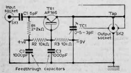
Fig. 1—Circuit diagram of the u.h.f. preamplifier.
