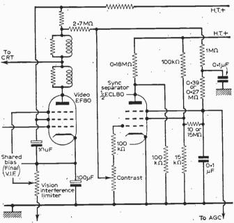
Fig. 29—Philips TG100U, etc. Video amplifier also acts as interference limiter and sync separator is used also as a form of a.g.c. clamp.
