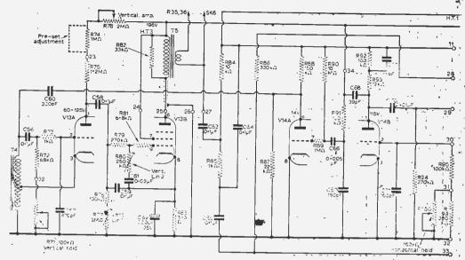
Fig. 5-Frame oscillator/output stage and line oscillator.
