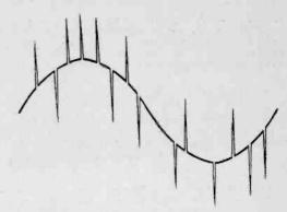
Fig. 3—Showing spikes of impulsive interference superimposed upon a signal waveform.
