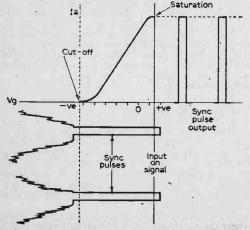
Fig. 24b—Vg/la curve for saturated pentode type of sync separator, with input as Fig. 24a. Polarity of applied signal is arranged to drive the valve rapidly from cut-off to saturation when the sync pulse arrives. Anode current drops rapidly again when the sync pulse ceases. Duration of sync pulse is approximately 10µS, occurring at 100µS intervals,
