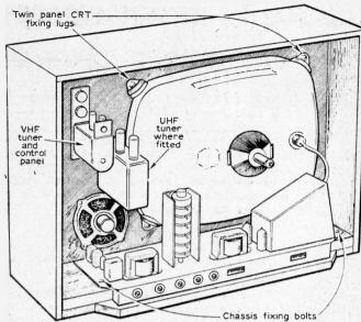
Fig. 2: Back view of the K-B Model WV20, showing location of major components.
