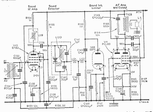
Fig. 3—All the components shown in this circuit section are dealt with in the text. The circuit is of the Ferguson 306T and 308T models and covers the sound l.F. stage, the sound detector, the sound interference limiter and the A.F. and output stages.
