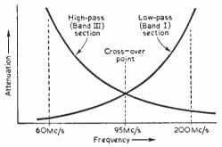
Fig. 10—The frequency and attenuation characteristics of a simple diplexer (or aerial cross-over network) of the kind shown in Fig. 9 last month.
