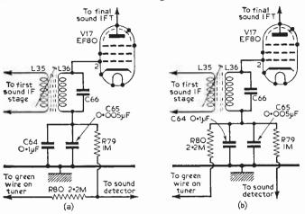
Fig. 3 (a)—The original circuit; (b)—the circuit after modification on the DM4 series to cure sound-on-vision.
