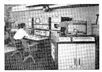
Much of the technical equipment at Border Television Ltd.'s new Television Centre at Carlisle has been supplied by EMI Electronics Ltd., who were also responsible for the wiring and installation of all the electronic equipment. This illustration shows the telecine suite where two switchable monitors have been installed.
