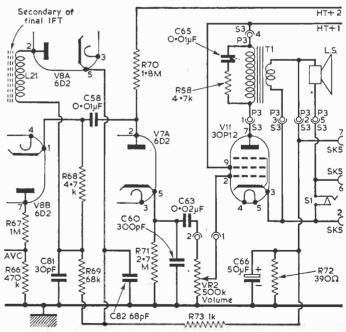
Fig. 4—The sound detector, limiter and output stages.
