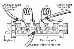
Fig. 11-The tag-board construction of a simple aerial cross-over network.
