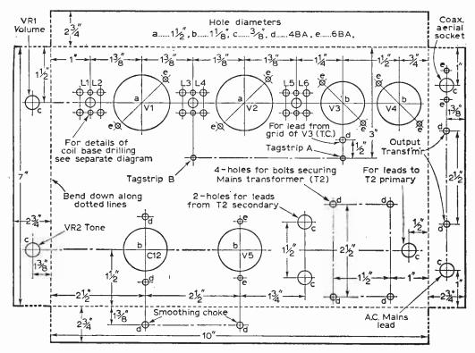
Fig. 2-The chassis drilling details.
