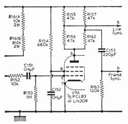
Fig. 4—This circuit modification, on the English Electric T40 series, will improve frame stability.
