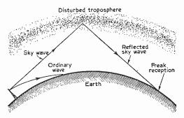
Fig. 5—Freak reception is caused by the long-range reflection of the wave by the troposphere. This happens when the state of the troposphere differs from normal and is generally associated with periods of fine weather.
