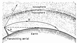
Fig. 1—The surface wave (A), the direct wave (B), and the sky wave (C). The latter wave is usually lost in space.
