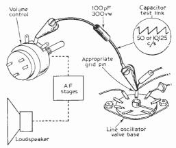
Fig. 4—A quick test to check that the line or frame oscillator is operating.
