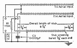
Fig. 2—Eliminating pattern interference on Band III.
