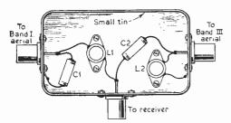
Fig. 12 (above)—An aerial cross-over unit, constructed in a small tobacco tin.
