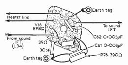
Fig. I—Modifying Decca DM4/C models to clear adjacent channel interference; (above) the component layout around the valvebase, after modification, (below left) the circuit before modification and (below right) after modification.
