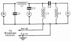
Fig. 14—By the addition of an inductor (L3) and a capacitor (C3) the television aerials can also serve the ordinary broadcast receiver to advantage.
