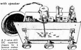
Long and medium wave. With cord and drum reduction tuning drive and illuminated glass dial (size 6½ x.2½in.). Controls: Volume on/off, tuning and wave change. The receiver is self-powered, employing a mains dropper and a valve rectifier. Size 6½ x 9 x 5½in. high. Complete with 5-inch speaker, valves (UCH42, UAF42, UL41, UY41), mains lead, ivory knobs, etc. ONLY \$4.19.6 P. & P. 6/6.
