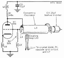
Fig. 5—The coaxial lines oscillator.
