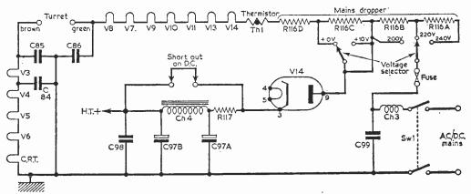
Fig. 8—The power supply circuits of a typical receiver, showing also the heater chain.
