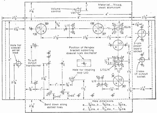
Fig. 3—The drilling details of the chassis.
