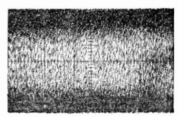
Fig. I—A picture of noise taken from the screen of an oscilloscope.
