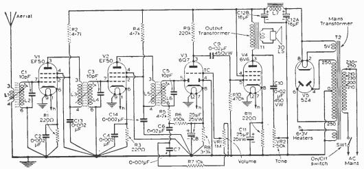
Fig. I—The complete circuit diagram.
