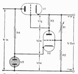
Fig. 1.—The basic circuit of a variable voltage stabilised power supply.
