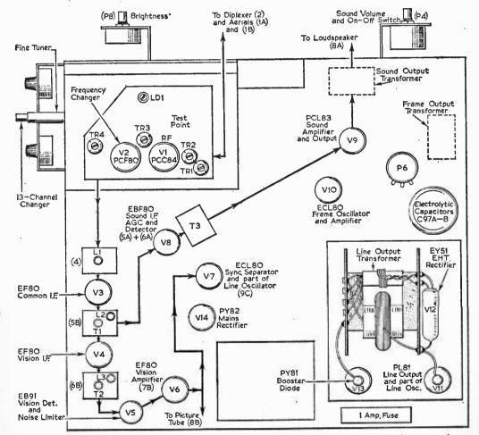
Fig. 2.—The above-chassis view of a typical receiver showing the various stages and signal paths in accordance with the block diagram in Fig. 1.
