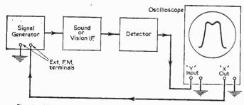
Fig. 4.—Using an oscilloscope with a signal generator to display the I.F. response curve.
