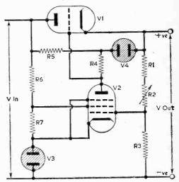
is an EL37 tetrode with its anode and screen connected together as a triode. Fig. 3 shows the characteristics of this valve, and from these characteristics it can be seen that with the grid voltage at -2V and the anode current at 50mA, the anode voltage is about 115V. The transformer/ rectifier unit must therefore provide a voltage equal to the voltage of 300V, when 50mA is being delivered to the load, and when the mains voltage it as its minimum. This fixes point (B) at 415V (Fig. 2).
