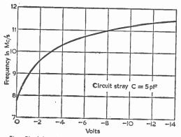
Fig. 2b (above).—Variation of the frequency with applied voltage of the SVCI. Below: Curve from a VHF transistor portable.
