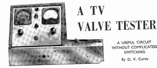
HIS TV valve tester was built up mainly of surplus components and enables a large range of common valves to be tested for mutual conductance and behaviour under various working conditions. Nothing new is claimed for the circuit, indeed it is extremely simple (Fig. 1) with no multiplicity of switching, but almost any normal voltage or bias can be fed to the valve and voltage and anode current readings observed simultaneously.
