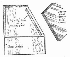
Fig. 2.-Construction of the case and front panel.
