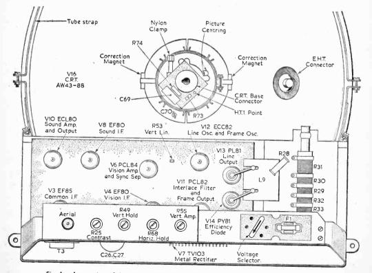
Fig. 1.- A rear view of the receiver showing the positions of some of the larger components.
