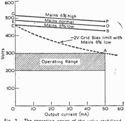
Fig. 2.—The operating range of the valve stabilised power supply.
