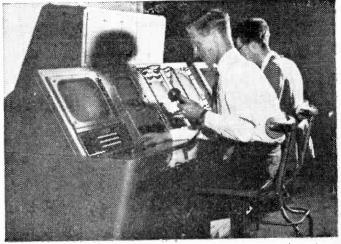
This Tabular Display unit and combined Radar/Synthetic Display unit, made by Marconi, will be shown at the S.B.A.C. exhibition in the near future. Of special interest is the closed circuit television screen, which is used to give an updated display of meteorological information.
