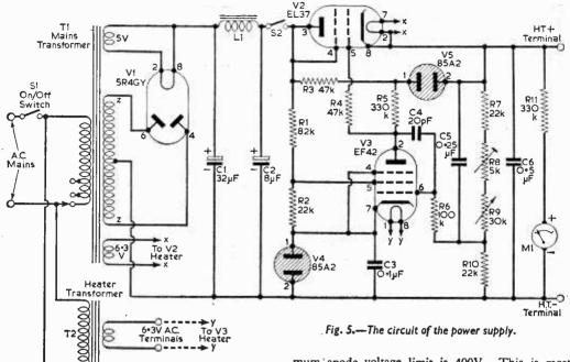
Two other points are important as far as V1 is concerned. One is that the maximum anode voltage of V1 should not be exceeded, and the other is that the maximum anode plus screen dissipation of V1 should not be exceeded. For the EL37 the maxi-
