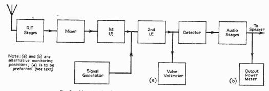
Fig. 3.—How the signal generator is used to align the I.F. amplifier.
