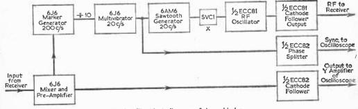
Fig. 1.—The block diagram of the wobbulator.
