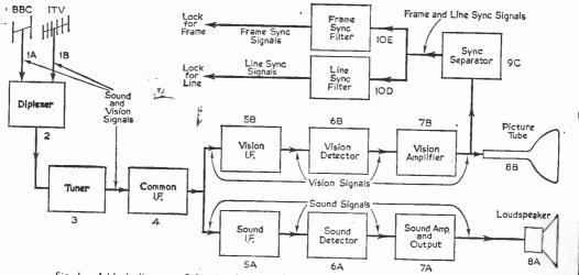
Fig. 1.—A block diagram of the signal stages of a television receiver showing the signal paths.
