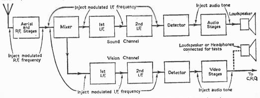
Fig. 1.—Using a signal generator to test for breaks in the sound and vision channels.
