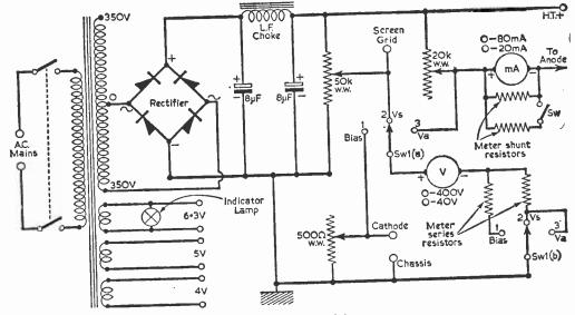
Fig. 1 .- The basic circuit of the tester.
