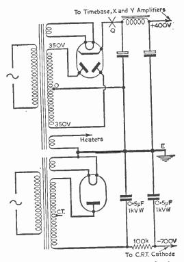
Fig. 16 .- The circuit of the power supplies for the oscilloscope.
