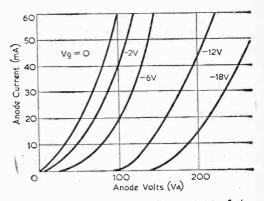
Fig. 3 (above).—The Ia/Va characteristics of the EL37 triode-connected.
