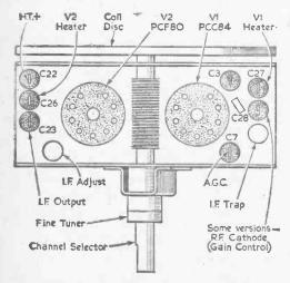
Fig. 1.—The top view of the original Fireball tuner. The shaded components are lead-through decoupling capacitors.
