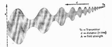
Fig. 1.—The well known representation of an amplitude modulated carrier wave.
