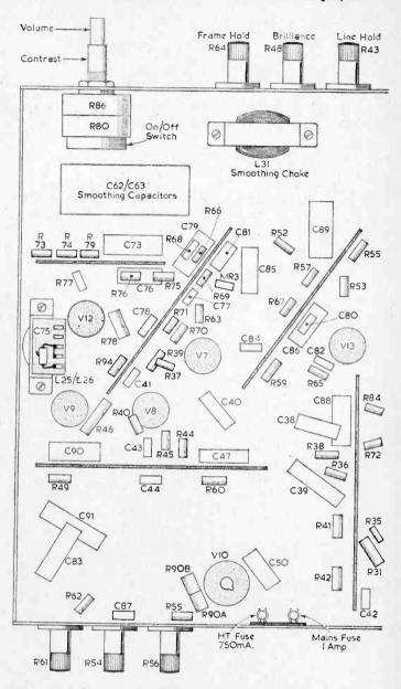
Fig. 6.—The underchassis view of the receiver.
