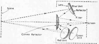
Fig. 10.—Colour focus camera; the focused scene is analysed into three primaries and combined on the screen. The colour units are optical "sandwiches" of lens, filter and reflector. The convex reflector collects and registers the coloured rays.
