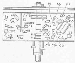
Fig. 2.—The underchassis view of the first Fireball.
