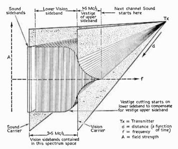
Fig. 3.—A "picture" of a television channel with equal vision/sound power ratio.
