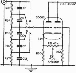
Fig. 12.—The input attenuator and cathode-follower input to the Y-amplifier. R30 and R32 are equal in value (2.2k) and should be matched.
