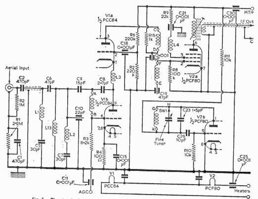
Fig. 5.—The circuit of the unit used in recent Sobell and McMichael television receivers.
