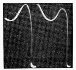
The oscilloscope trace of a screen pulse (for fly-back blanking) :f=100kc/s.
