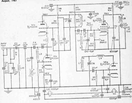
Fig. 3 .- The circuit of the tuner.
