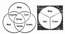
Fig. 7 (left).—Additive colour primaries superposed to show the formation of white and three complementary colours.
