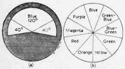
Fig. 9.—A nine-colour wheel. Three primary images are superposed to form the wheel on the screen. One positive mask is shown.
