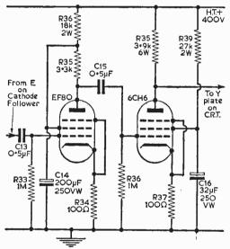
Fig. 13.—The Y-amplifier circuit: A.C. coupled only. The gain is about 800, and the bandwidth is approximately 3·4 Mc/s.
