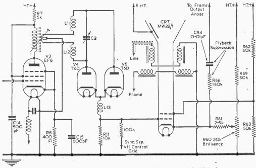
Fig. 1.—The final vision R.F. detector and CRT circuit of the receiver dealt with in the text.
