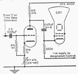
Fig. 10 (obove).—The cothode connection to the CRT, with flyback blanking.
