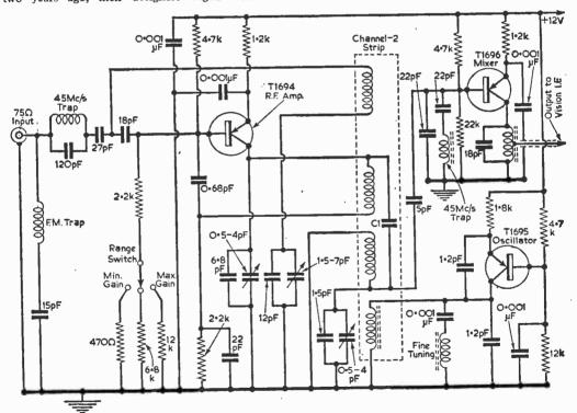
Fig. 1.—An early transistor tuner, designed by Philco.
