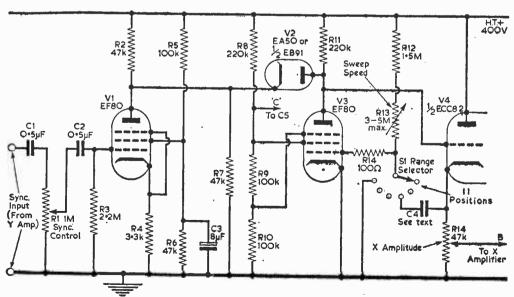
Fig. 9.—The circuit of the Timebase generator.
