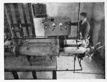
In this furnace at the new Griffiths Electronic Guns, Ltd. factory in Eire, all the stainless steel parts of the electronic guns are hydrogen fired.
