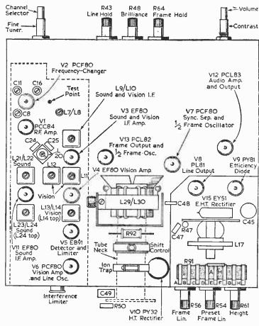
Fig. 5.—Plan view of the chassis.
