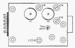
Fig. 1.—The above-chassis layout of the tuner unit.
