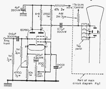
Fig. 4.—The circuit of a suitable Y-amplifier.
