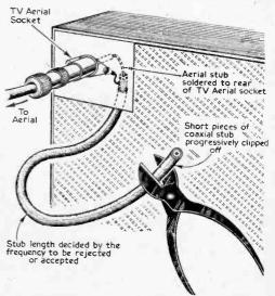
Fig. 2.—A method of adjusting an aerial stub.
