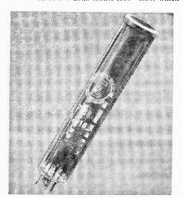
The 7038 Vidicon television pick-up tube which has recently been introduced by the English Electric Valve Co. Ltd.
