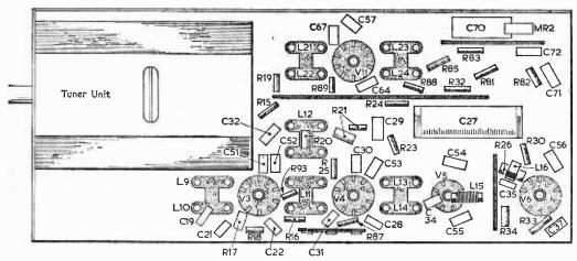
Fig. 4.—The under-chassis layout of the I.F. section.
