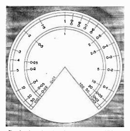
Fig. 6.—Assuming that the potentiometer, VRI, is linear, the calibrations on the scale should be similar to this.
