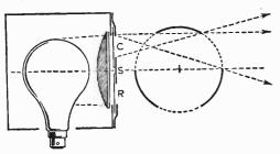
Fig. 3.—A two-colour projector with filters (C: cyan; R: red) in a frame with a strip S and a rotary shutter.
