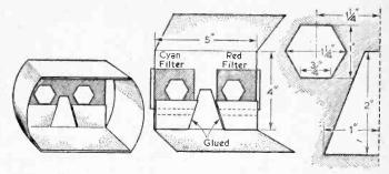
Fig. 1.—A binocular-type viewer with two colour filters—dimensions of the apertures are given on the right.
