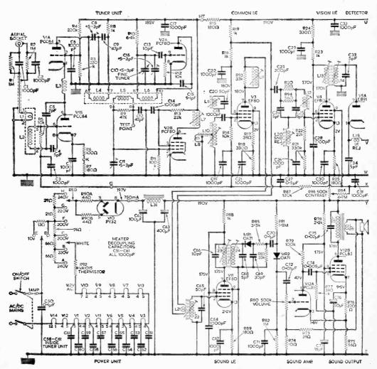
gain by disconnecting pin 9 from the AGC line and connecting it to chassis (6) or cathode (1 and 3). As the circuit stands, pin 9 of V4 (suppressor grid) acts as a clamp diode to prevent the AGC line becoming positive. The lead to pin 9 may be connected to a crystal diode, say an OA71, the positive end of which may then be connected to chassis. Valve V4 will then work at full gain, but if the connection of pin 9 to pins 1 and 3 results in instability, connect pin 9 instead to chassis (pin 6).
