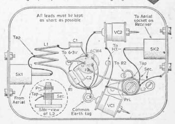
side of the chassis; see Fig. 3. If desired, the common earth tag may be soldered to the chassis for extra rigidity.
