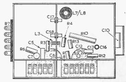
Fig. 2.—The under-chassis layout of the tuner unit.
