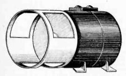
Fig. 4.—A rotary shutter driven by a small motor.
