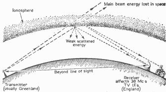
Fig. 13.—Sometimes interference is received from scatter propagation transmitters in remote countries.
