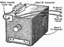
Fig. 3a. (above)— A normal Band III converter installation.
