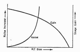
Fig. 1.—Naise from the R.F. valve rises steeply with increase in bias, while the stage gain fallows a gentle decline, as illustrated by the two curves above.
