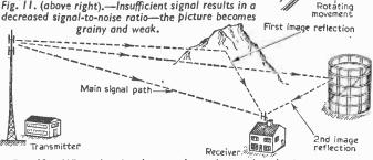
Fig. 12.—When the signal proceeds to the receiver by two or more different paths, the result is a succession of images on the screen—see Figs. 8 and 9, last month.
