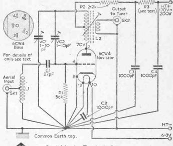
Fig. I (above).—The circuit diagram.
