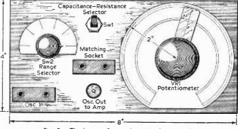
Fig. 3.—The layout of controls on the front panel.
