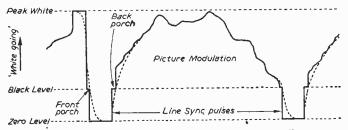
Fig. 1.—One line of a television signal between two line sync pulses. The dotted line shows the distortion of the theoretically ideal wave-shape which results from too great a rise-time in the amplifier.
