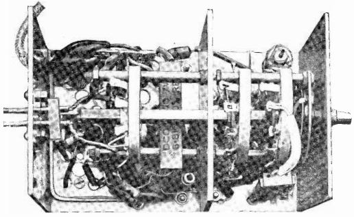
Underchassis wiring of the tuner.
