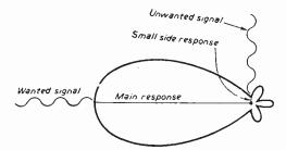
Fig. 8.—An aerial response pattern as shown may well be necessary to obtain maximum discrimination between the wanted and unwanted signals.
