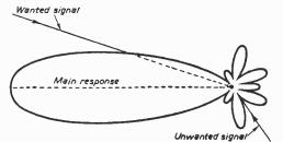
Fig. 11.—This diagram shows how the response to the wanted signal could be severely reduced if an aerial with a narrow forward lobe were orientated to reduce the response to an interfering signal coming in towards the rear. Nevertheless, an aerial with a narrow forward lobe may be required to reduce interference coming in from a variety of directions.
