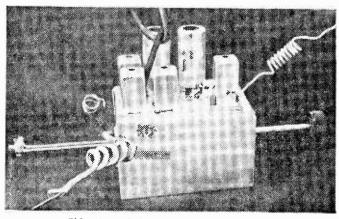
Side view of the completed tuner unit.
