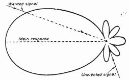
Fig. 10.—If there is one major interfering signal, an aerial with a relatively wide forward lobe may be orientated to give maximum rejection of the interfering signal without unduly affecting the pickup of the wanted signal.
