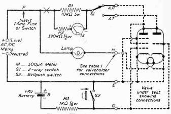
Fig. 2.---The circuit diagram.
