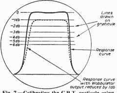
Fig. 7.—Calibrating the C.R.T. graticule using an attenuator.
