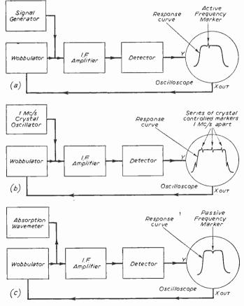
Fig. 6.-Three types of frequency marker.
