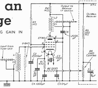
Fig. 1.-The circuit diagram.
