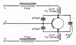
Fig. 8.-Motor suppressed for TV (Band III).
