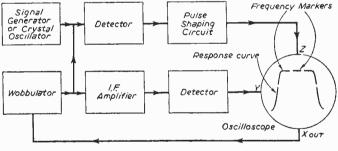
Fig. 9.—Using frequency markers to intensity-modulate the display oscilloscope.
