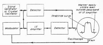
Fig. 8.—Producing markers that by-pass the equipment under test.
