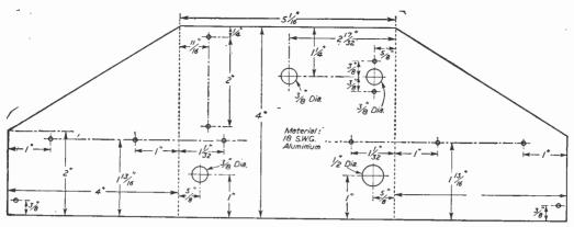
Fig. 6.—Case bending and drilling details.
