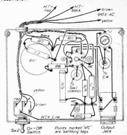
Fig. 4.—Underchassis wiring scheme.
