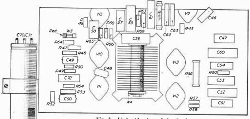
Fig. 3.—Underside view of the timebase and power unit.
