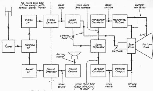
Fig. 2.—Sounds to be heard at various points in the circuit.
