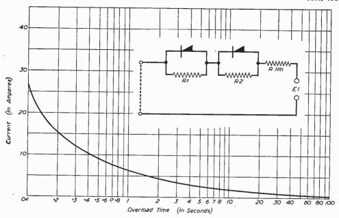
Fig. 3.—Typical curve giving overload current related to overload time. Fig. 4 (inset) Initial current surge when switching on the receiver is limited by the resistor Rlim in series with the rectifying system.
