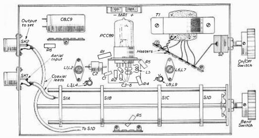
Fig. 3.—Layout of the pre-amp. (As the layout naturally depends to some extent on the parts employed, no detailed wiring has been given.)
