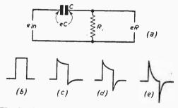
Fig. 2.—A basic differentiator circuit is shown at (a) and a line sync pulse at (b), while (c), (d) and (e) are the output waveforms for a time constant much larger than, equal to and smaller than the pulse duration.
