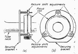
Fig. 1.— A method of focus-coil mounting.
