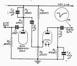
Fig. 6.—A frame pulse shaper circuit showing the waveform output at (a).
