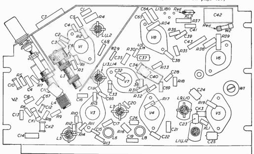
Fig. 4.—Underside view of the RF unit.
