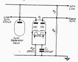
Fig. 7.—A frame pulse separator circuit.
