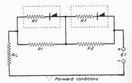
Fig. 2.—Forward conditions for two diodes in series.
