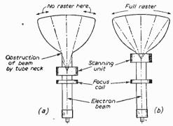
Fig. 2.—Showing how a wrongly positioned scanning unit can cause corner shadow.
