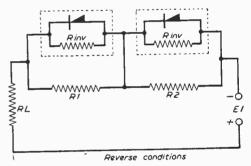
Fig. 1.—Reverse voltage conditions for two diodes in series. R1 and R2 are the equalising resistors.
