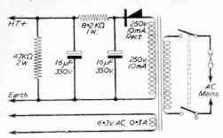
Fig. 3.-A mains power supply unit.
