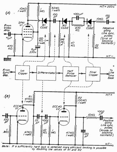
Fig. 2.—Two methods of line-pulse shaping.
