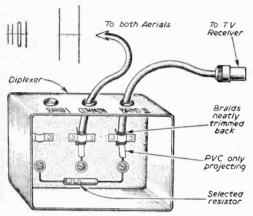
Fig. 1.—The necessary wiring.
