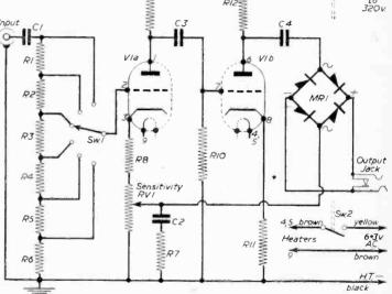
Fig. 1,-Circuit of the valve voltmeter.
