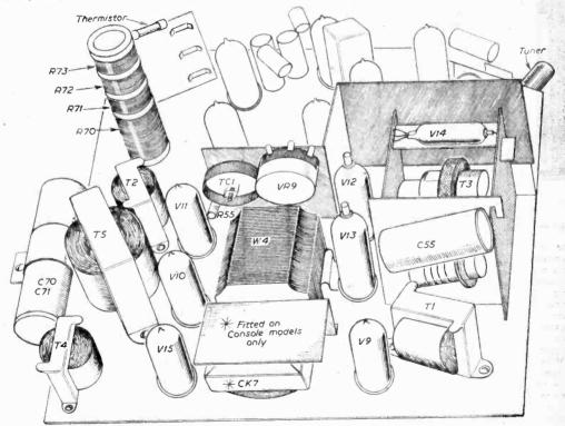
Fig. 1.—View of the timebase chassis.
