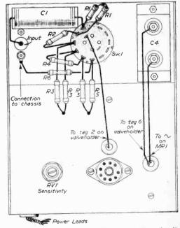
Fig. 5.—Above chassis and panel wiring details.
