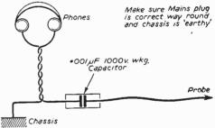
Fig. 1.—Using earphones with a condenser for signal tracing.
