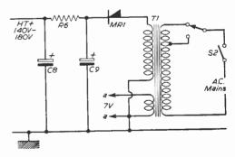
Fig. 2.—The circuit diagram of a simple power supply.
