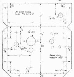
Fig. 2.—Chassis bending and drilling details.
