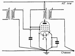
Fig. 3.—Single-point wiring is carried out as shown here.
