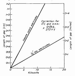
Fig. 10.—Spark gap lengths in air at 760 mm. Hg pressure and at 25 deg. C.
