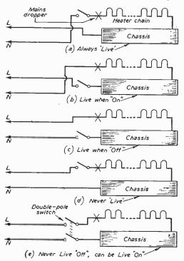
Fig. 1.--Results of various methods of connecting the mains.
