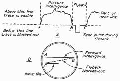
Fig. 3.-Waveform for one line.
