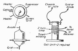
Fig. 2.-Coil and valve data. Note that the pin connections for the valve are only correct when it is viewed from the anode end.
