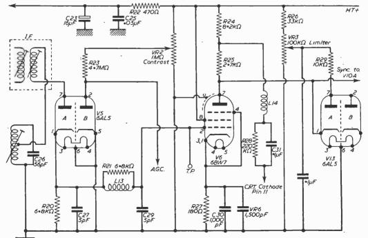
millin 3.3. 5. -- Vision detector, AGC diode, video amplifier, vision limiter and H.T. feed (via R22) to early stages.
