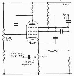
Fig. 52.—Miller transitron timebase.
