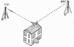
Fig. 2.—Yagi aerials are directional and must be pointed towards the transmitter.
