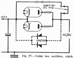
can be metal or valve types, in parallel.
