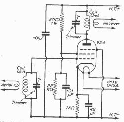
Fig. 1.—The circuit diagram. Power is obtained from the H.T. and L.T. supplies of the receiver.
