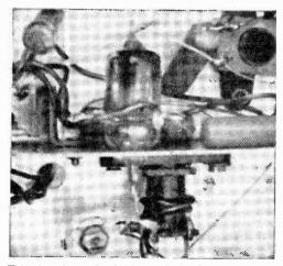
This view shows clearly the method of mounting the valve to protrude through the sub-chassis.
