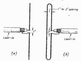
Fig. 1a (left).—The construction of a simple dipole. Fig. 1b (right).—The construction of a folded dipole.
