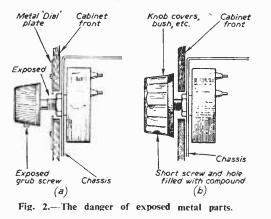
contact with the chassis, or wired to it. It is not unusual for danger to arise at the control knobs, especially in home constructed sets. A metal indicator or dial plate may be used, as shown at "a" in Fig. 2, and may be in contact with the birth or holding nut of a component. If no plates are used, a small knob, or long spindle, may allow the fingers to touch the spindle, bush.
