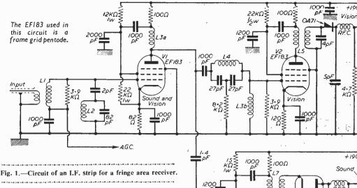
Band III, and a D.C. output of 2.0V peak white from the detector, the signal required at the aerial is  $63\mu V$  r.m.s. for the conventional receiver "A" but only  $11\mu V$  for the frame grid receiver "B."
