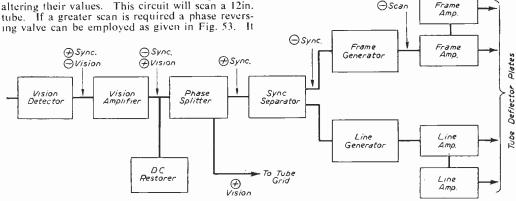
Fig. 51.-Block diagram of a receiver employing electrostatic deflection.
