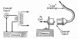
Fig. 3.-How the aerial connection may be "live".
