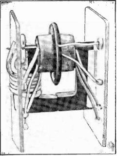
A home-constructed line-output transformer.
