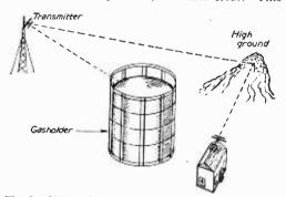
Fig. 3.—If there is an obstacle between the transmitter and the receiving aerial, a reflected signal can sometimes be utilised.
