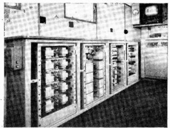
The first mobile Ampex Videotape recording unit to be mounted in a specially designed vehicle is being put into operation by TWW. The view above shows the interior of the van; all equipment is mounted in four low-level racks topped by a working area and in the background is the record monitor and part of the Ampex console.
